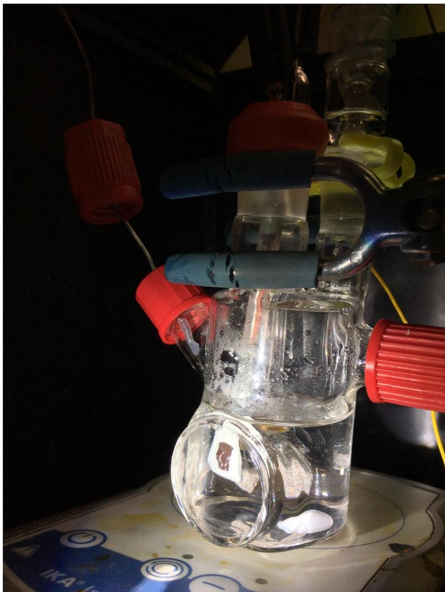
**Supplementary Information Figure S11.** The experimental setup used for the photoelectrochemical measurements which consists of the working electrode, GaP, Ag/AgCl (sat'd KCl) reference electrode, and a Pt mesh counter electrode immersed in 0.1 M H<sub>2</sub>SO<sub>4</sub> (pH 1.1).
