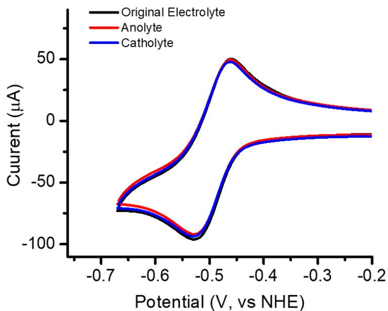
**Figure S3.** Post CV analysis of the  $(\text{SPr})_2\text{V}/(\text{SPr})_2\text{V}^{\cdot-}$  half-cell RFB after the cycling test.
