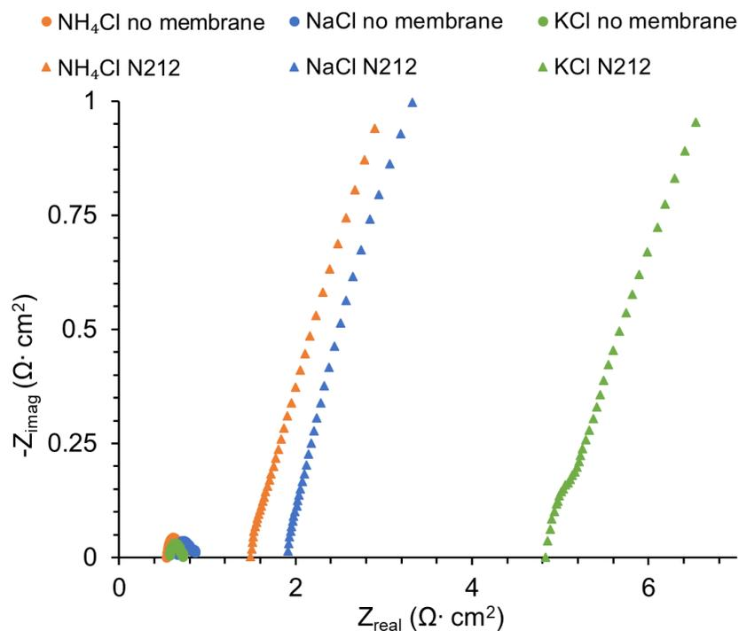
**Figure S5.** EIS curves of flow batteries without membrane and with a Nafion 212 membrane in the presence of 1.0 M NH<sub>4</sub>Cl, 1.0 M NaCl, or 1.0 M KCl as supporting electrolyte.
