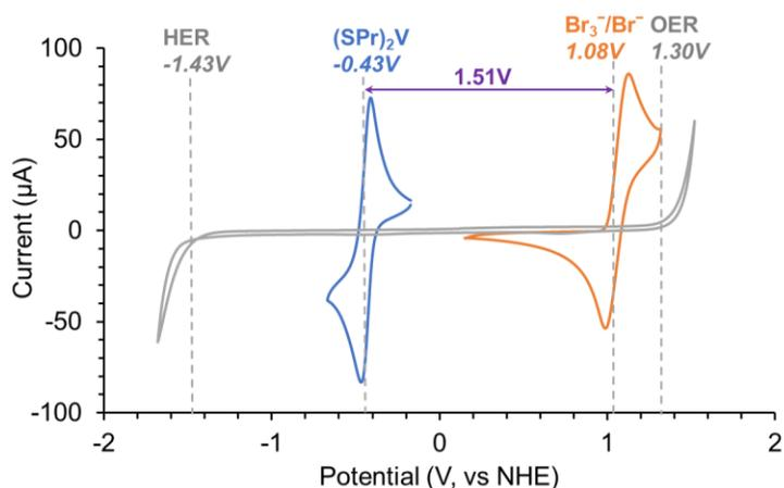
**Figure S1.** The cyclic voltammograms of (SPr)<sub>2</sub>V (-0.43 V) and NH<sub>4</sub>Br (1.08 V) in 0.5M NH<sub>4</sub>Cl aqueous electrolyte. Experiment conditions: 4.0 mM (SPr)<sub>2</sub>V or 50 mM NH<sub>4</sub>Br, 100 mV/s scan rate, glassy carbon working electrode for (SPr)<sub>2</sub>V, Pt working electrode for NH<sub>4</sub>Br, glassy carbon counter electrode, Ag/AgCl reference electrode.
