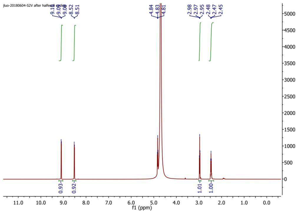
**Figure S4.** Post  $^1\text{H}$ -NMR analysis of the  $(\text{SPr})_2\text{V}/(\text{SPr})_2\text{V}^{\cdot-}$  half-cell RFB after 500 charge/discharge cycles.
