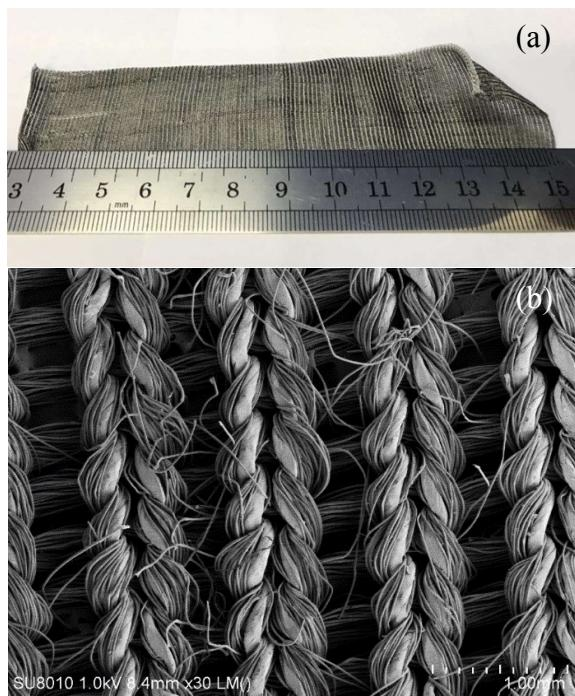
**Figure S6. CNT/PET hybrid knitted fabrics:** (a) Photograph and (b) SEM image.
