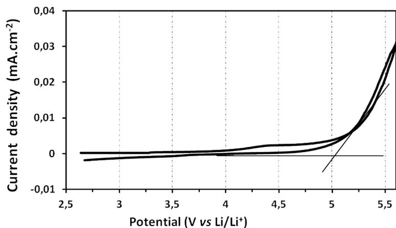
**Fig. S13** Electrochemical stability window of SIN-PC-3 SPE/TEG obtained by CV at a scan rate of  $0.5 \text{ mV s}^{-1}$  at r.t.
