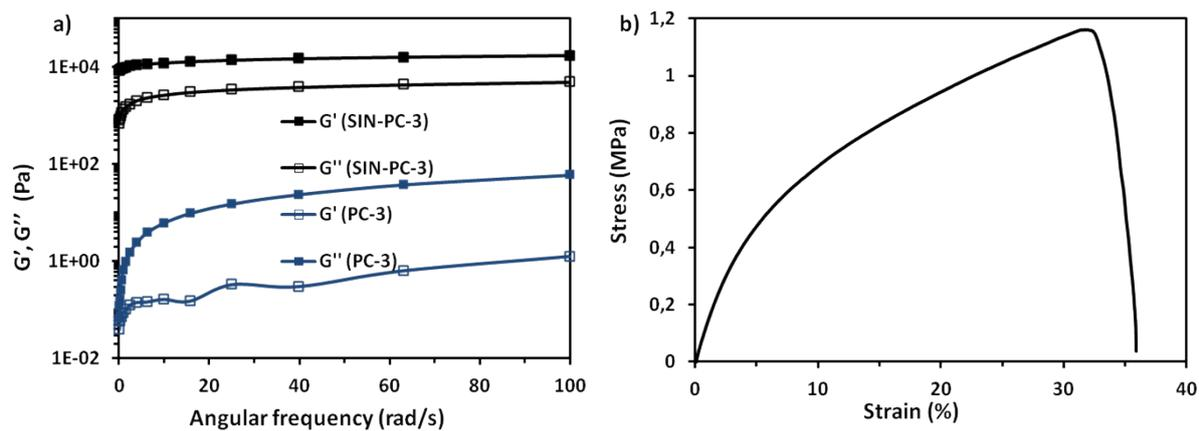
**Fig. S6** (a) Elastic modulus ( $G'$ ) and Storage modulus ( $G''$ ) of PC-3 based SPE and SIN-PC-3 based SPE, (b) stress-strain curves at room temperature of SIN-PC-3 based SPE (deformation rate:  $2 \text{ mm min}^{-1}$ ).
