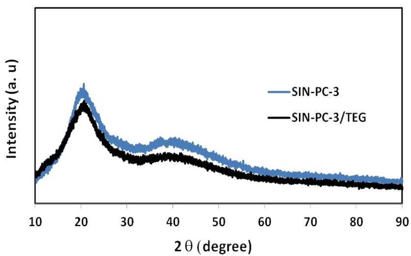
**Fig. S8** XRD spectrum of SIN-PC-3 and SIN-PC-3/TEG membranes.
