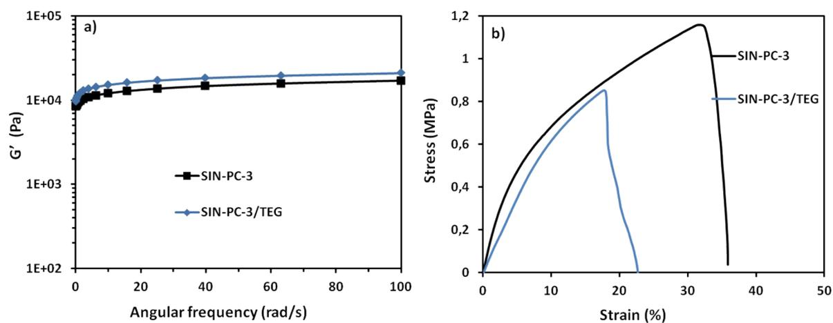
**Fig. S12** (a) Elastic modulus ( $G'$ ) of SIP-PC-3 and SIP-PC-3/TEG (b). stress-strain curves at room temperature of SIN-PC-3 and SIP-PC-3/TEG based SPE (deformation rate: 2 mm min<sup>-1</sup>).
