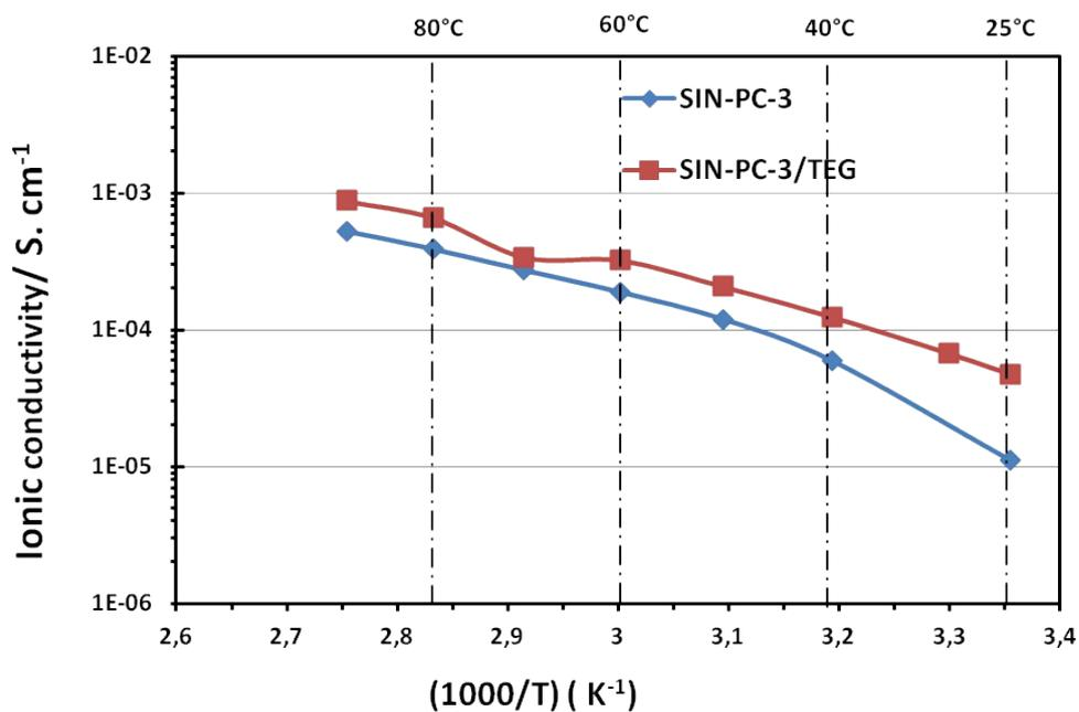
**Fig. S11** Temperature dependence of ionic conductivity of SIN-PC-3 and SIN-PC-3/TEG.
