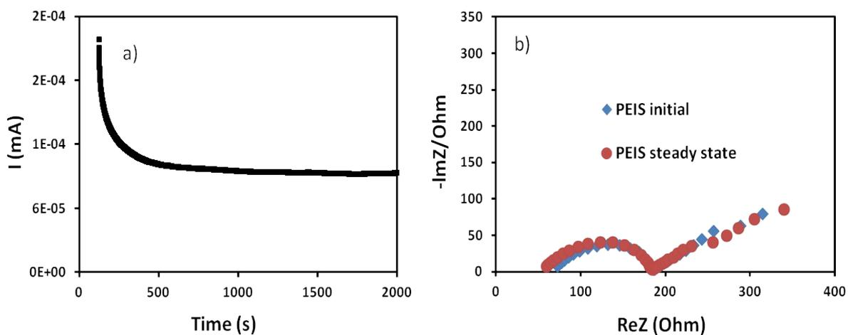
**Fig. S9** (a) The chronoamperometry profile of a symmetric Li/SIN-PC-3/Li battery under a polarization potential of 10 mV, (b) the EIS before and after the polarization.
