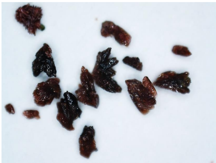
Figure S2. Light microscope image of solvated bulk TMU-61 crystals.
