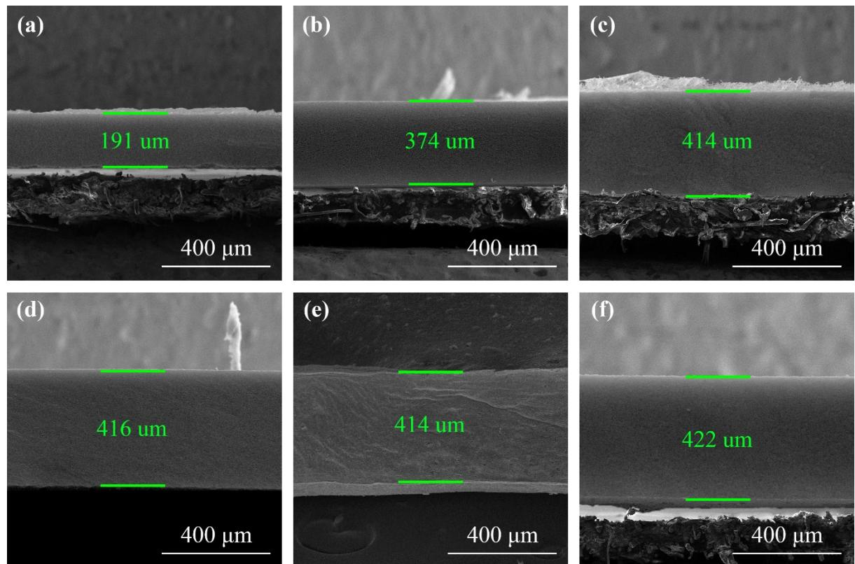
Fig. S6 Cross-sectional SEM images of (a) the pure rGOAM and PEG-rGOAMs with  $Mw_{PEG}$  of (b) 200, (c) 800, (d) 2000, (e) 8000, (f) 20000 Da.
