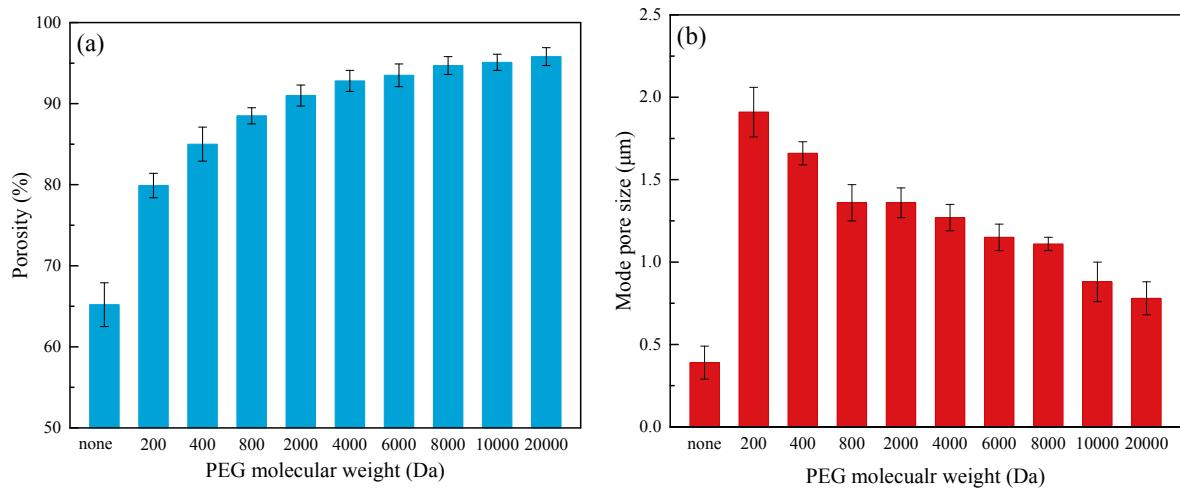
Figure S10. (a) Porosity and (b) mean pore sizes of the pure rGOAMs and PEG-rGOAMs with  $Mw_{PEG}$  from 200 to 20000 Da prepared with large initial GO nanosheets (theoretical average size = 3  $\mu\text{m}$ ).
