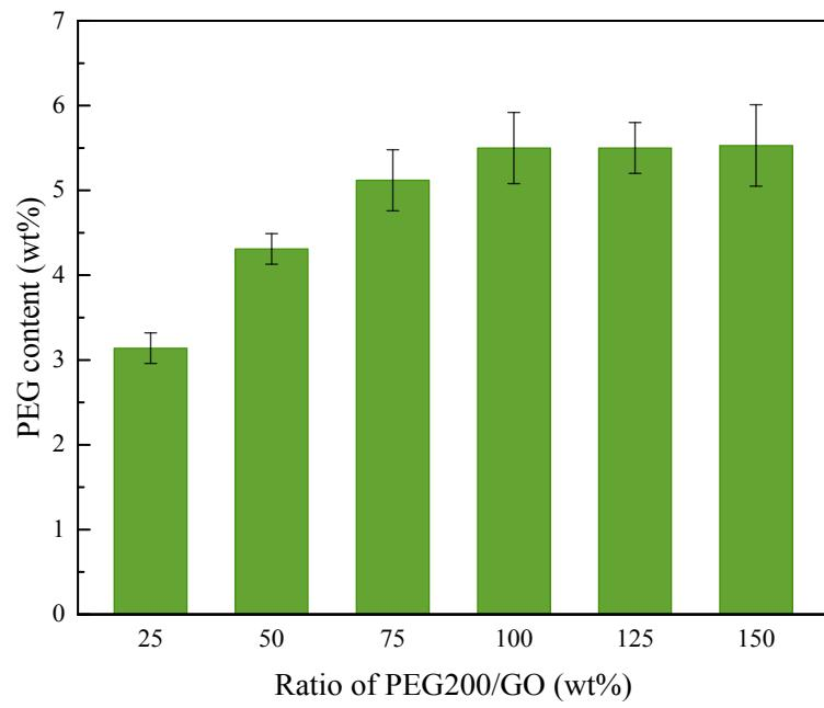
Figure S15. PEG contents in PEG-rGOAMs with the mass ratios of PEG 200/GO from 0wt% to 150wt%.
