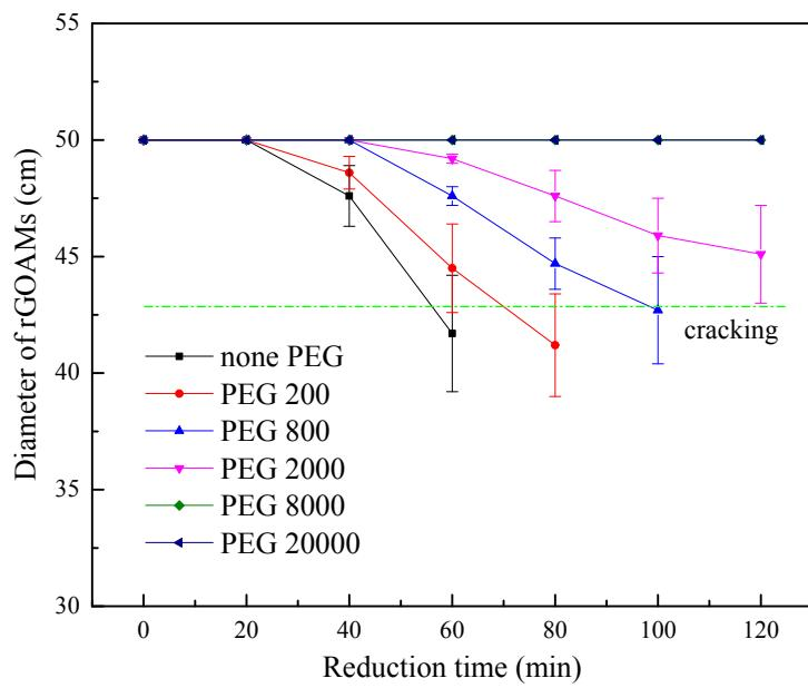
Figure S11. Reduction time-dependent diameter of the pure rGOAM and PEG-rGOAMs with  $Mw_{PEG}$  from 200 to 20000 Da.
