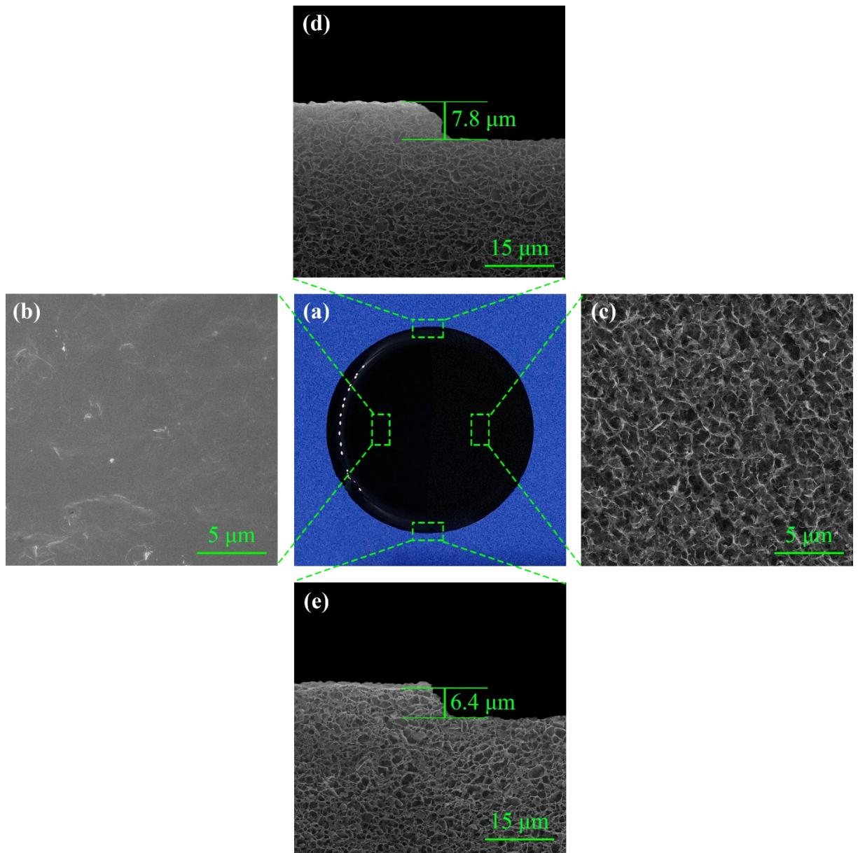
Fig. S7 (a) Photographic image of the virgin PEG-rGOAM ( $Mw_{PEG}$  of 8000) with the right half of the surface treated by metallographic abrasive paper (P2000). Surface morphology of the PEG-rGOAM (b) before and (c) after treatment. (e) and (f) Cross-sectional SEM images of the boundary, showing the thickness of the removed dense surface layer.
