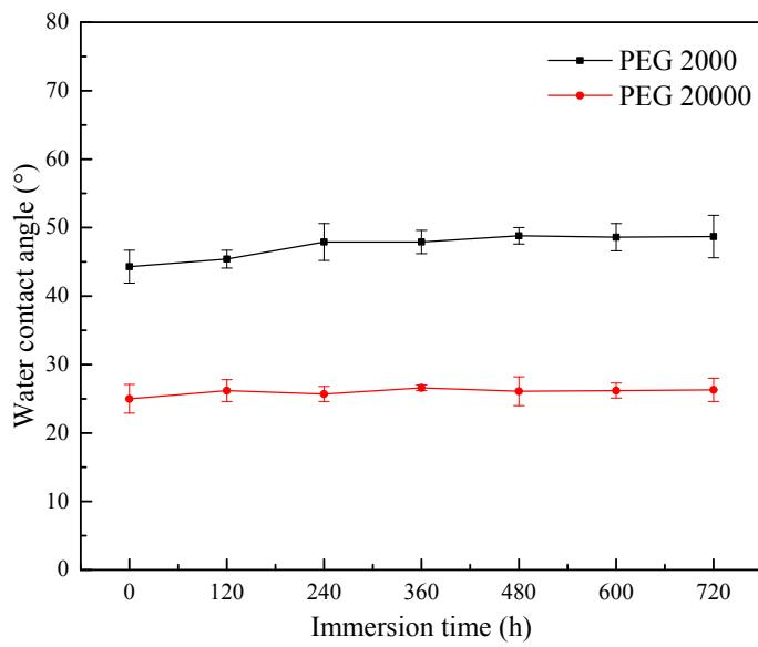
Figure S24. The surface water contact angles of PEG-rGOAMs with  $Mw_{PEG}$  of 2000 and 20000 Da during the immersing test.
