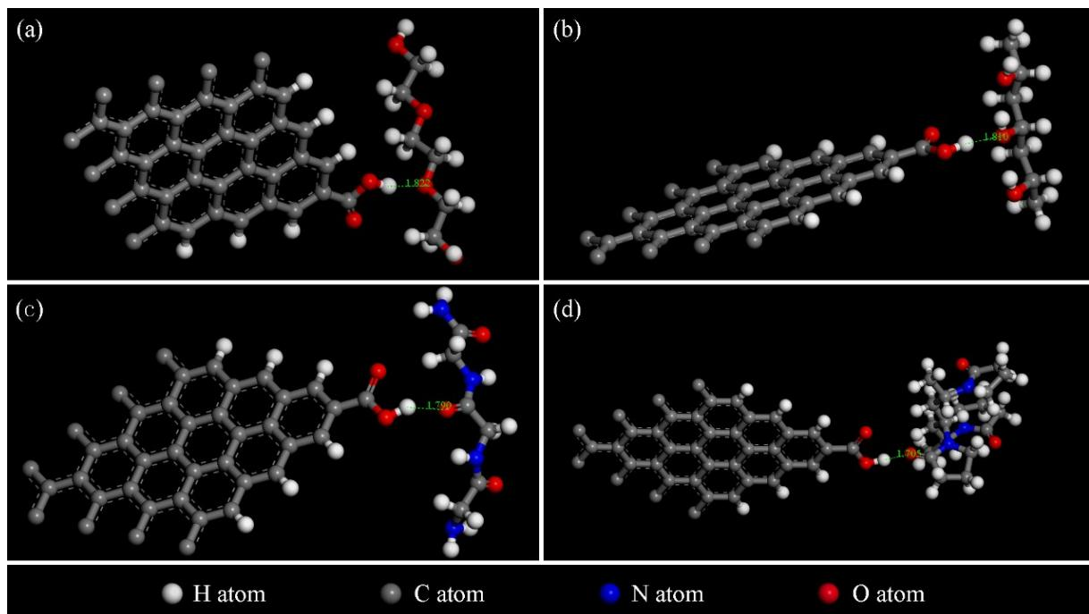
Figure S25. Calculation of the hydrogen bond length of the polymers with benzoic carboxyl groups of rGO nanosheets in the (a) PEG-rGOAM, (b) PVA-rGOAM, (c) polyglycine-rGOAM and (d) PVP-rGOAM by Materials Studio.
