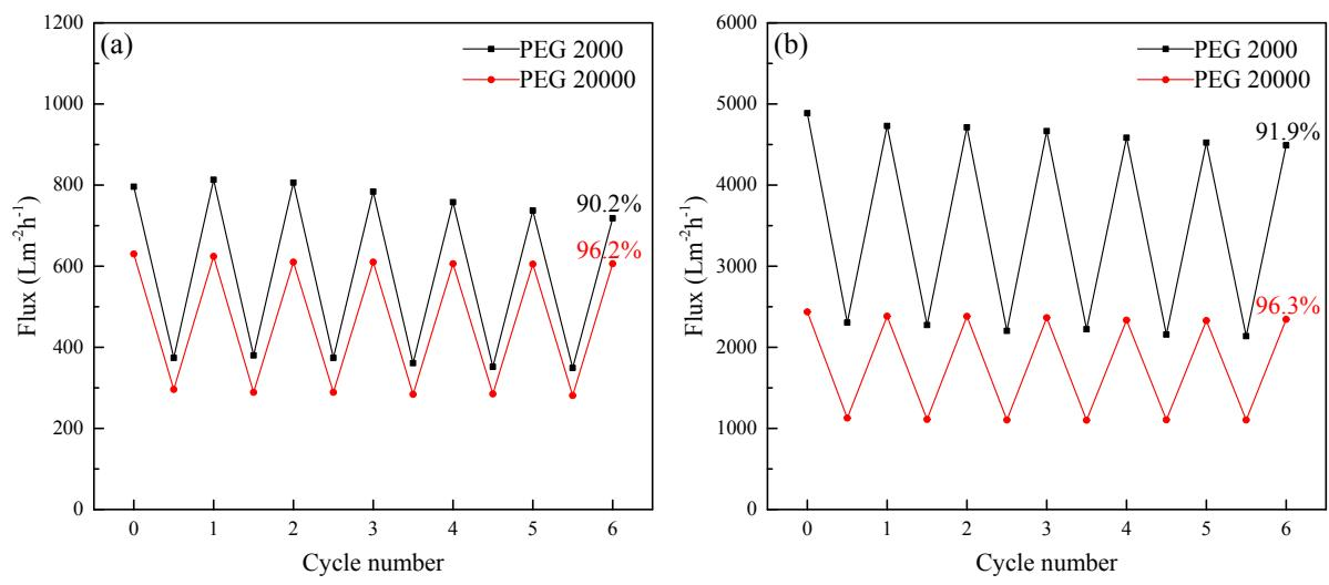
Figure S21. Antifouling performance of PEG-rGOAMs with  $Mw_{PEG}$  of 2000 and 20000 Da in the separation of bump oil-in-water emulsion under the pressure of (a) 0.01 and (b) 0.1 bar.
