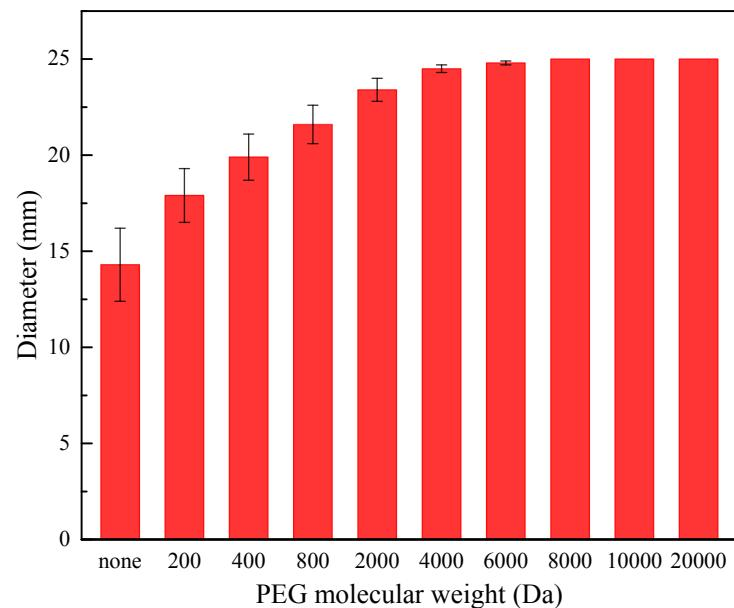
Fig. S4. Diameter of the pure rGOAM and PEG-rGOAMs with  $Mw_{PEG}$  from 200 to 20000 Da prepared in the cylindrical mold with the diameter of 25.0 mm.
