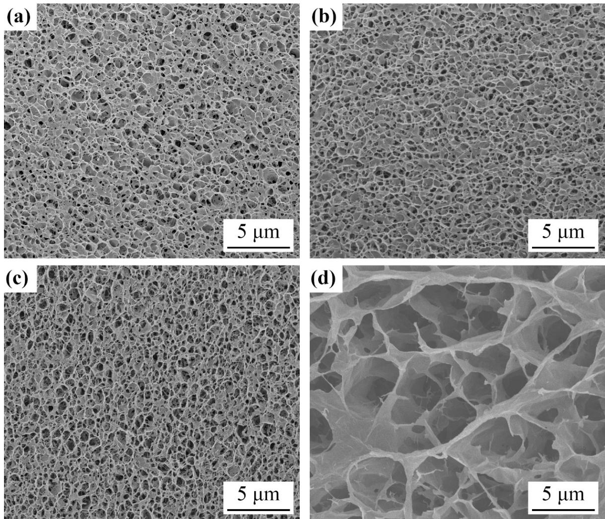
Figure S26. Surface morphology of the (a) PEG-rGOAM, (b) PVA-rGOAM, (c) polyglycine-rGOAM and (d) PVP-rGOAM.
