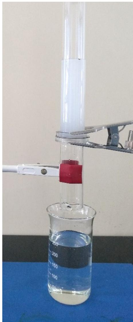
Figure S18. Photo of the PEG-rGOAM with  $Mw_{PEG}$  of 2000 Da utilized in the separation of corn oil-in-water emulsion.
