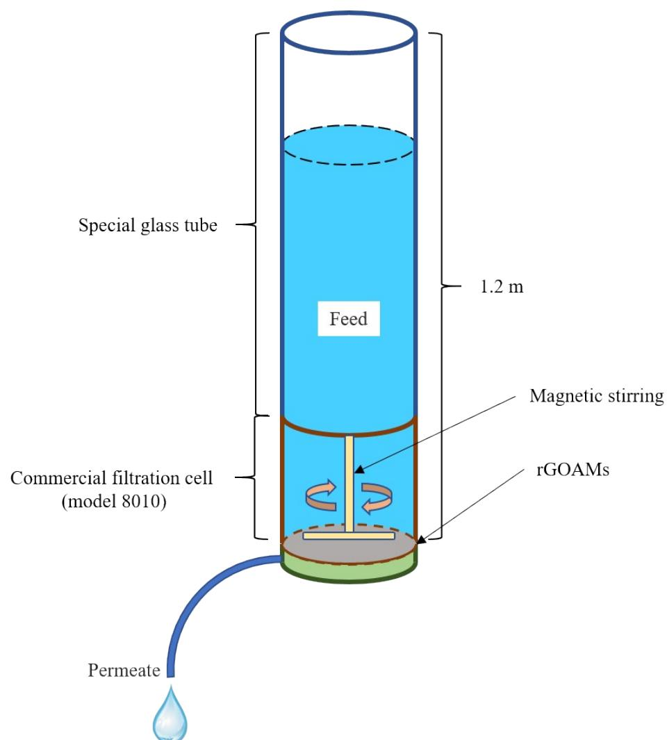
Fig. S1 Schematic illustration of the gravity-driven dead-end stirred cell filtration system.
