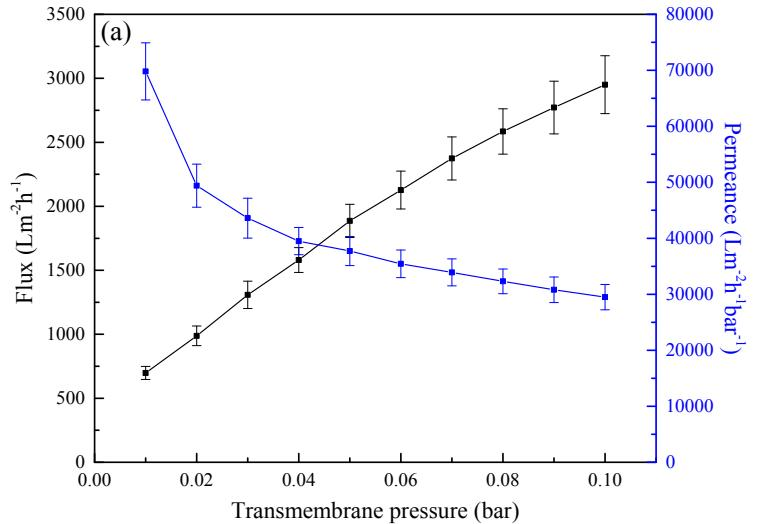
Figure S19. Flux and permeance of PEG-rGOAMs with  $Mw_{PEG}$  of 8000 Da under the transmembrane pressure varied from 0.01 bar to 0.1 bar.
