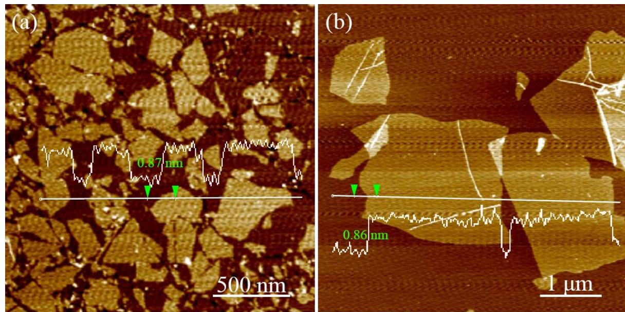
Fig. S2. AFM morphology of initial monolayer GO nanosheets with the theoretical average size of (a) 300 nm and (b) 3  $\mu$ m.
