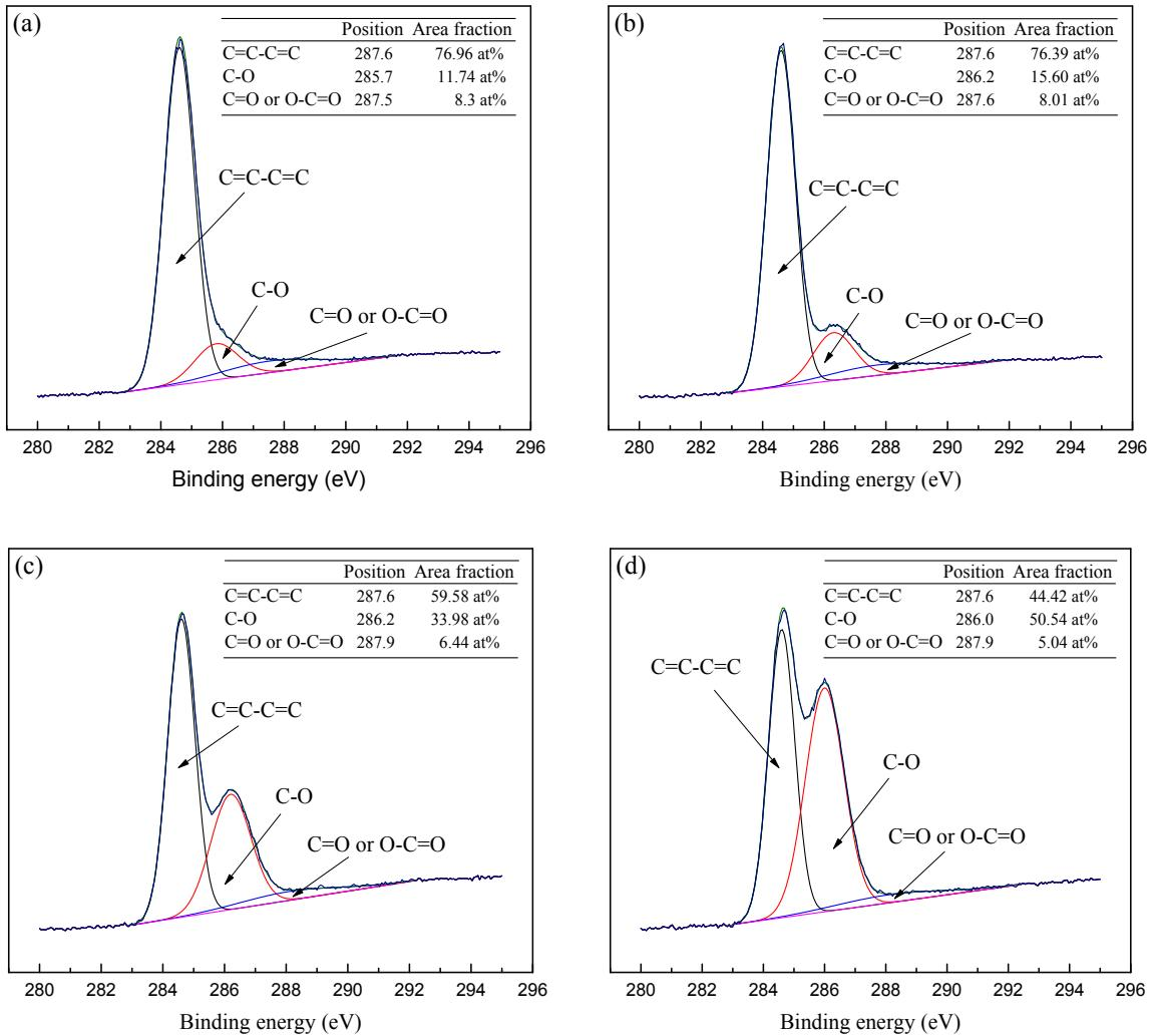
Figure S16. XPS C1s core level spectra of (a) the pure rGOAMs and PEG-rGOAMs with  $Mw_{PEG}$  of (b) 200, (c) 2000 and (d) 20000 Da.
