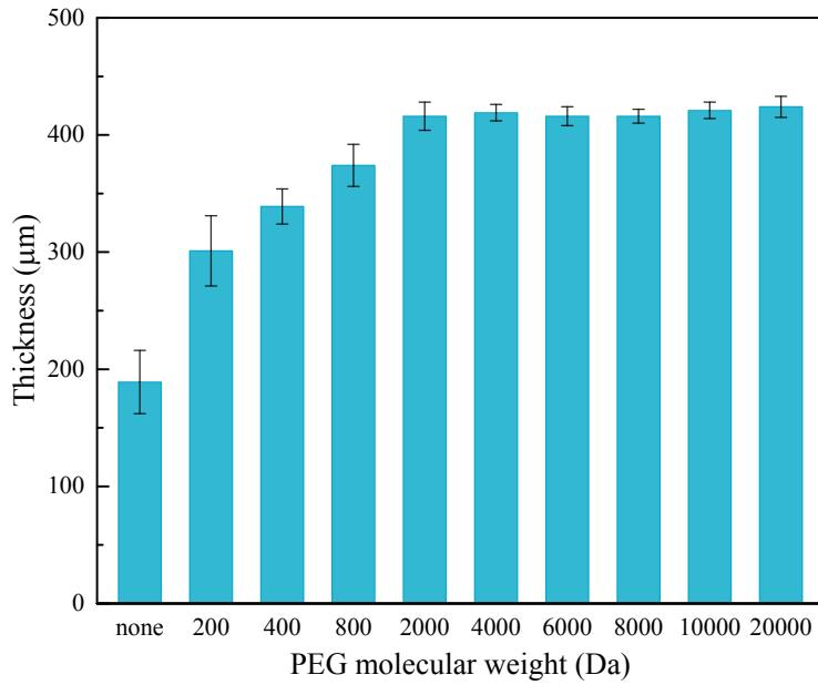
Fig. S5. Thickness of the pure rGOAM and PEG-rGOAMs with  $Mw_{PEG}$  from 200 to 20000 Da prepared in the cylindrical mold with the diameter of 50.0 mm.
