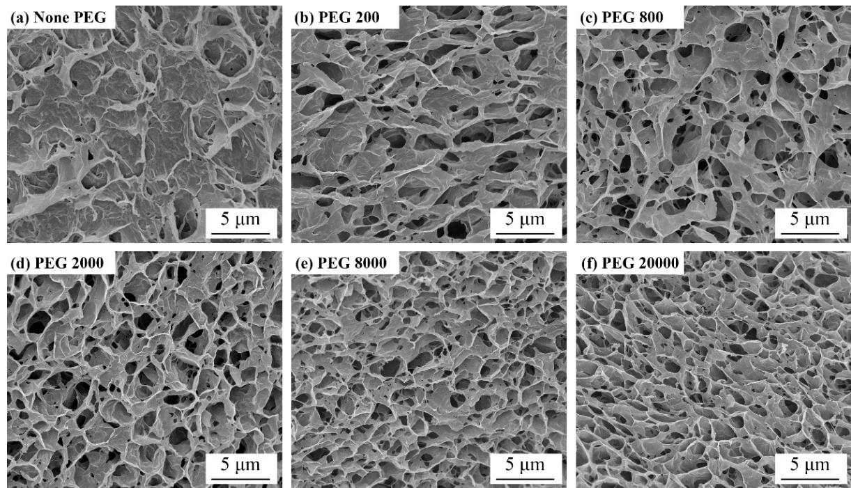
Figure S9. Surface morphology of the pure rGOAM and PEG-rGOAMs with  $Mw_{PEG}$  from 200 to 20000 Da prepared with large initial GO nanosheets (theoretical average size = 3  $\mu\text{m}$ ).
