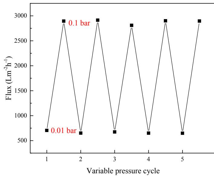
Figure S22. Operational stability of the PEG-rGOAM with  $M_{w,PEG}$  of 8000 Da in the variable pressure cycling test.
