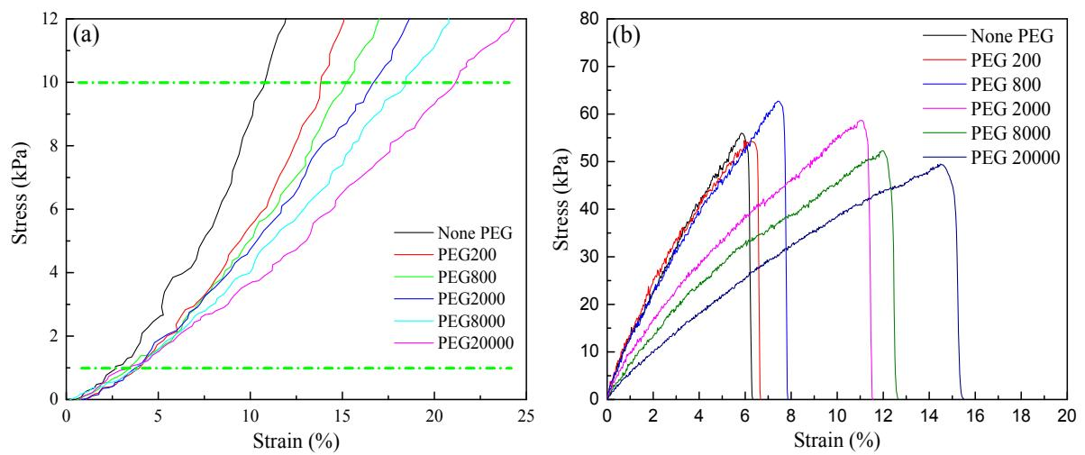
Figure S17. Stress-strain curves of the pure rGOAM and PEG-rGOAMs with  $Mw_{PEG}$  from 200 to 20000 Da in (a) the compressing test and (b) the stretching test.
