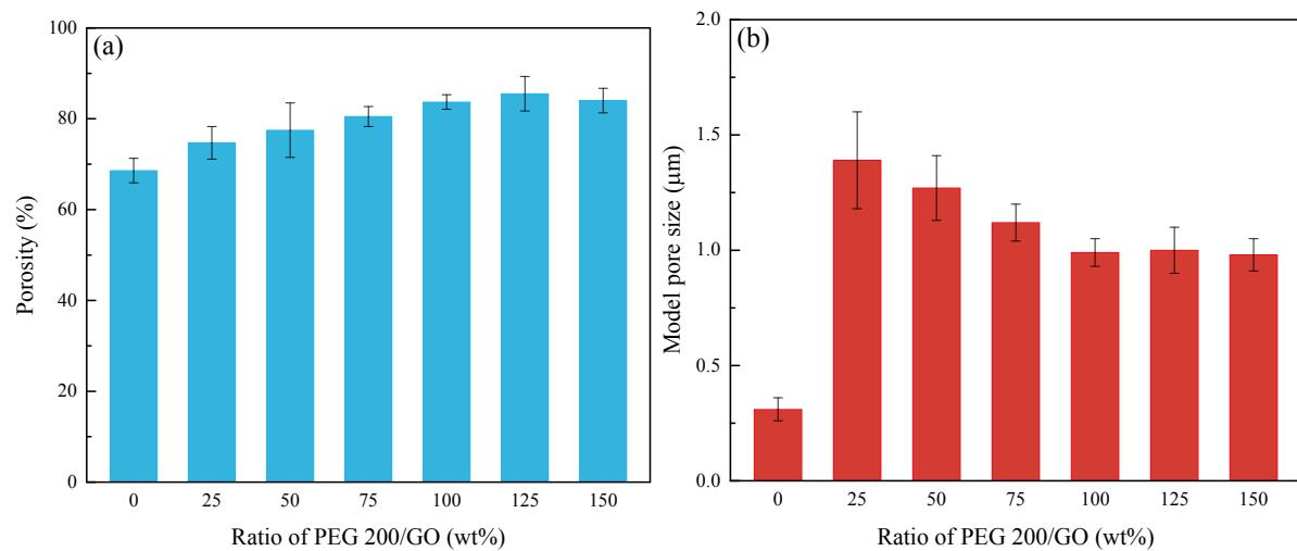
Figure S14. (a) Porosity and (b) mean pore sizes of the pure rGOAM and PEG-rGOAMs with the mass ratios of PEG 200/GO from 25 wt% to 150 wt%.
