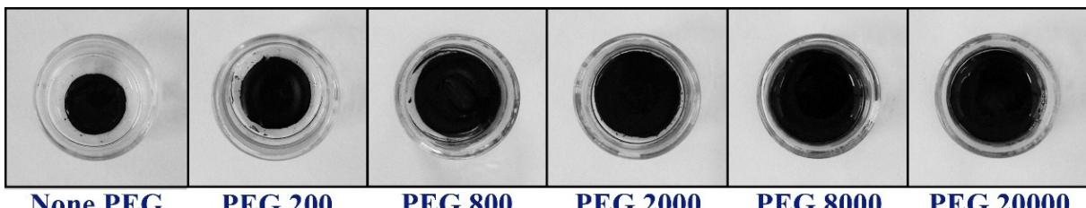
Fig. S3. Macroscopic profiles of the pure rGOAM and PEG-rGOAMs with  $Mw_{PEG}$  from 200 to 20000 Da prepared in cylindrical molds with the diameter of 2.5.
