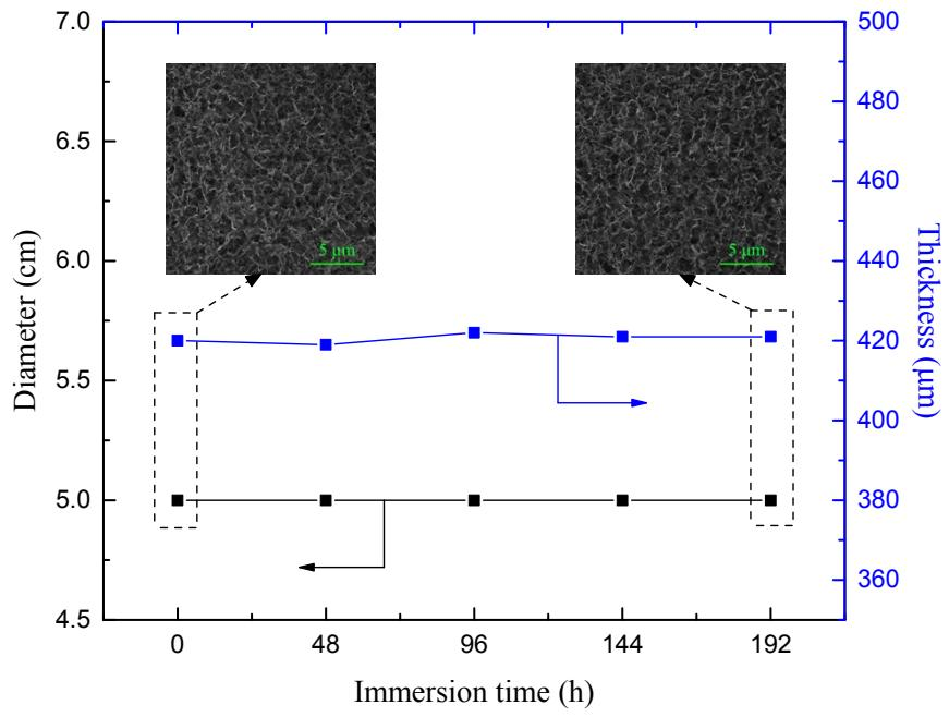
Fig. S23. The morphology of the PEG-rGOAM with  $Mw_{PEG}$  of 2000 during the long-term immersing test.
