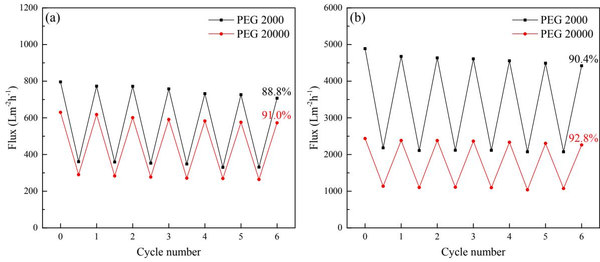
Figure S20. Antifouling performance of PEG-rGOAMs with  $Mw_{PEG}$  of 2000 and 20000 Da in the separation of corn oil-in-water emulsion under the pressure of (a) 0.01 and (b) 0.1 bar.
