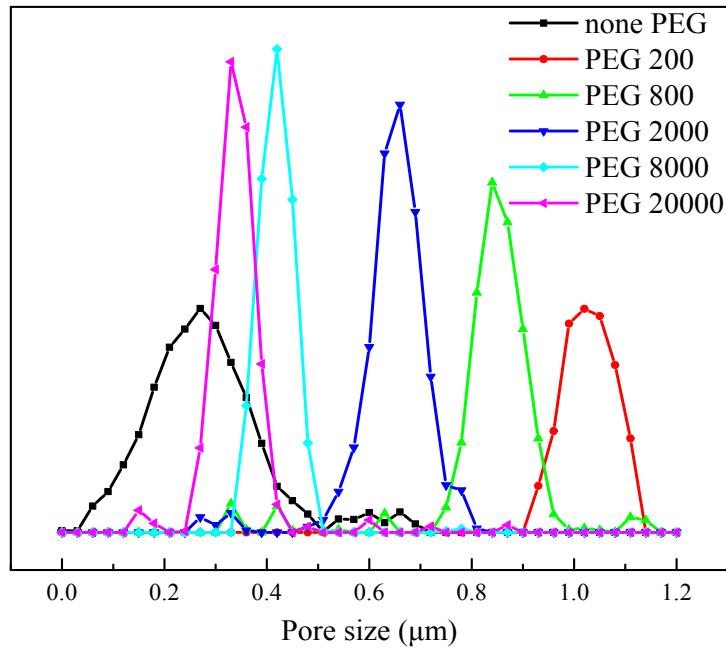
Fig. S8. Pore size distribution of the pure rGOAM and PEG-rGOAMs with  $Mw_{PEG}$  from 200 to 20000 Da acquired by the bubble-pressure method.
