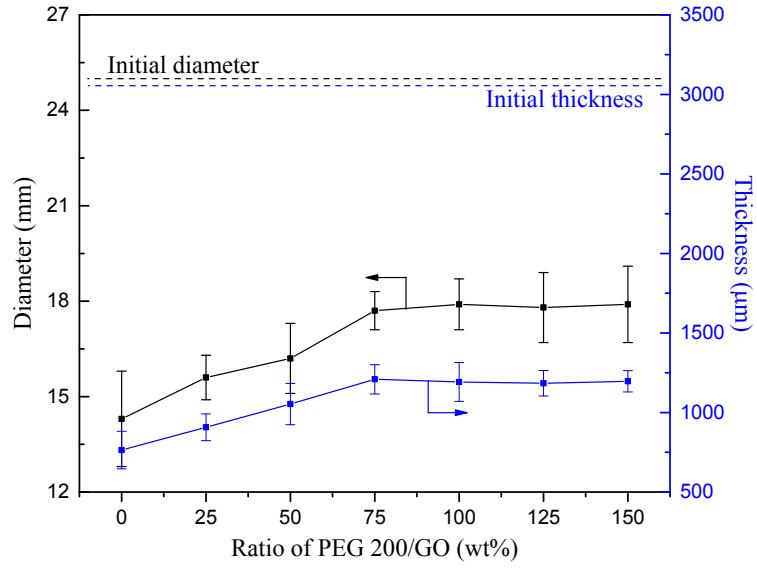
Figure S12. Diameter and thickness of the pure rGOAM and PEG-rGOAMs with the mass ratios of PEG 200/GO from 25wt% to 150wt%.
