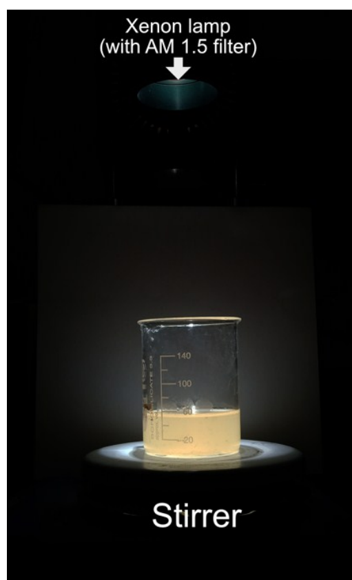
Figure S2. Setup of the practical application study under the simulated solar irradiation. No temperature controller is provided for the reaction.
