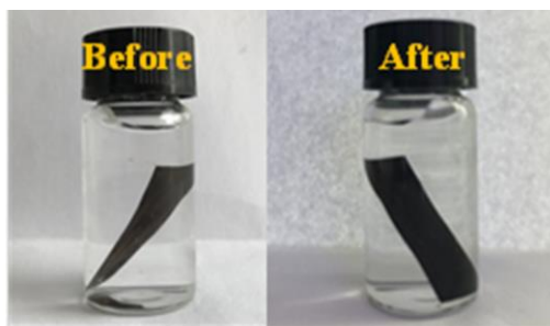
Figure S5. digital photos of the 260-PPy/CNTP electrode before and after 30 min ultrasonic treatment.
