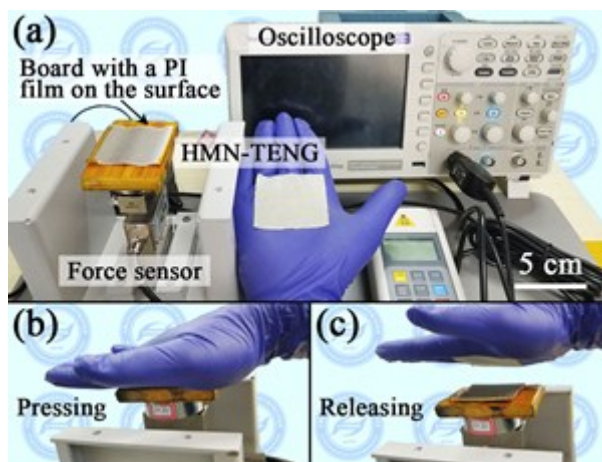
Fig. S11. Photographs of (a) the test setup platform, (b) pressing state and (c) releasing state during hand patting. In the experiment, a PI film was pasted on the surface of the board for the sake of reducing electrostatic charge generated between the top surface of the board and the bottom surface of Part A of the HMN-TENG.
