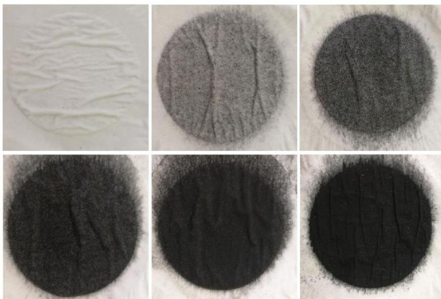
**Fig. S2** Air-laid paper (a) without and with (b) 0.004 kg·m<sup>-2</sup>, (c) 0.016 kg·m<sup>-2</sup>, (d) 0.040 kg·m<sup>-2</sup>, (e) 0.080 kg·m<sup>-2</sup>, (f) 0.160 kg·m<sup>-2</sup> MoS<sub>2</sub> deposition.
