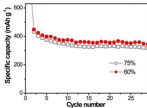
Fig.S12 Cycling performance of the hollow  $\text{Sb}_2\text{Se}_3@\text{C}$  microtube at  $100 \text{ mA g}^{-1}$  with active material content of 75 % (with 15% of conductive agent and 10% of binder). The red symbol imply the sample with 60% of active materials in agreement with
