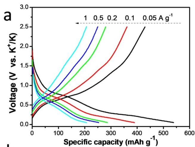
Fig. S13. (a) Rate charge/discharge curves of the hollow  $\text{Sb}_2\text{Se}_3@\text{C}$  microtubes at different current densities. (b) Comparison of the potassium storage performances of the hollow  $\text{Sb}_2\text{Se}_3@\text{C}$  microtubes and the previously reported selenide/sulfide-based anode materials in PIBs.
