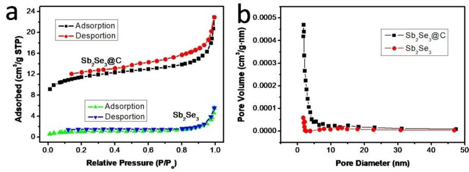
Fig.S14. (a) N<sub>2</sub> adsorbed curves and (b) pore volume of the hollow Sb<sub>2</sub>Se<sub>3</sub>@C microtubes and pure Sb<sub>2</sub>Se<sub>3</sub> microrod electrode.
