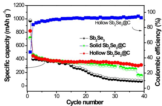
Fig. S11. Comparison of the galvanostatic cycling performance at a current density of  $100 \text{ mA g}^{-1}$ .
