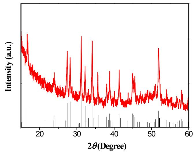
Fig. S4. XRD pattern of the solid Sb<sub>2</sub>Se<sub>3</sub>@C submicrorods.
