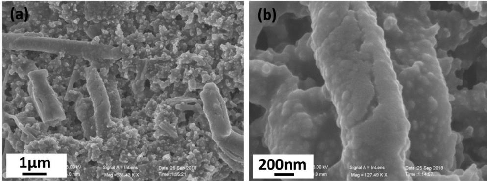
Fig.S15. SEM images of (a-b) the solid  $\text{Sb}_2\text{Se}_3@C$  submicrorod electrode.
