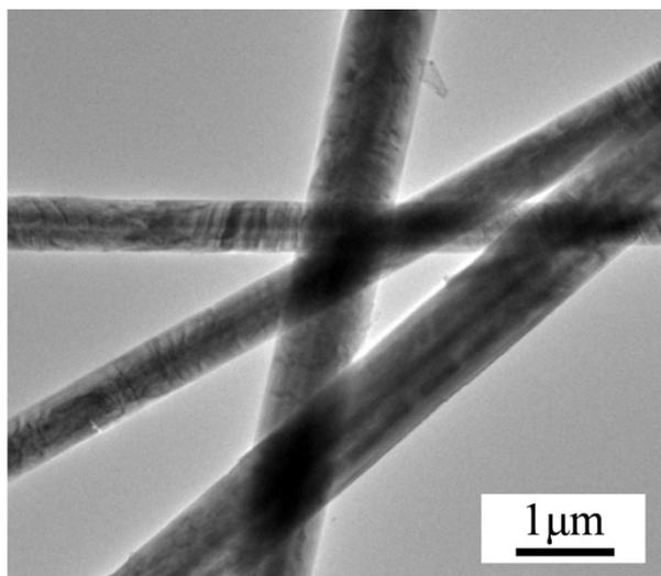
Fig.S2. The TEM image of the  $\text{Sb}_2\text{O}_3$  precursor.
