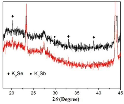
Fig. S9. The XRD pattern of the hollow Sb<sub>2</sub>Se<sub>3</sub>@C microtube electrode discharged at 0.05 V vs K<sup>+</sup>/K.
