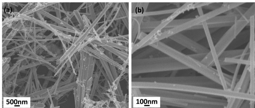
Fig. S5. (a-b) SEM images of solid  $\text{Sb}_2\text{Se}_3$  submicrorods obtained by a hydrothermal method..
