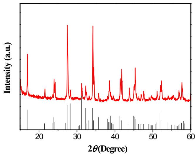
Fig. S6. XRD pattern of the solid  $\text{Sb}_2\text{Se}_3$  submicrorods obtained by a hydrothermal method.
