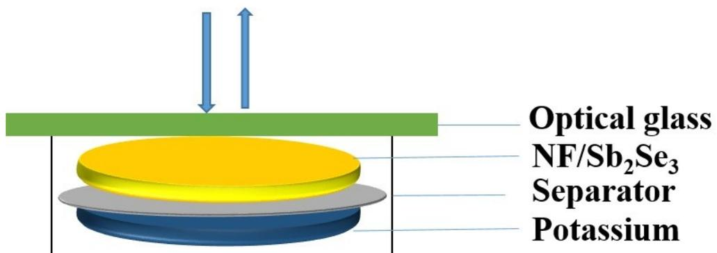
Fig. S8. Schematic of Raman cell setup (NF=Ni foil).
