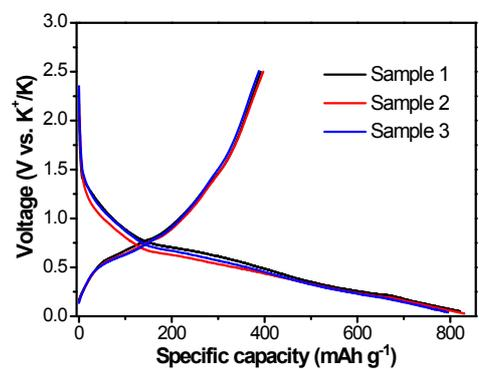
Fig.S10 The first charge/discharge curves of the hollow Sb<sub>2</sub>Se<sub>3</sub>@C microtube at 100 mA g<sup>-1</sup>. These curves are obtained from three cells at similar testing condition.
