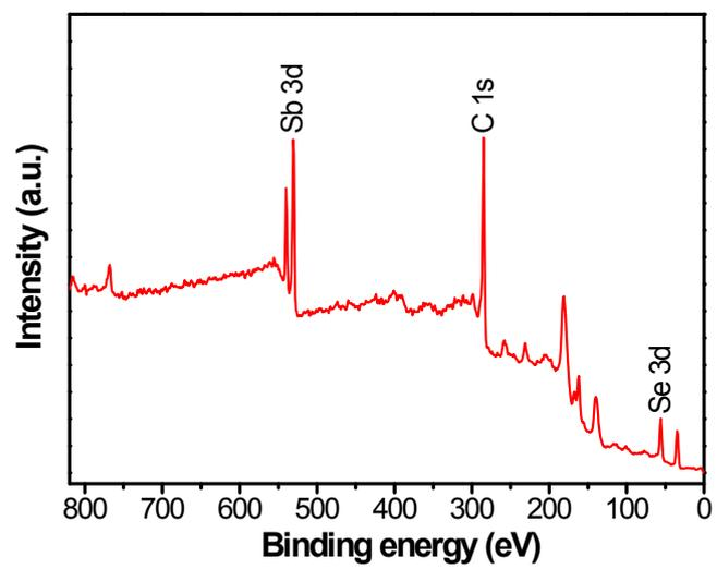
Fig. S7. The XPS of the hollow  $\text{Sb}_2\text{Se}_3$ @C submicrotubes.
