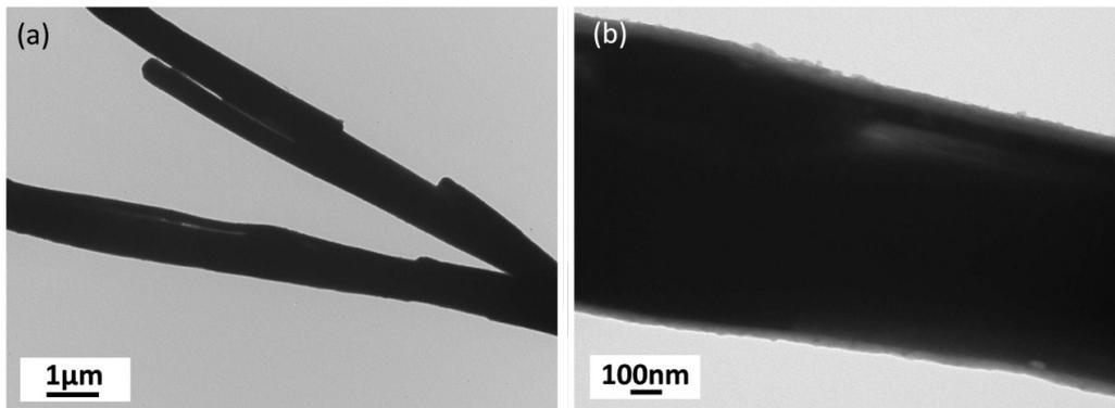
Fig. S3. (a-b) TEM images of the solid  $\text{Sb}_2\text{Se}_3@\text{C}$  submicrorods.
