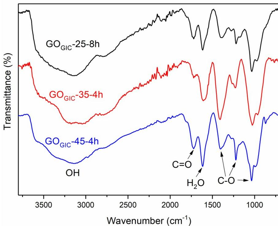
Figure S5. ATR-FTIR spectra for  $\text{GO}_{\text{GIC}}$  films which indicated the presence of C=O (the peak at  $\sim 1723 \text{ cm}^{-1}$ ), C-O (at  $1400$  and  $1225 \text{ cm}^{-1}$ ) and -OH ( $3700\text{-}2700 \text{ cm}^{-1}$ ) in GO samples.<sup>1,2</sup>
