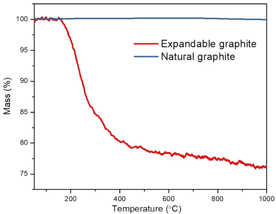
Figure S2. TGA curves of expandable graphite and natural graphite heated from 50 to 1000 °C at the rate of 5 K/min under pure argon atmosphere.
