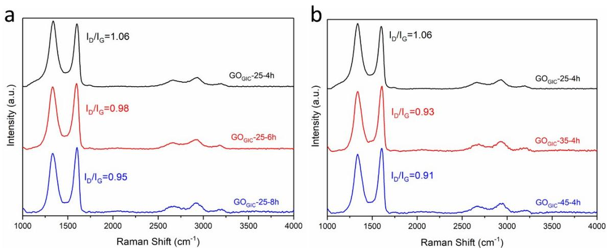
Figure S3. The Raman spectra of GO<sub>GIC</sub> (a) at the temperature of 25 °C for different time, and (b) at different temperature for 4 h.
