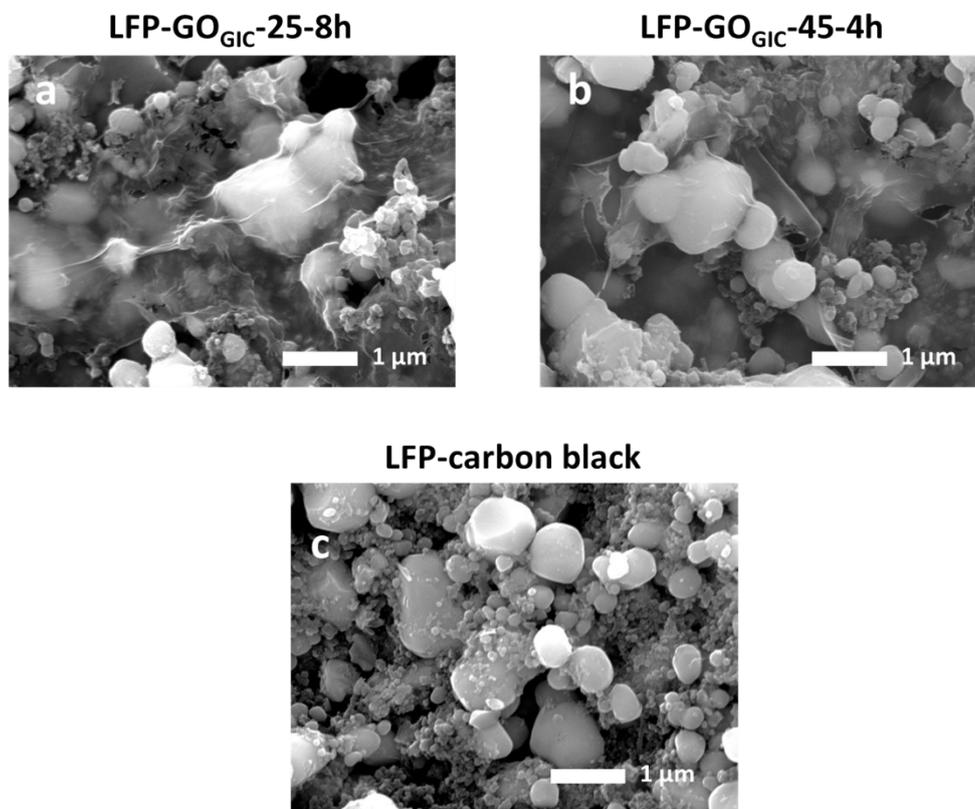
Figure S6. SEM images for  $\text{GO}_{\text{GIC}}$  modified LFP cathodes and unmodified LFP cathode.
