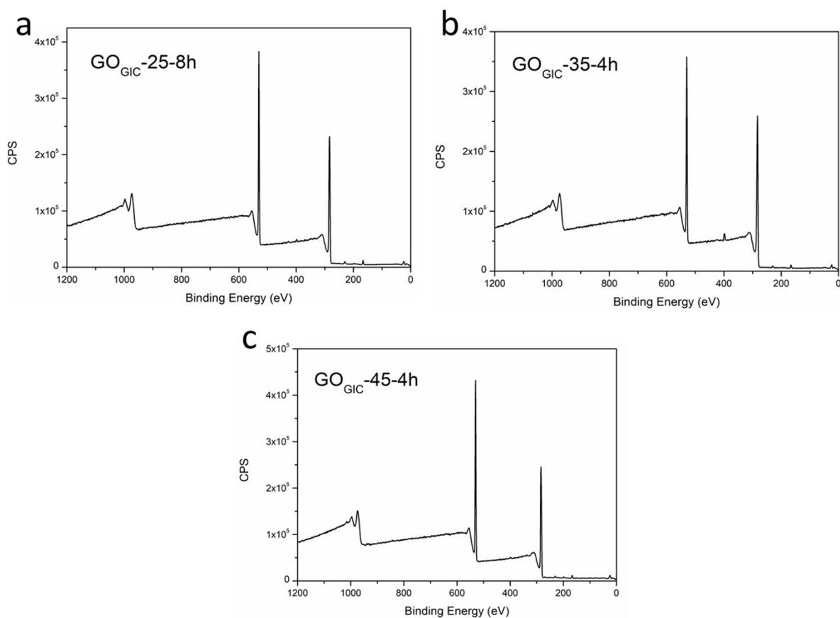
Figure S4. XPS survey spectra for different GO<sub>GIC</sub> samples. The C/O ratios for GO<sub>GIC</sub>-25-8h, GO<sub>GIC</sub>-35-4h and GO<sub>GIC</sub>-45-4h were 2.68, 3.05 and 2.41, respectively.
