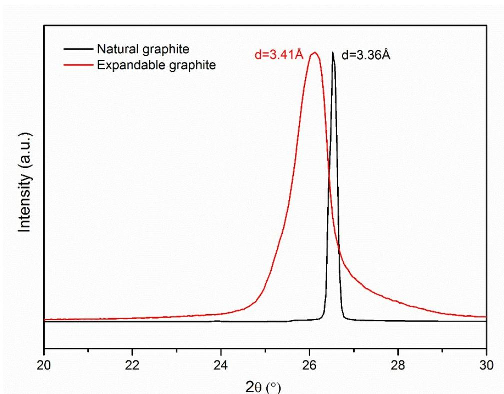
Figure S1. The XRD curves for expandable graphite and natural graphite.
