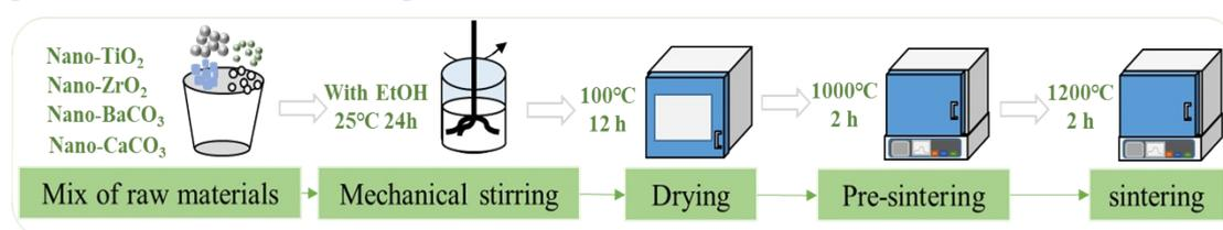
**Fig. S1.** Synthesis procedure schematic of BCZT-SS particles.
