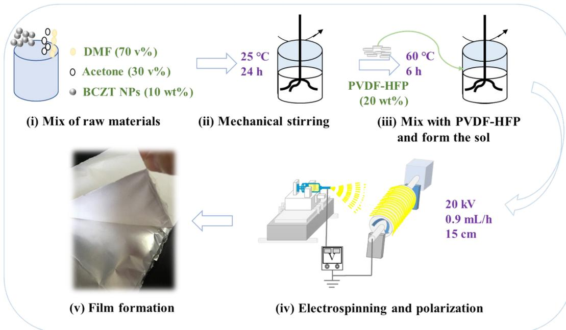
**Fig. S4.** Synthesis procedure schematic of BP-based NF.
