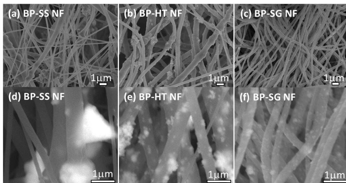
**Fig. S5.** SEM images of BP-based NF under (a-c) ETD Mode and (d-f) BSED Mode.
