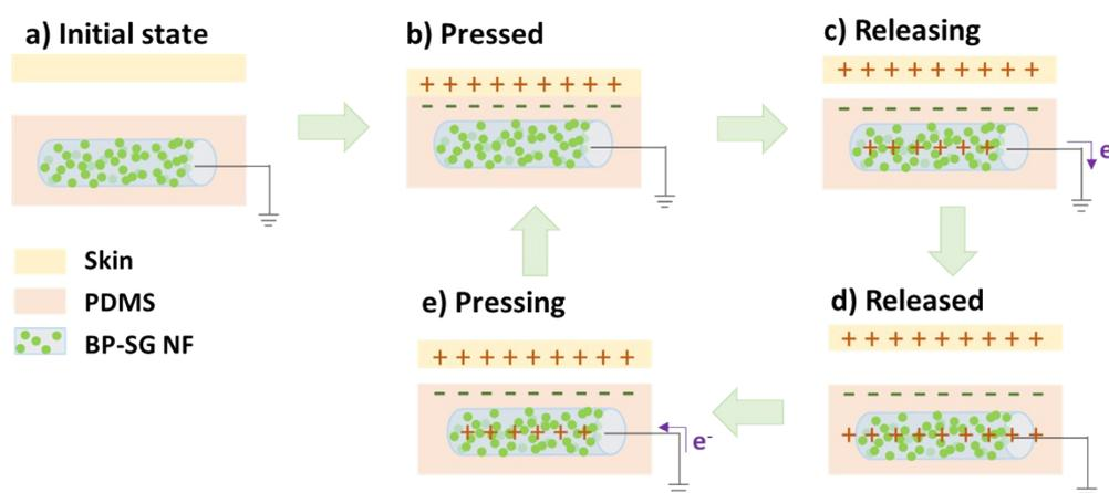
**Fig. S7.** Working mechanism of BP-SG S-TPNG.
