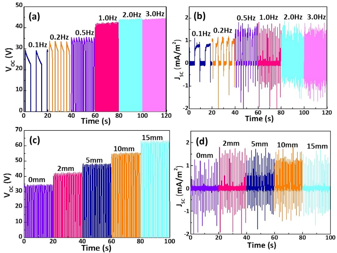
**Fig. S6.** Effect of (a, b) contact frequency and (c, d) gap distance between on the open-circuit voltage ( $V_{oc}$ ) and short-circuit current ( $J_{sc}$ ) of BP-SG PTNG.
