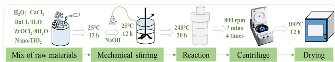
**Fig. S2.** Synthesis procedure schematic of BCZT-HT particles.
