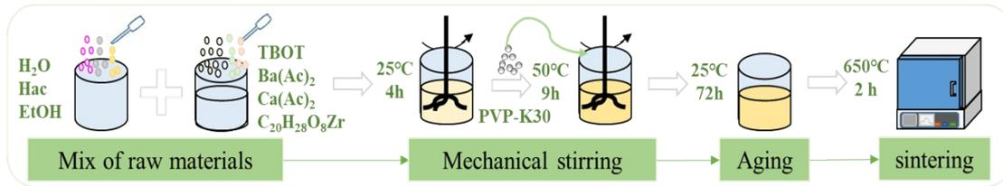
**Fig. S3.** Synthesis procedure schematic of BCZT-SG particles.
