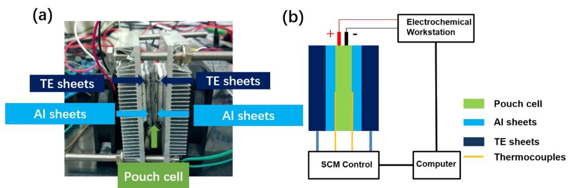
**Figure S6** The home-made thermal cycler for temperature measurement and thermal cycling. (a) A camera image of the setup, (b) The structure of the system.
