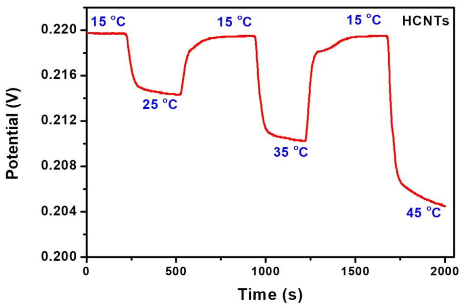
**Figure S7.** The real time measurement of temperature coefficient of HCNTs
