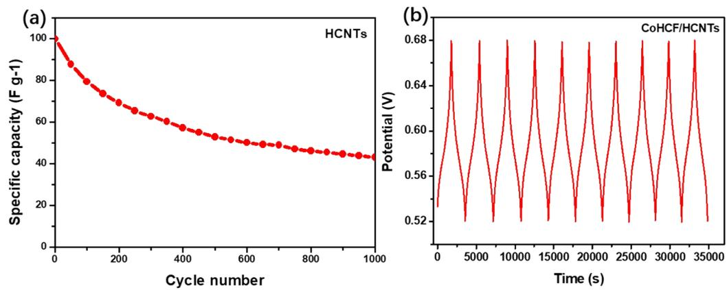
**Figure S5** Cycling stability of (a) HCNTs and (b) CoHCF/HCNTs
