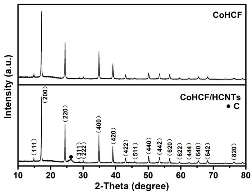
**Figure S2.** XRD patterns of as-prepared CoHCF and CoHCF/HCNTs composite.
