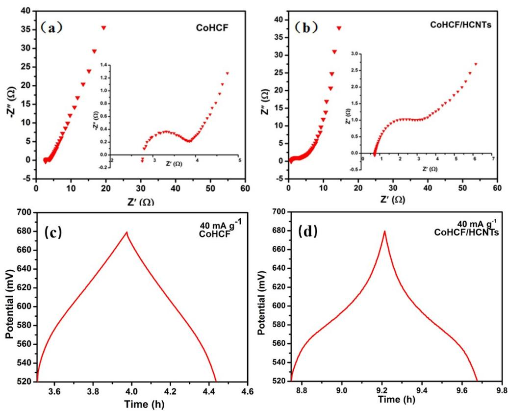
**Figure S4.** Nyquist spectra of (a) CoHCF electrode and (b) CoHCF/HCNTs electrode (inset shows the magnified), GCD curves of the (c) pure CoHCF and (d) CoHCF/HCNTs electrode.
