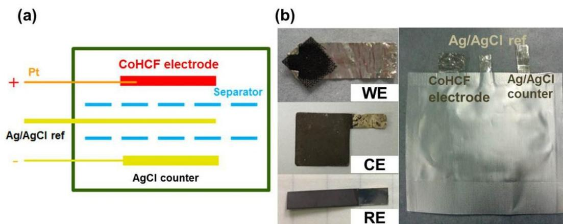
**Figure S3.** The pouch cell configuration used in electrochemical measurements. (a) Schematic of the pouch cell, (b) Optical images of TREC electrodes and fabricated cell.
