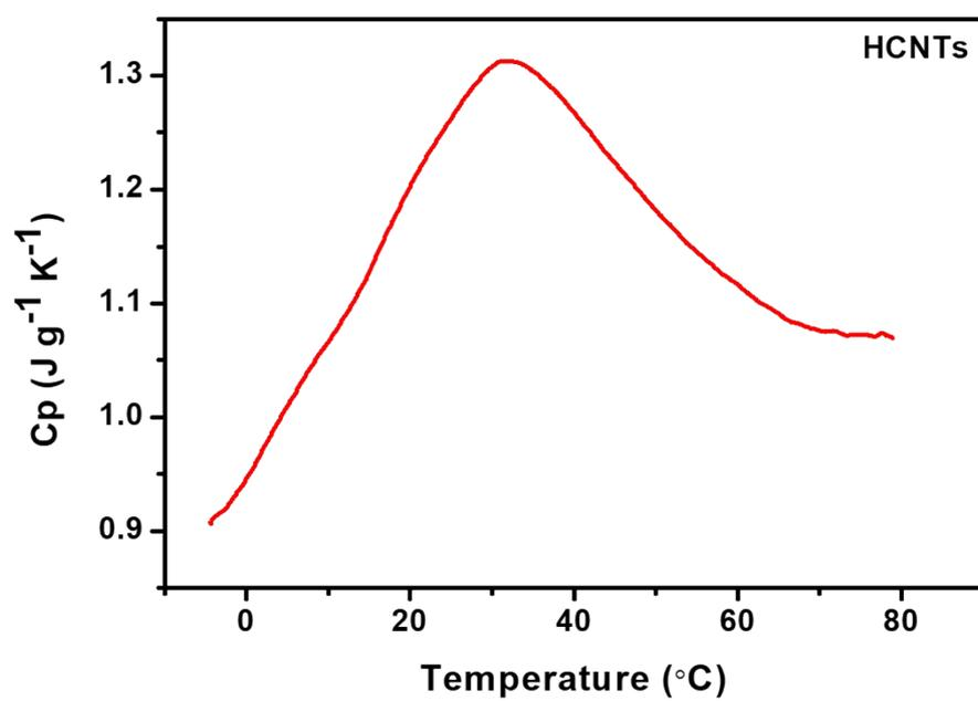
**Figure S9.** The specific heat of pure HCNTs
