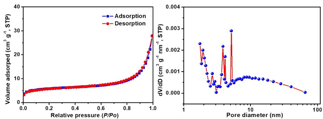
**Figure S8** N<sub>2</sub> adsorption/desorption isotherms of HCNTs and the corresponding pore size distributions.
