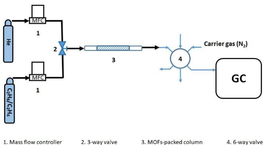
**Fig. S2** Schematic illustration of the self-assembly apparatus for the breakthrough experiments
