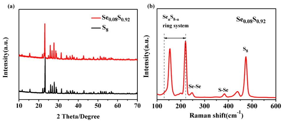
**Fig. S1** XRD pattern (a) and Raman spectra (b) of  $\text{Se}_{0.08}\text{S}_{0.92}$ .
