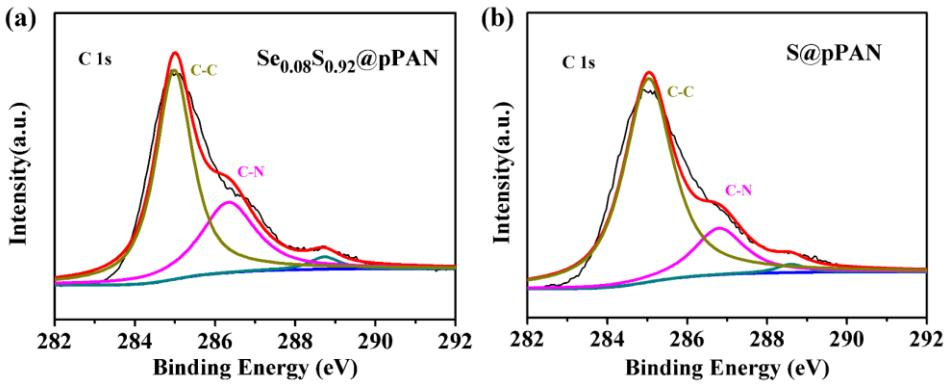
**Fig. S4** XPS spectra of C 1s for  $\text{Se}_{0.08}\text{S}_{0.92}@\text{pPAN}$  (a) and S@pPAN (b).
