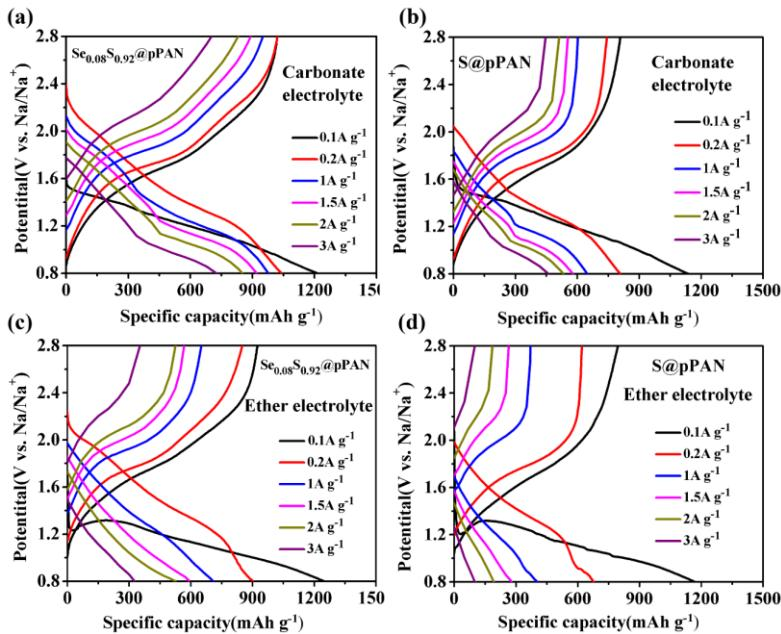
**Fig. S5** Voltage profiles at various current densities from  $0.1 \text{ A g}^{-1}$  to  $3 \text{ A g}^{-1}$  of  $\text{Se}_{0.08}\text{S}_{0.92}@\text{pPAN}$  in carbonate electrolyte (a) and in ether electrolyte (c). Voltage profiles at various current densities from  $0.1 \text{ A g}^{-1}$  to  $3 \text{ A g}^{-1}$  of S@pPAN in carbonate electrolyte (b) and in ether electrolyte (d).
