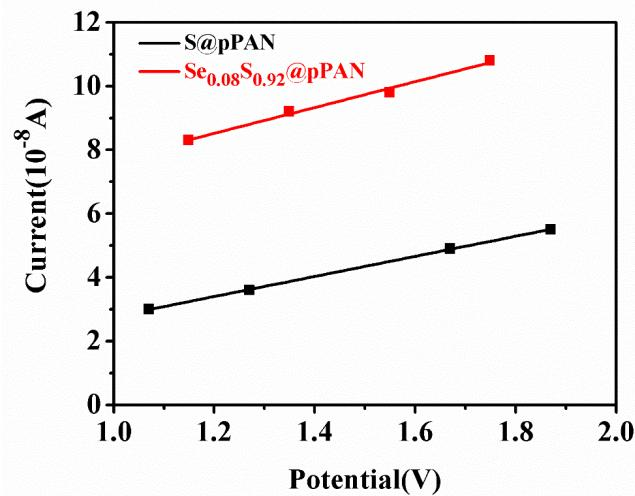
**Fig. S8** Equilibrium current of the  $\text{S@pPAN}$  and  $\text{Se}_{0.08}\text{S}_{0.92}\text{@pPAN}$  at different set voltages.
