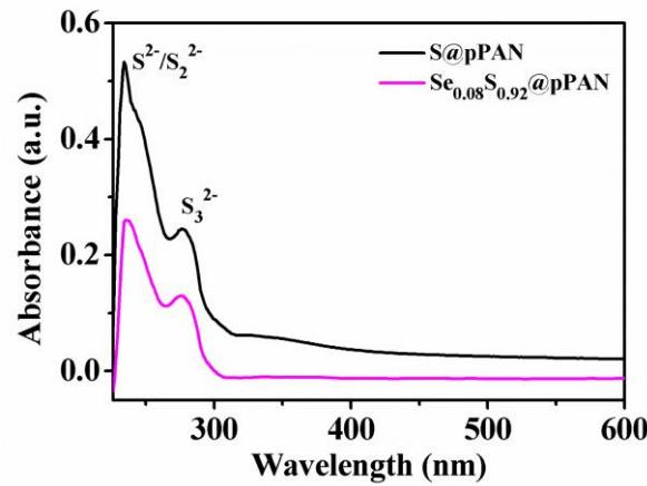
**Fig. S13** UV-vis spectra of the  $\text{S}@\text{pPAN}$  and  $\text{Se}_{0.08}\text{S}_{0.92}@\text{pPAN}$  cathodes solutions cycled in ether electrolyte.
