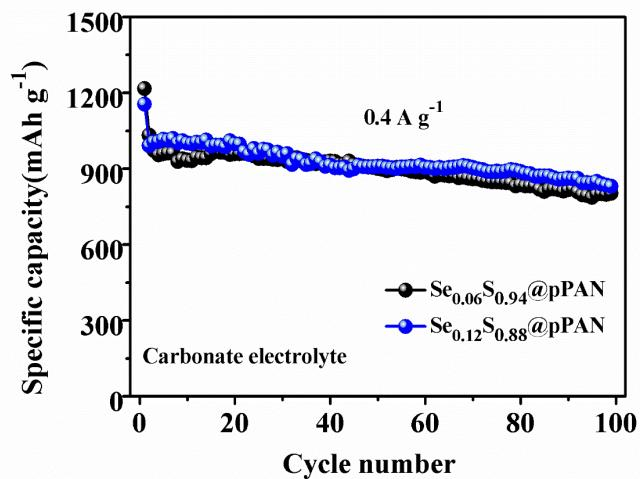
**Fig. S7** Cycle performance of  $\text{Se}_{0.06}\text{S}_{0.94}\text{@pPAN}$  and  $\text{Se}_{0.12}\text{S}_{0.88}\text{@pPAN}$  composite cathode in carbonate electrolyte.
