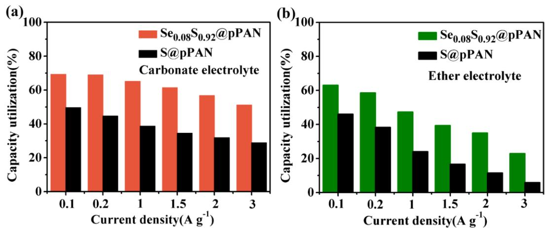
**Fig. S6** Comparisons of capacity utilization rates between  $\text{Se}_{0.08}\text{S}_{0.92}\text{@pPAN}$  and  $\text{S@pPAN}$  in carbonate electrolyte (a) and in ether electrolyte (b).
