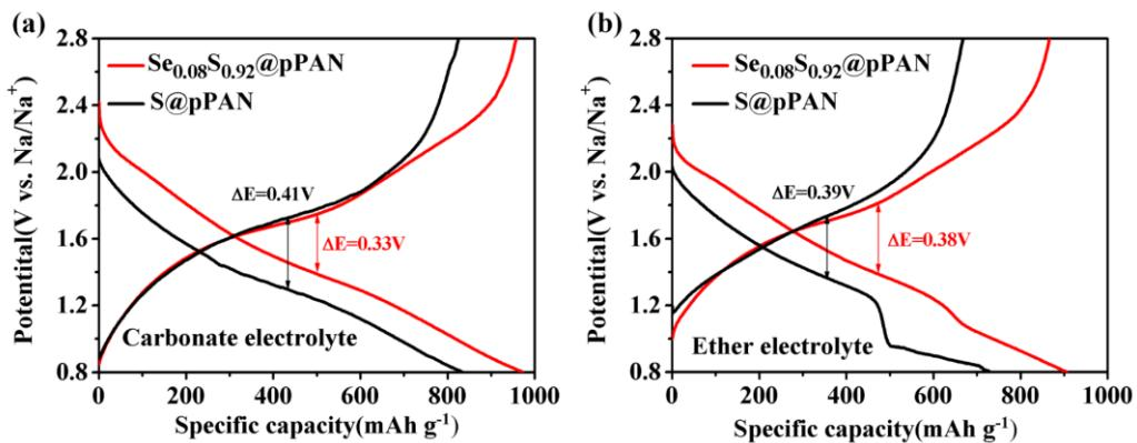
**Fig. S9** Discharge/charge curves of  $\text{Se}_{0.08}\text{S}_{0.92}@\text{pPAN}$  and  $\text{S}@\text{pPAN}$  electrodes in carbonate electrolyte (a) and in ether electrolyte (b).
