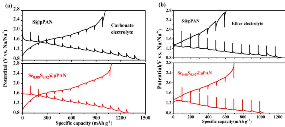
**Fig. S12** GITT voltage profiles of the  $\text{Se}_{0.08}\text{S}_{0.92}@\text{pPAN}$  and of  $\text{S}@\text{pPAN}$  in carbonate electrolyte (a) and in ether electrolyte (b).
