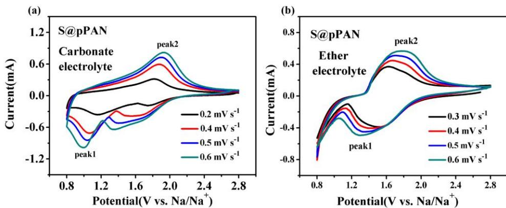
**Fig. S10** CV curves of  $\text{S}@\text{pPAN}$  in carbonate electrolyte (a) and in ether electrolyte (b).
