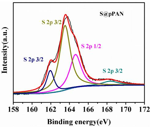
**Fig. S3** XPS spectra of S2p for S@pPAN.
