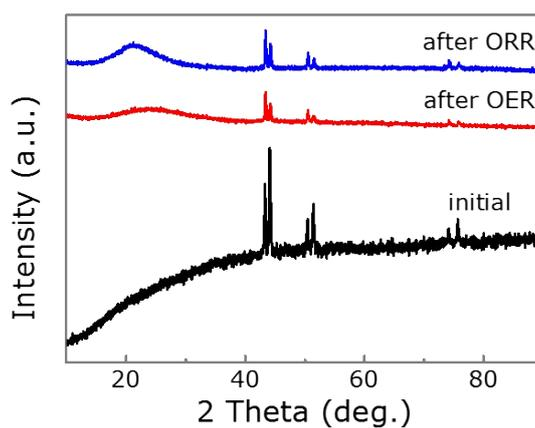
**Figure S14.** XRD results of CuCo@N-C after the stability test.
