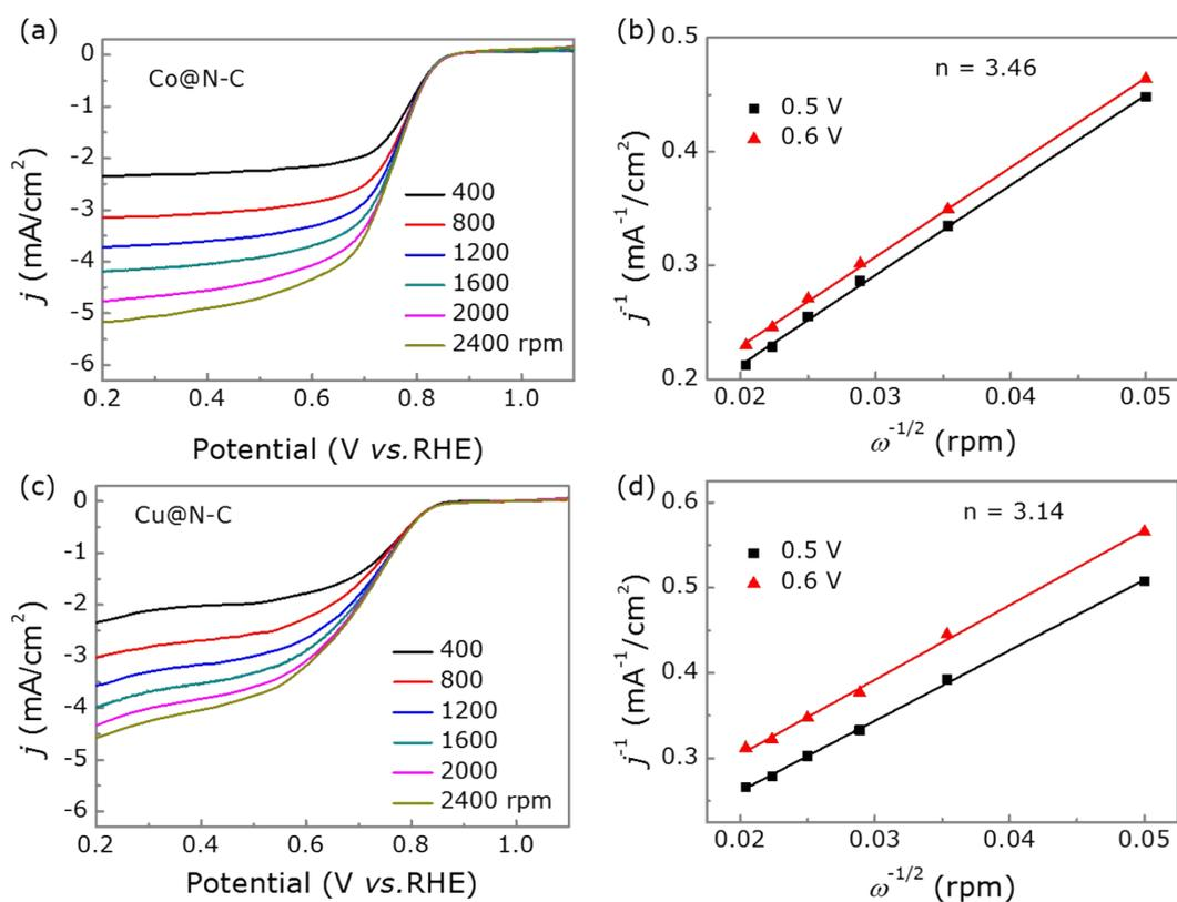
**Figure S8.** (a) LSV curves of ORR for Co@N-C at different rotation speeds and (b) the corresponding Koutecky–Levich plots. (c) LSV curves of ORR for Cu@N-C at different rotation speeds and (d) the corresponding Koutecky–Levich plots.
