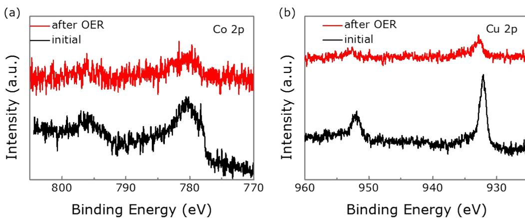
**Figure S15.** XPS results of CuCo@N-C after the OER test.
