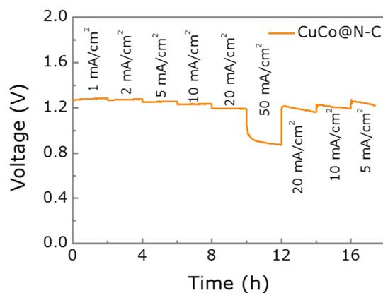
**Figure S17.** Discharge curves of the CuCo@N-C based ZABs at different current densities.
