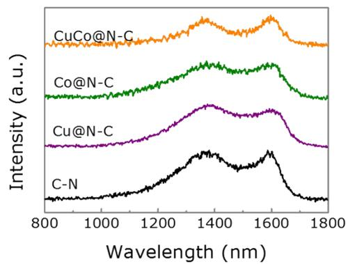
**Figure S1.** The Raman spectra of catalysts CuCo@N-C, Co@N-C, Cu@N-C and N-C.
