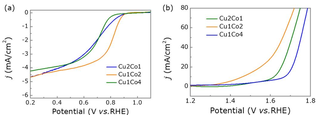
**Figure S7.** (a) LSV polarization curves of ORR for all the catalysts (Cu : Co= 2 : 1, 1 : 2 and 1 : 4, respectively.) at 1600 rpm. (b) LSV polarization curves of OER for all the catalysts (Cu : Co= 2 : 1, 1 : 2 and 1 : 4, respectively.).
