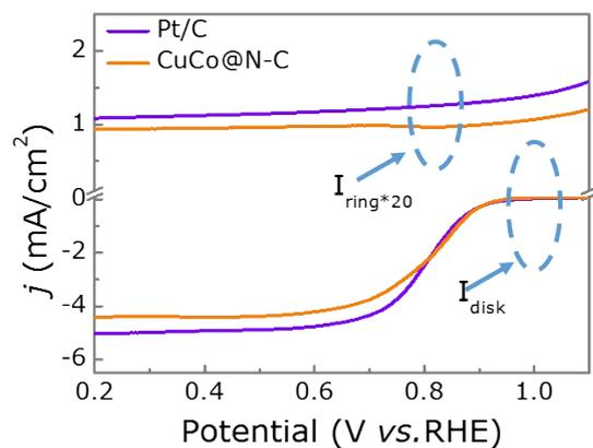
**Figure S9.** The RRDE curves for CuCo@N-C and Pt/C in O<sub>2</sub> saturated 0.1 M KOH at 1600 rpm.
