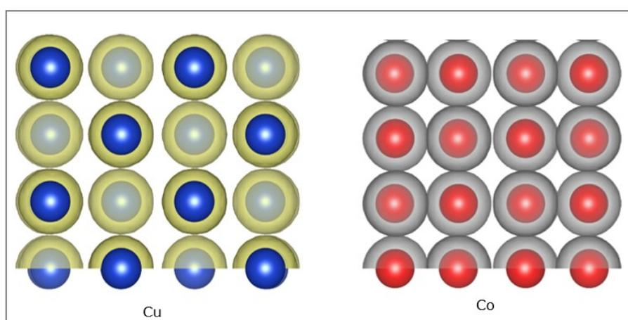
**Figure S6.** The charge density of Cu and Co with the isosurface value of 0.05 e/bohr<sup>3</sup>.
