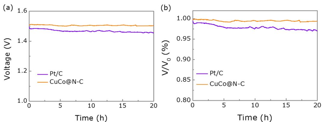
**Figure S18.** (a) The Open circuit voltage of Pt/C and CuCo@N-C. (b) The percentage of  $V/V_0$  for Pt/C and CuCo@N-C.
