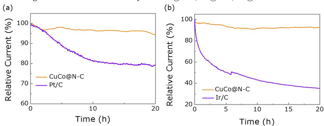
**Figure S13.** (a) The chronopotentiometric response of ORR for catalyst CuCo@N-C and Pt/C (20%) at a constant voltage of 0.7 V vs. RHE. (b) The chronopotentiometric response of OER for CuCo@N-C and Ir/C (20%) at a constant voltage of 1.50 V vs. RHE.
