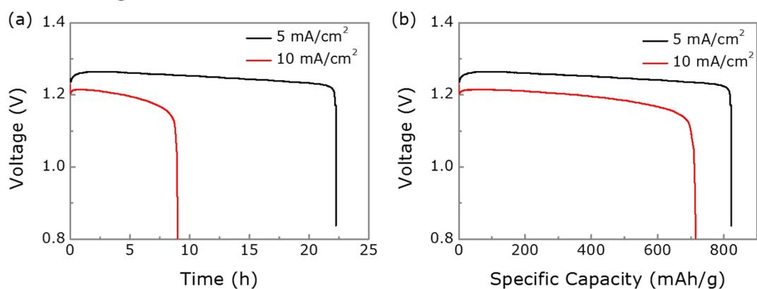
**Figure S19.** (a) Discharge curves at the current density of 5 mA/cm<sup>2</sup>, 10 mA/cm<sup>2</sup> and (d) the corresponding specific capacities of the CuCo@N-C based battery, respectively.
