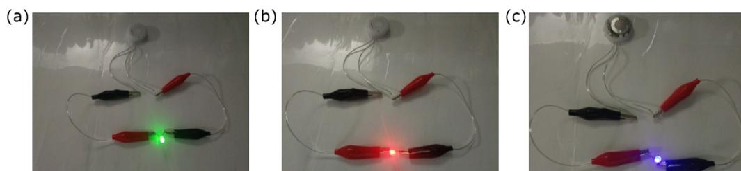
**Figure S21.** (a), (b) and (c) The photograph of a blue, green and red LED powered by two tandem all-solid-state ZABs.
