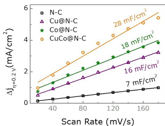
**Figure S11.** ECSA results of catalysts CuCo@N-C, Co@N-C, Cu@N-C and N-C.
