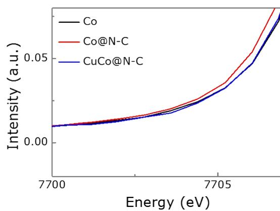
**Figure S3.** XANES spectrum of Co foil, Co@N-C and CuCo@N-C.
