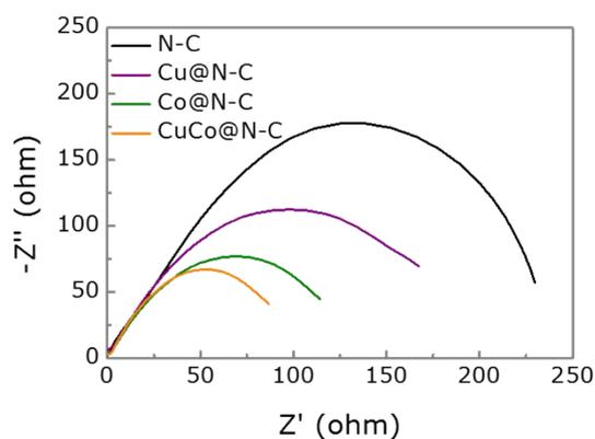
**Figure S10.** EIS curves of catalysts CuCo@N-C, Co@N-C, Cu@N-C and N-C.
