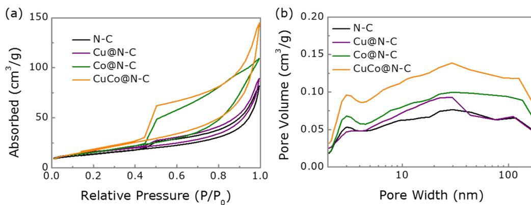
**Figure S4.** (a) BET plots and (b) pore width of CuCo@N-C, Co@N-C, Cu@N-C and N-C.
