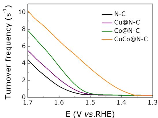
**Figure S12.** TOF results of catalysts CuCo@N-C, Co@N-C, Cu@N-C and N-C.
