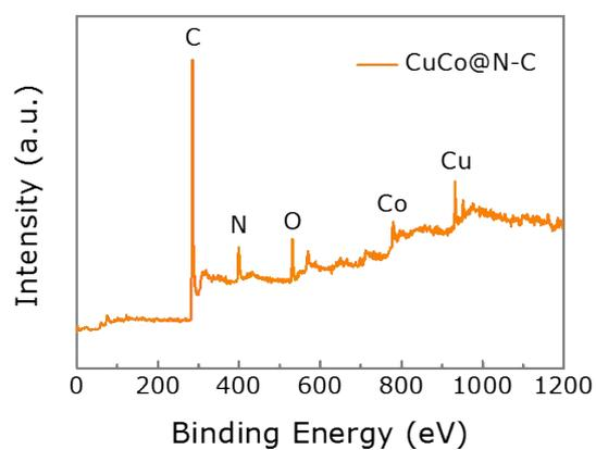
**Figure S5.** The XPS spectrum of CuCo@N-C.
