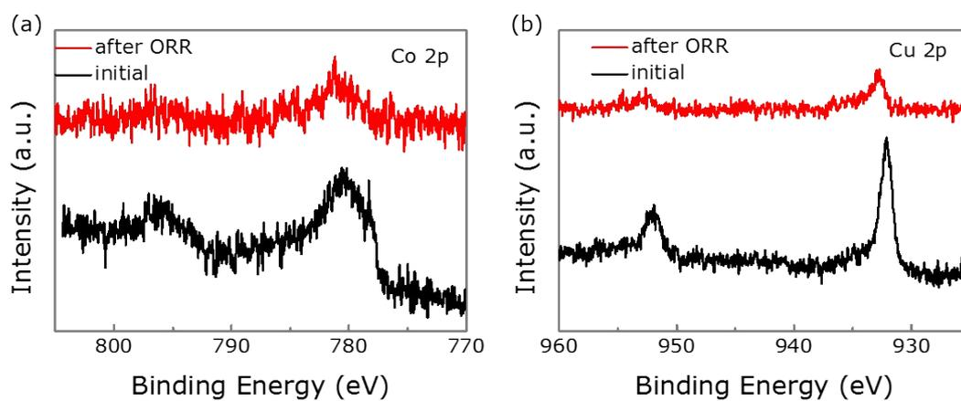
**Figure S16.** XPS results of CuCo@N-C after the ORR test.
