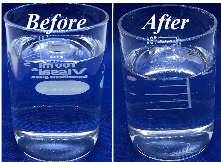
Fig. S16. Optical images of the bulk saturated NaCl solution. The recrystallized salts are not found in saturated NaCl solution, when the extra salt on the upper of evaporator fully disappeared.
