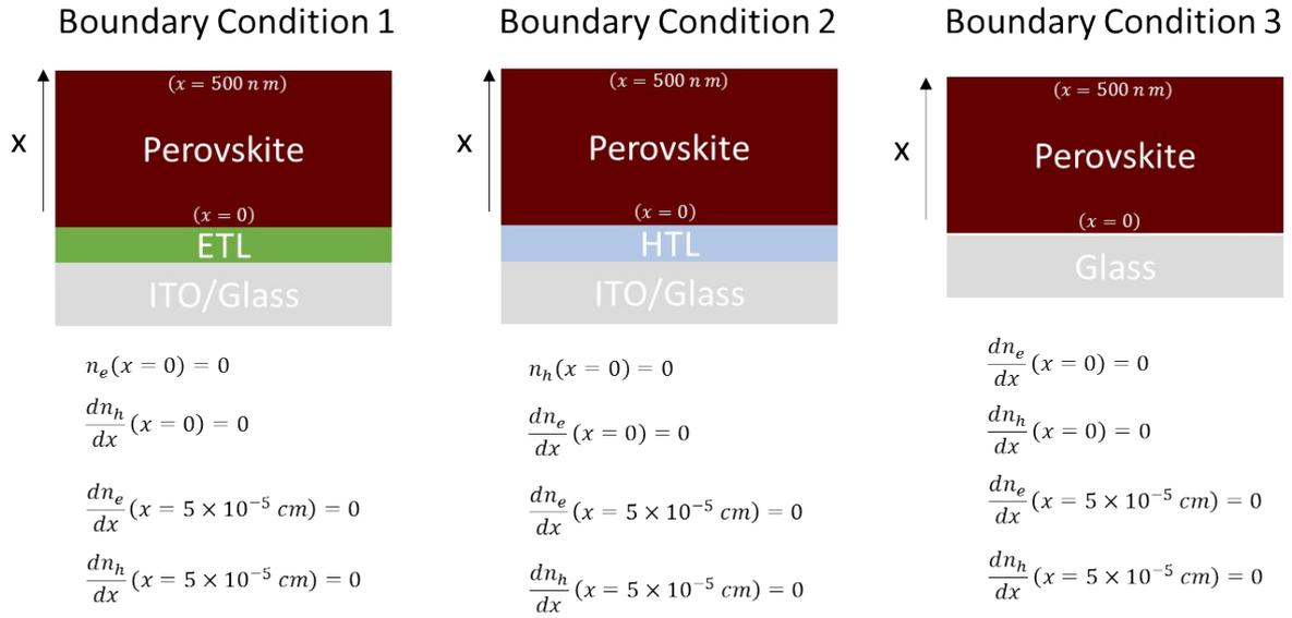
**Supplementary Information Figure 2.** Boundary conditions for ETL/MAPbI<sub>3</sub>, the HTL/MAPbI<sub>3</sub>, and the glass/MAPbI<sub>3</sub> devices to solve equation 14 and 15.
