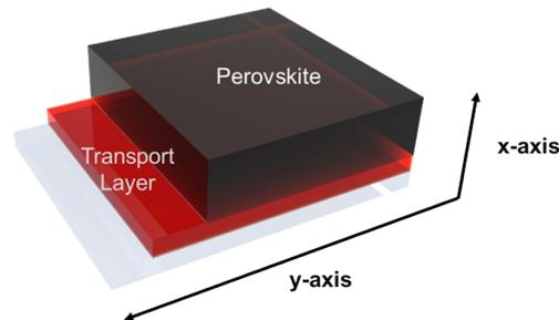
**Supplementary Information Figure 1.** Simplified 1-d model for Transport Layer/Perovskite using in this calculation
