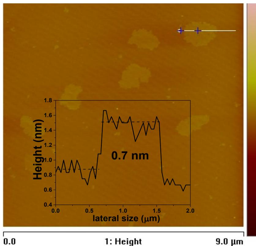
**Figure S4.** Atomic force microscopic (AFM) image of single layer NiPS<sub>3</sub> and corresponding height profile (inset).
