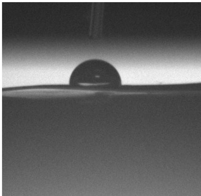
**Figure S14.** Water contact angle data on NiPS<sub>3</sub> film (80°).
