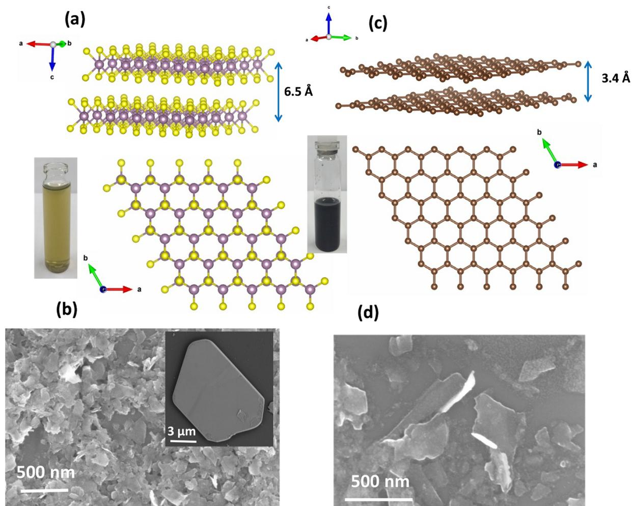
**Figure S2.** Structural representation of (a) MoS<sub>2</sub> along with the (b) scanning electron microscopic (SEM) images of bulk and few-layer MoS<sub>2</sub> and (c) graphene along with the (d) SEM image.
