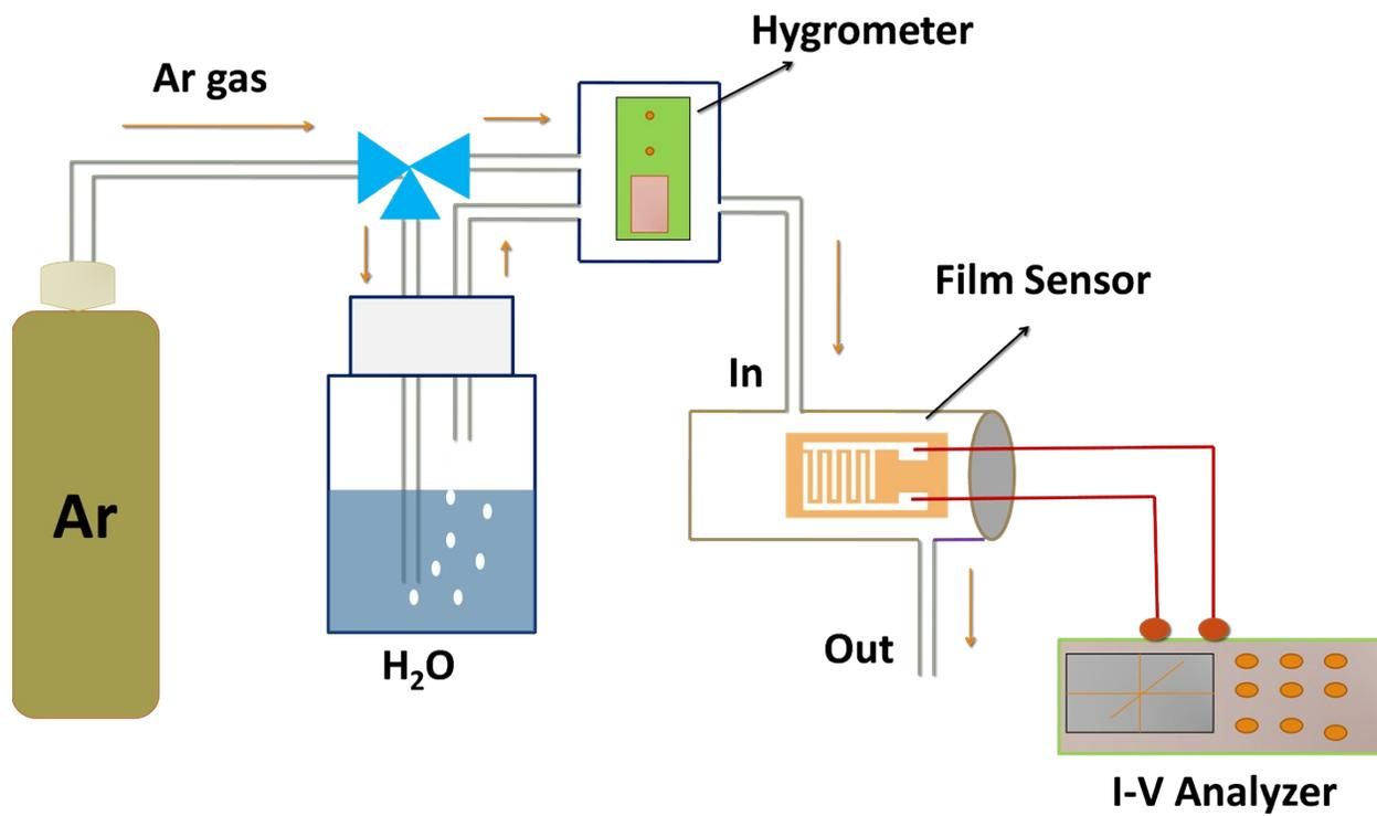
**Figure S1.** Schematic diagram of humidity sensor setup.
