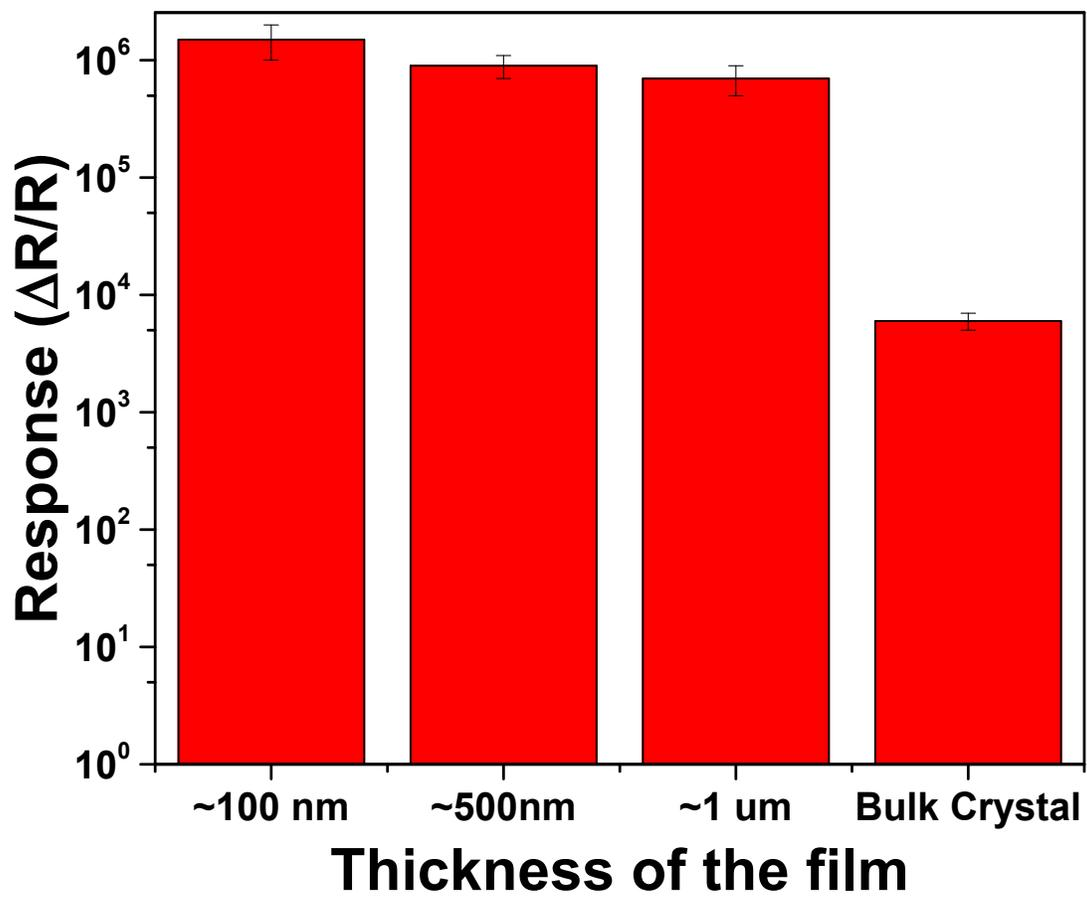
**Figure S9.** Thickness dependent humidity sensing performance of restacked few-layer NiPS<sub>3</sub> films of various thicknesses ( $\sim 100$ nm,  $\sim 500$ nm and  $\sim 1000$ nm) and bulk crystal.
