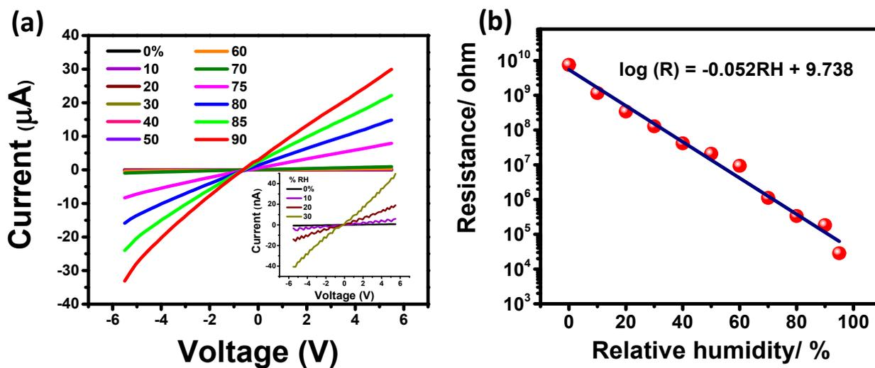
**Figure S5.** (a) I-V profiles of NiPS<sub>3</sub> obtained at different relative humidity (RH) values. (b) log(R) vs RH.
