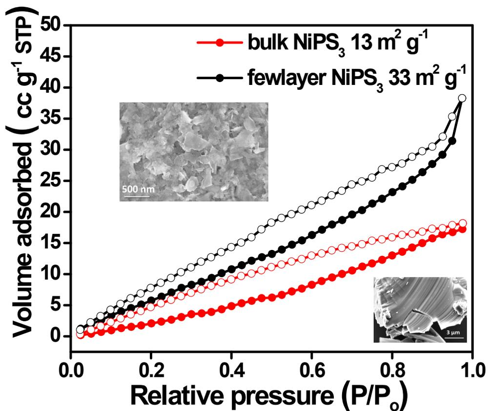
**Figure S3.** BET adsorption – desorption isotherms of bulk and few-layer NiPS<sub>3</sub>. BET measurements are carried out in N<sub>2</sub> atmosphere and at 77K temperature.
