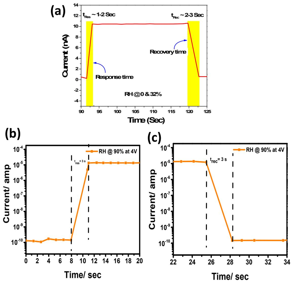
**Figure S7.** (a) Response vs recovery time at low humidity (RH of 0% to 32%); (b, c) denote high humidity response and recovery between RH of 0% to 90%.
