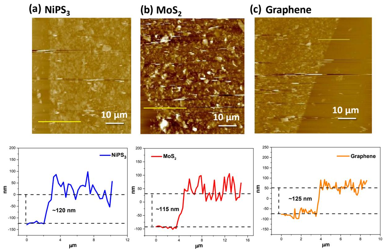
**Figure S6.** Atomic force microscopic images of thin films a) NiPS<sub>3</sub>, b) MoS<sub>2</sub> and c) Graphene along with corresponding height profiles.
