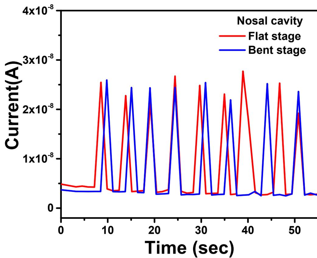
**Figure S12.** Current response to RH of the breath exhaled from the nasal cavity in both flat and bent configurations.
