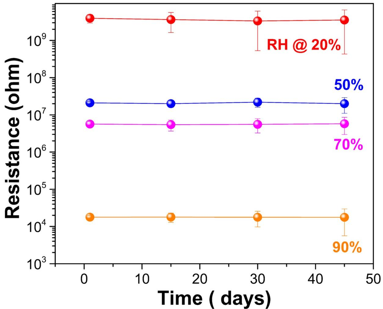
**Figure S8.** Stability of few-layer NiPS<sub>3</sub> humidity sensor over storage time for various humidity levels.
