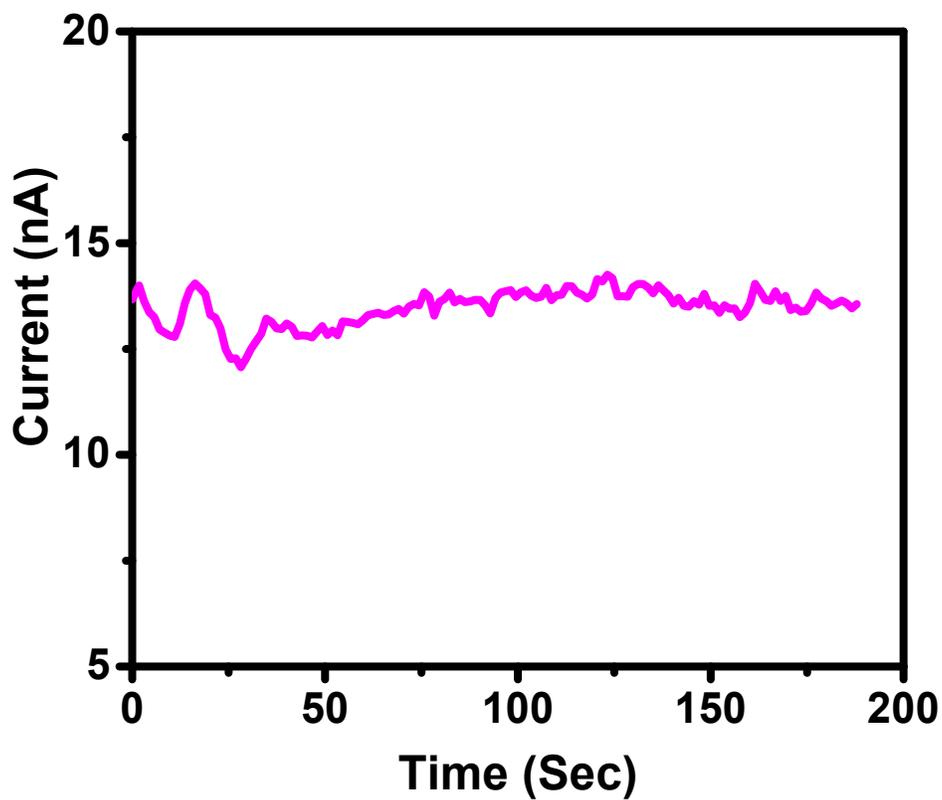
**Figure S13.** Response of the sensor for glove wearing hand. The base current is due the ambient humidity in the laboratory.
