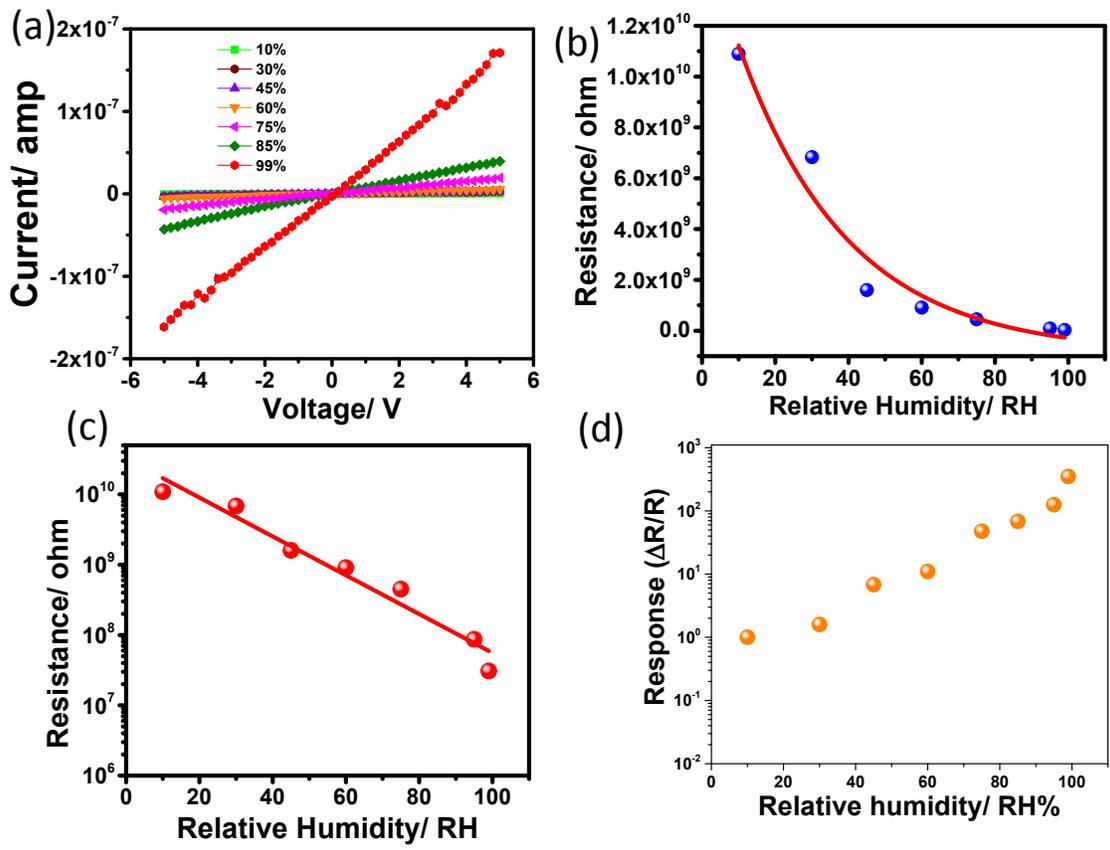
**Figure S10.** (a) I-V profiles obtained for the device based on bulk NiPS<sub>3</sub> at different relative humidity (RH) values (b) Resistance (R) vs RH at different ranges of humidity; (c) Log(R) vs RH, (d) Responsivity ( $\Delta R/R$ ) vs. RH of bulk NiPS<sub>3</sub>.
