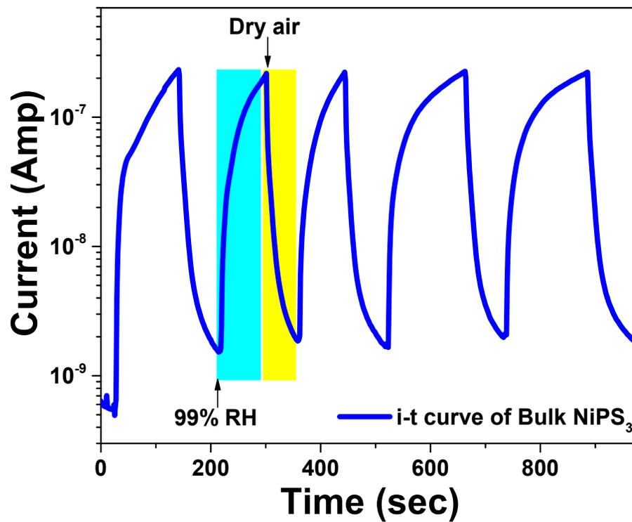
**Figure S11.** Response of bulk NiPS<sub>3</sub> based sensor between dry air and 99% RH.
