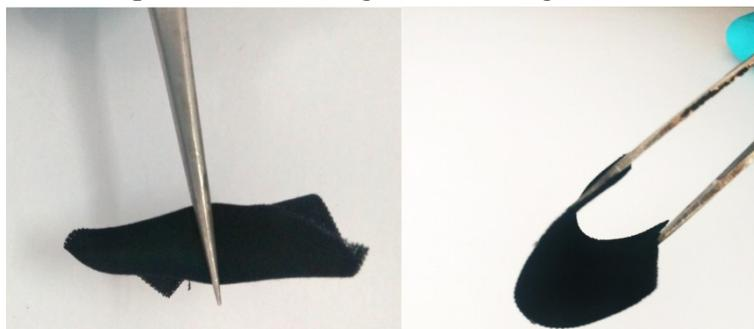
**Fig. S2.** The flexible display of C@NiSe<sub>2</sub>.
