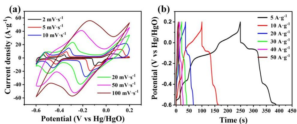
Fig. S5 CV and GCD curves of MoO<sub>3-x</sub> nanobelts electrode tested at 0°C.
