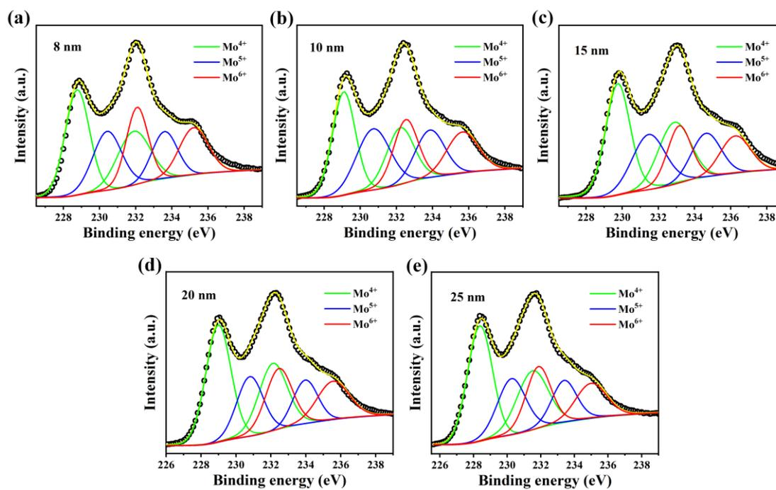
Fig. S3 XPS spectra of MoO<sub>3-x</sub> nanobelts in different depth from 8 to 25 nm.
