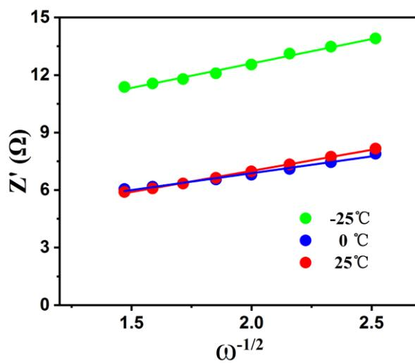
Fig. S7 Linear relationship between  $z'$  and  $\omega^{-1/2}$  in low frequency region.
