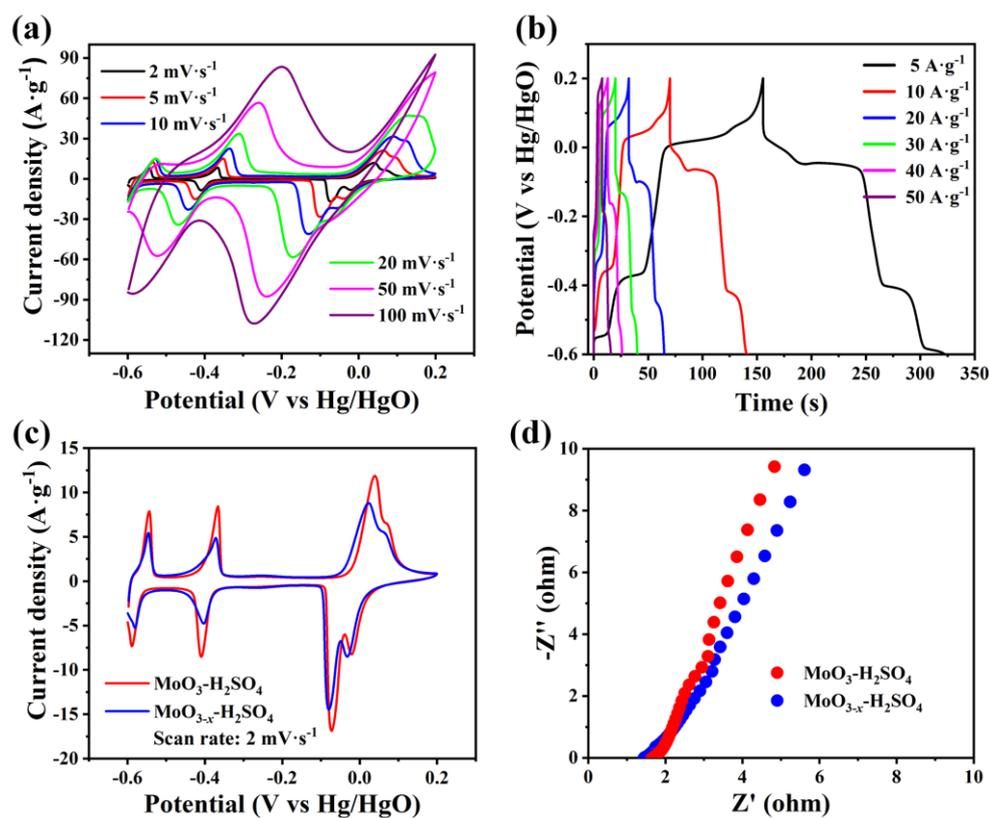
Fig. S4 (a) and (b) CV and GCD curves of MoO<sub>3</sub> nanobelts electrode tested in H<sub>2</sub>SO<sub>4</sub>; Comparison of MoO<sub>3</sub> and MoO<sub>3-x</sub> nanobelts electrodes: (c) CV curves and (d) EIS plots.
