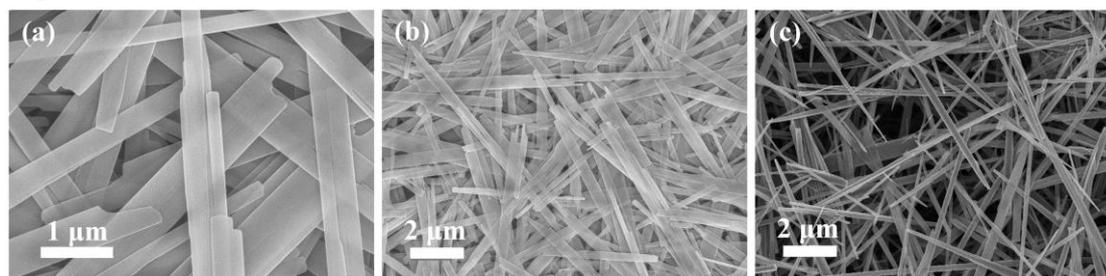
**Fig. S1** SEM images of MoO<sub>3</sub> nanobelts with different magnifications (a, b) and MoO<sub>3-x</sub> nanobelts (c).
