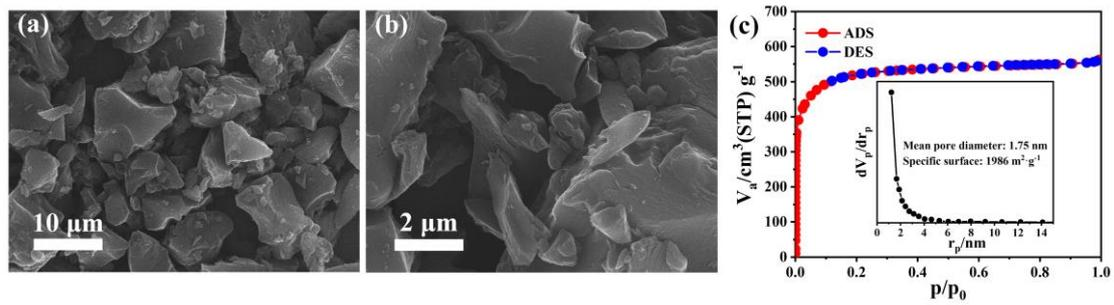
**Fig. S8** (a) and (b) SEM images of AC with different magnifications; (c) BET test result of AC.
