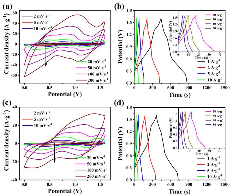
Fig. S6 CV and GCD curves of AC//MoO<sub>3-x</sub> tested at 0°C (a, b) and -25°C (c, d).
