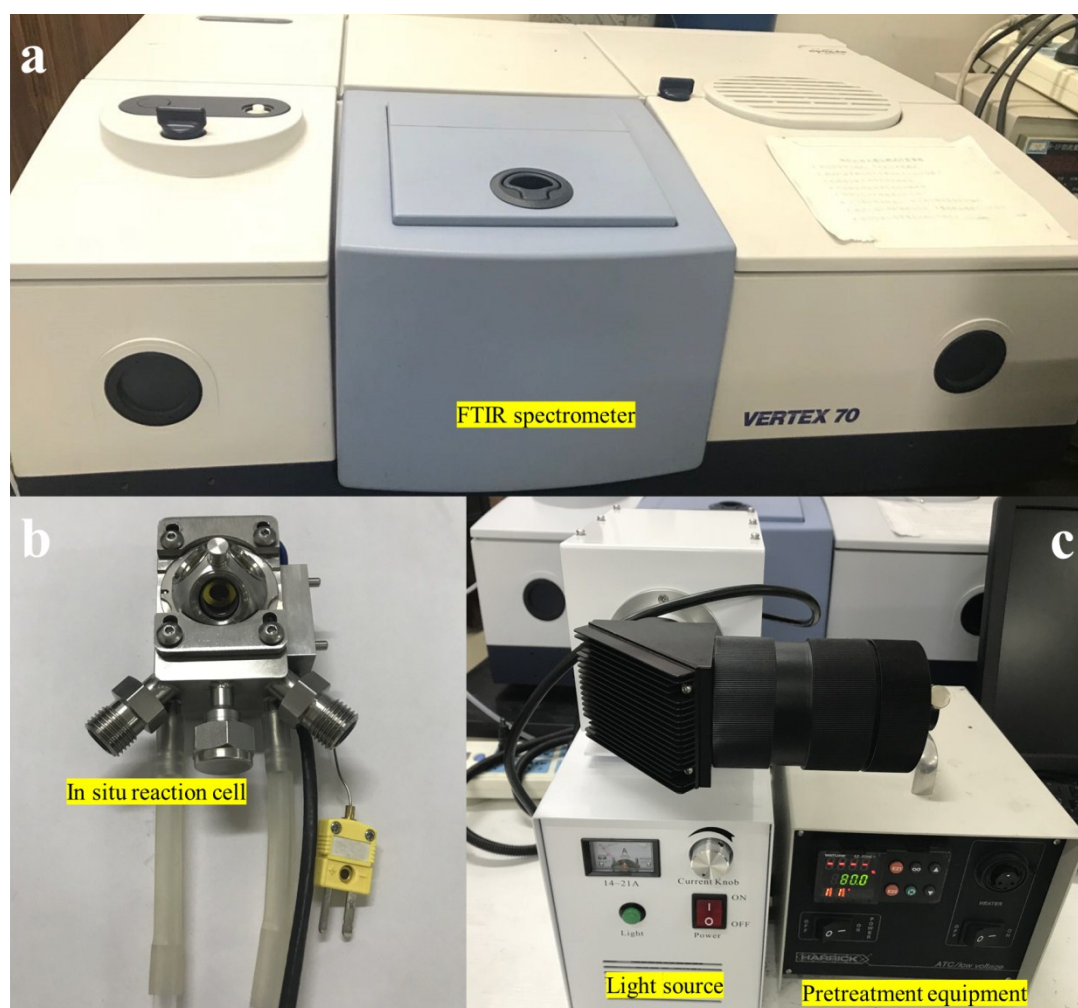
Scheme S2. (a) VERTEX 70 spectrometer (Bruker, Germany); (b) In situ reaction cell; (c) Pretreatment equipment and light source.
