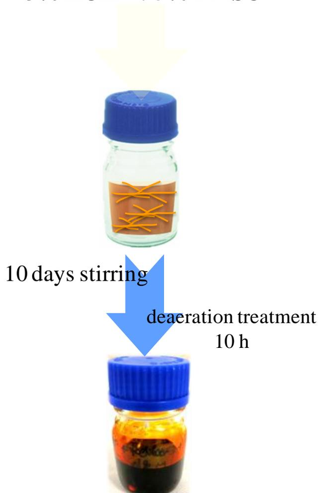
**Fig. S4.** Schematic diagram of preparation of membrane casting solution.
