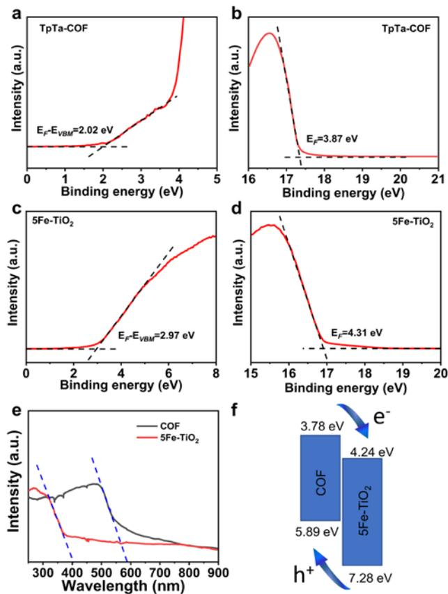
**Fig. S7** The UPS spectra and the band alignment of TpTa-COF and 5Fe-TiO<sub>2</sub>.
