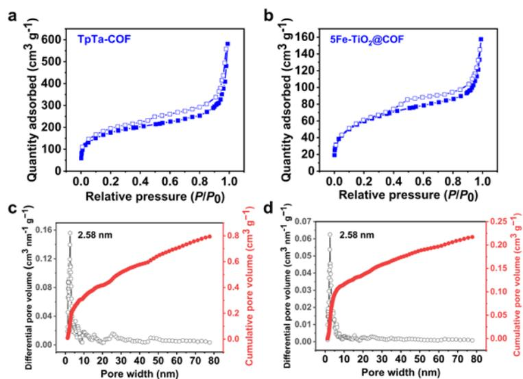
**Fig. S8** The Nitrogen adsorption and desorption isotherms of TpTa-COF (a) and 5Fe-TiO<sub>2</sub>@COF (b), DFT plots for TpTa-COF (c) and 5Fe-TiO<sub>2</sub>@COF (d).
