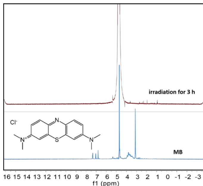
**Fig. S15** The NMR spectra of 40 mg L<sup>-1</sup> MB in D<sub>2</sub>O before and after degradation in ambient light. After 3 h of degradation, the NMR spectrum does not show the peaks corresponding to MB.
