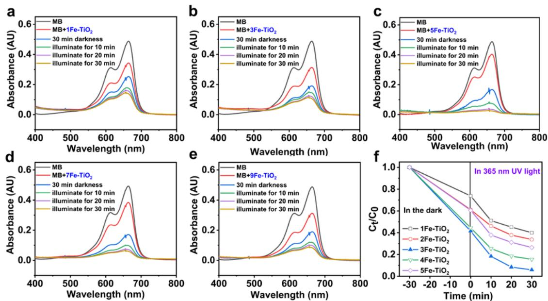
**Fig. S12** The time-dependent UV-vis absorption spectra of the MB samples (40 mg L<sup>-1</sup>) degraded by various catalysts (1 mg mL<sup>-1</sup>, 0.4 mL): 1Fe-TiO<sub>2</sub> (a), 3Fe-TiO<sub>2</sub> (b), 5Fe-TiO<sub>2</sub> (c), 7Fe-TiO<sub>2</sub> (d) and 9Fe-TiO<sub>2</sub> (e); The MB degradation percentage (C<sub>t</sub>/C<sub>0</sub>) calculated from the figures a-e (f). An LED light (365 nm) with a power of 21 W was used as the light source.
