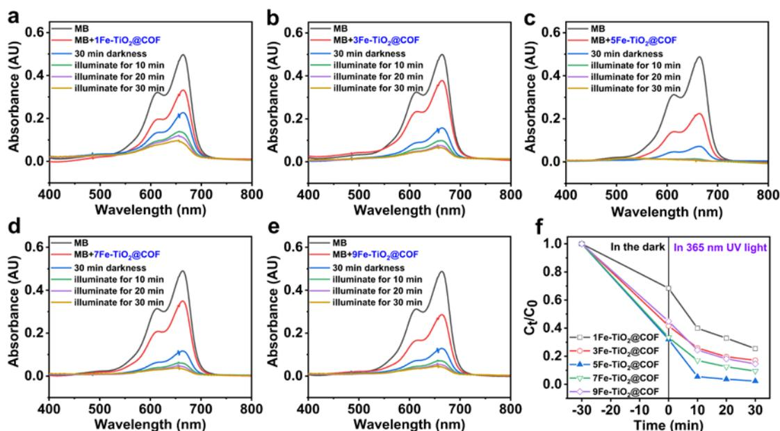
**Fig. S13** The time-dependent UV-vis absorption spectra of the MB samples (40 mg L<sup>-1</sup>) degraded by various catalysts (1 mg mL<sup>-1</sup>, 0.4 mL): 1Fe-TiO<sub>2</sub>@COF (a), 3Fe-TiO<sub>2</sub>@COF (b), 5Fe-TiO<sub>2</sub>@COF (c), 7Fe-TiO<sub>2</sub>@COF (d) and 9Fe-TiO<sub>2</sub>@COF (e); The MB degradation percentage (C<sub>t</sub>/C<sub>0</sub>) calculated from the figures a-e (f). LED light (365 nm) with a power of 21 W was used as the light source.
