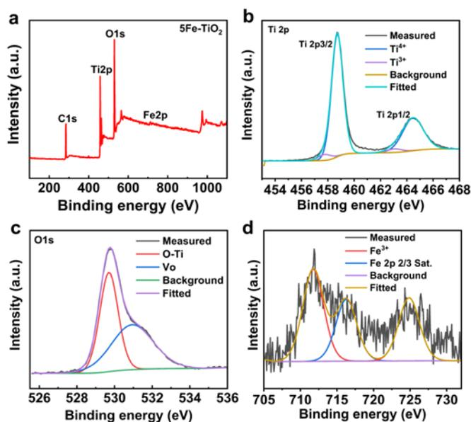
**Fig. S2** The XPS spectra of 5Fe-TiO<sub>2</sub> (a), high resolution XPS spectra of each element in 5Fe-TiO<sub>2</sub> (b-d).
