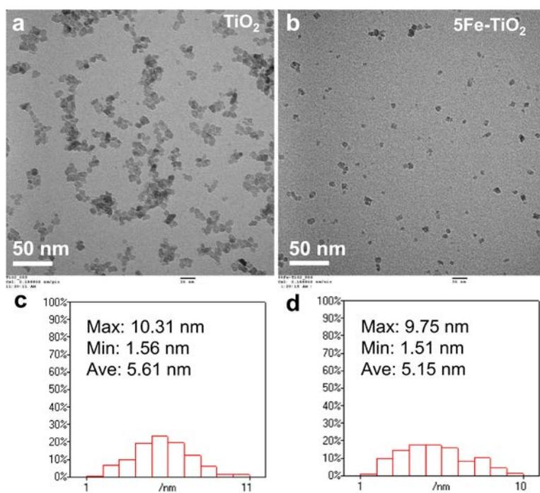
**Fig. S10** The TEM images of TiO<sub>2</sub> (a) and 5Fe-TiO<sub>2</sub> (b); The size distribution of TiO<sub>2</sub> (c) and 5Fe-TiO<sub>2</sub> (d).
