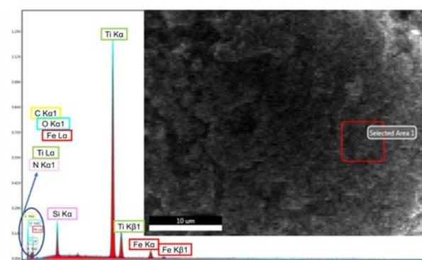
**Fig. S5** The EDS spectrum of 5Fe-TiO<sub>2</sub>@COF, inset: The SEM image of 5Fe-TiO<sub>2</sub>@COF.
