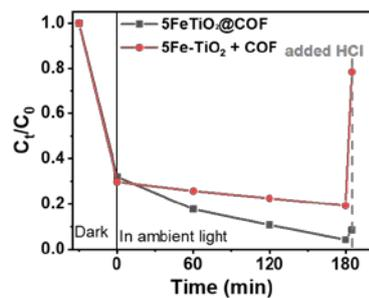
**Fig. S17** The comparison of photocatalytic activity of 5Fe-TiO<sub>2</sub>@COF and physically mixed 5Fe-TiO<sub>2</sub> and COF in the ambient light.
