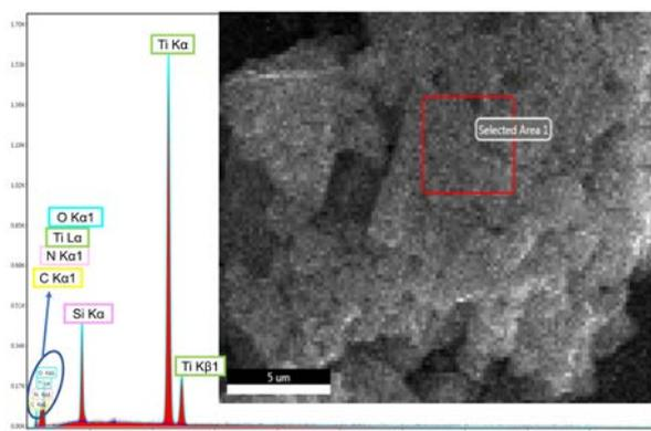
**Fig. S4** The EDS spectrum of TiO<sub>2</sub>@COF, inset: The SEM image of TiO<sub>2</sub>@COF.
