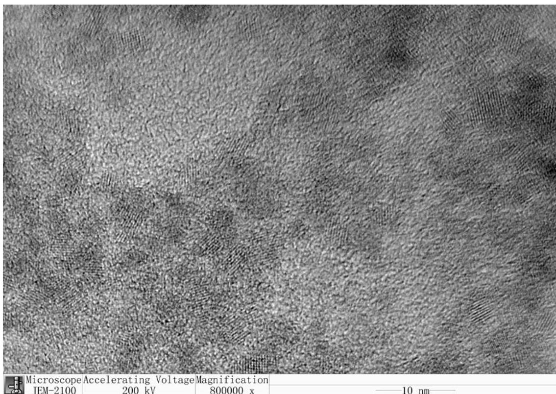
**Fig. S9** The TEM images of 5Fe-TiO<sub>2</sub>@COF.
