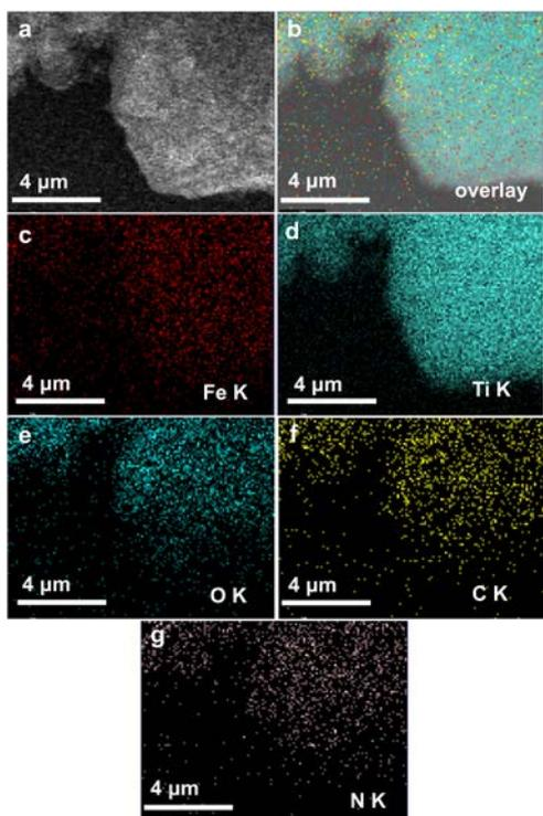
**Fig. S6** The EDS mapping of 5Fe-TiO<sub>2</sub>@COF.
