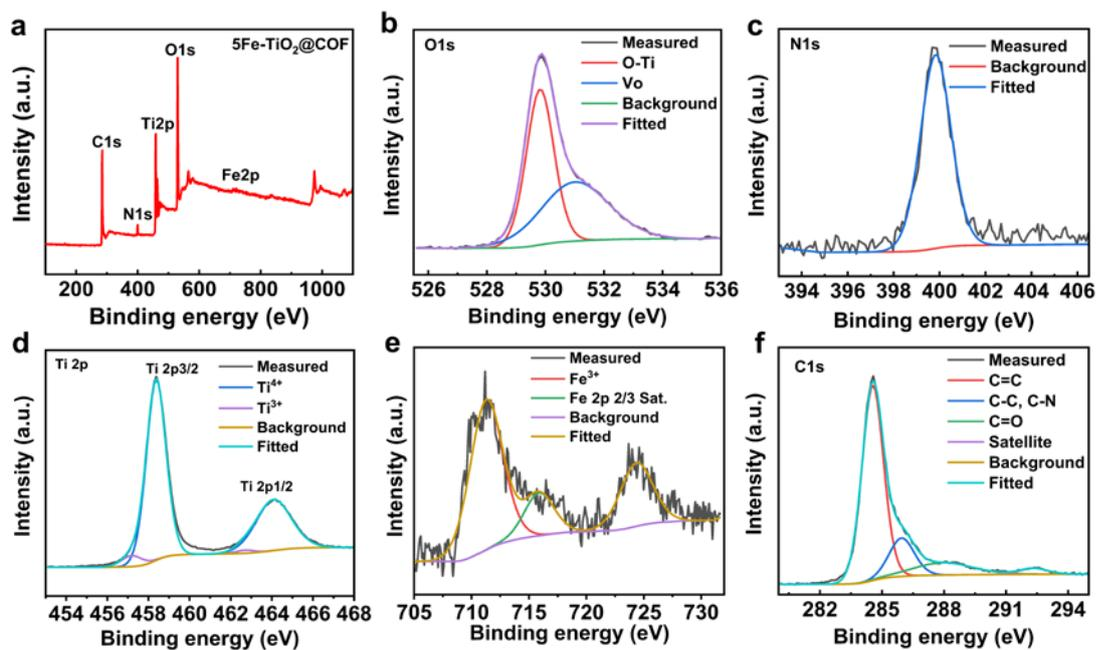
**Fig. S3** The XPS spectra of 5Fe-TiO<sub>2</sub>@COF (a), high resolution XPS spectra of each element in 5Fe-TiO<sub>2</sub>@COF (b-f).
