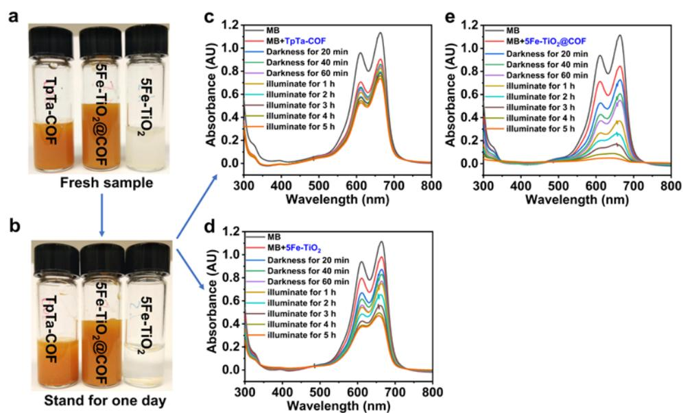
**Fig. S20** The MB degradation tests using freshly-made and one-day-aged catalysts: the images of freshly made catalysts (a) and one-day-aged catalysts (b); The time-dependent UV-vis absorption spectra of the MB samples ( $100 \text{ mg L}^{-1}$ ) degraded by TpTa-COF (c),  $5\text{Fe-TiO}_2$  (d) and  $5\text{Fe-TiO}_2@\text{COF}$  (e) under ambient light.
