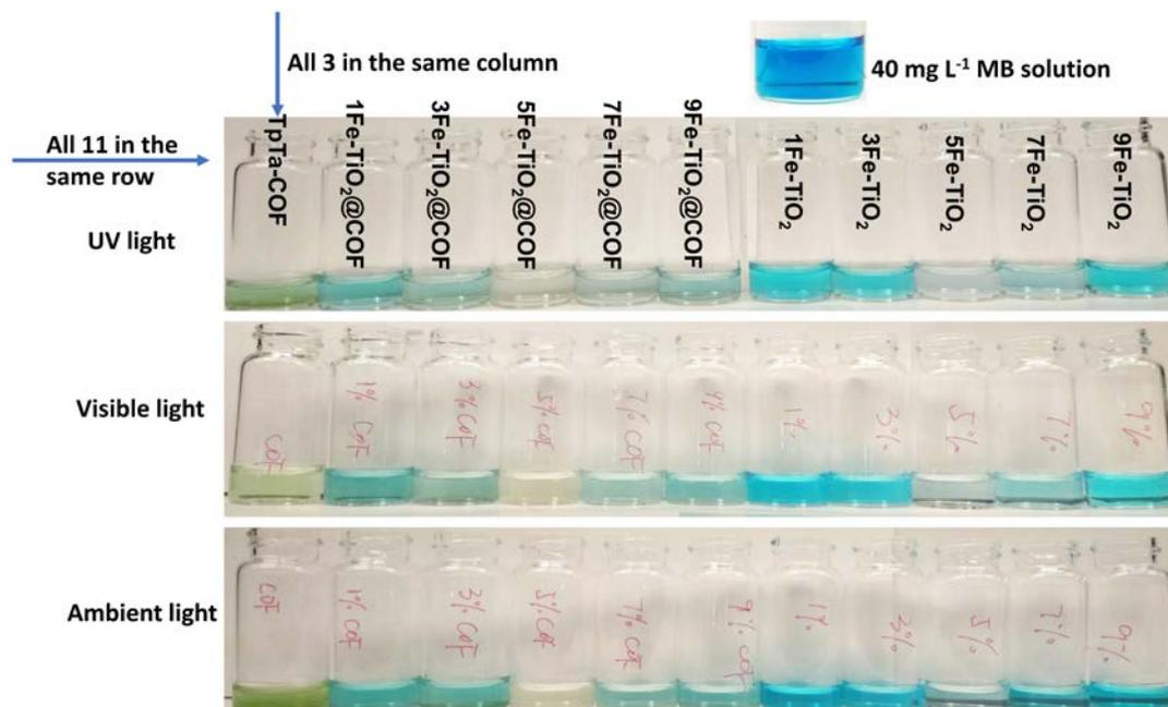
**Fig. S11** Decoloration of MB samples containing various catalysts when illuminated with different light sources.
