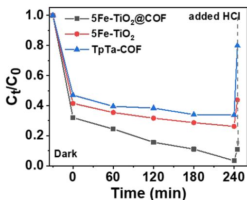
**Fig. S14** The comparison of photocatalytic activity of 5Fe-TiO<sub>2</sub>@COF, 5Fe-TiO<sub>2</sub> and TpTa-COF in MB (40 mg L<sup>-1</sup>) degradation in the dark.
