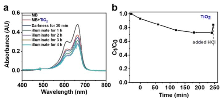
**Fig. S16** The photocatalytic activity of TiO<sub>2</sub> under ambient light.
