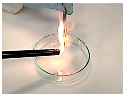
Fig. S4. Flammability of the CPE membrane with the DMF solvent.
