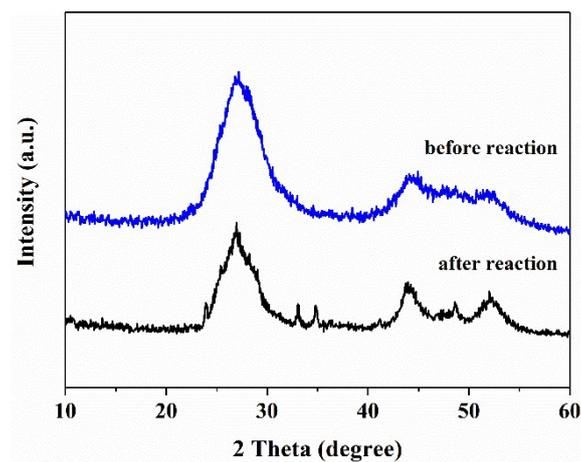
**Fig. S8.** XRD patterns of the CZ<sub>3</sub>P<sub>1</sub>S before and after cycling tests.
