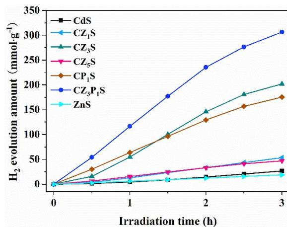
Fig. S7. Time courses of H<sub>2</sub> evolution over the as-synthesized samples.
