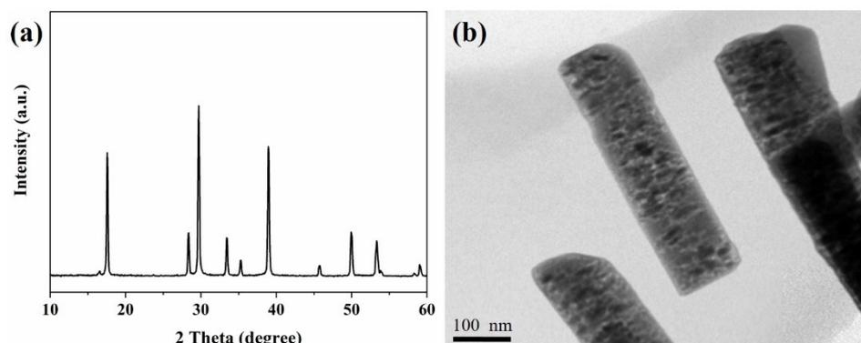
**Fig. S1.** The XRD pattern (a) and TEM image (b) of the as-prepared Cd(OH)Cl nanorods.
