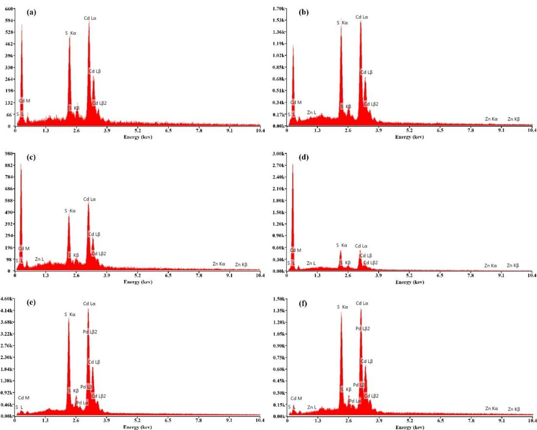
**Fig. S5.** EDX spectra of CdS (a), CZ<sub>1</sub>S (b), CZ<sub>3</sub>S (c), CZ<sub>5</sub>S (d), CP<sub>1</sub>S (e) and CZ<sub>3</sub>P<sub>1</sub>S (f).
