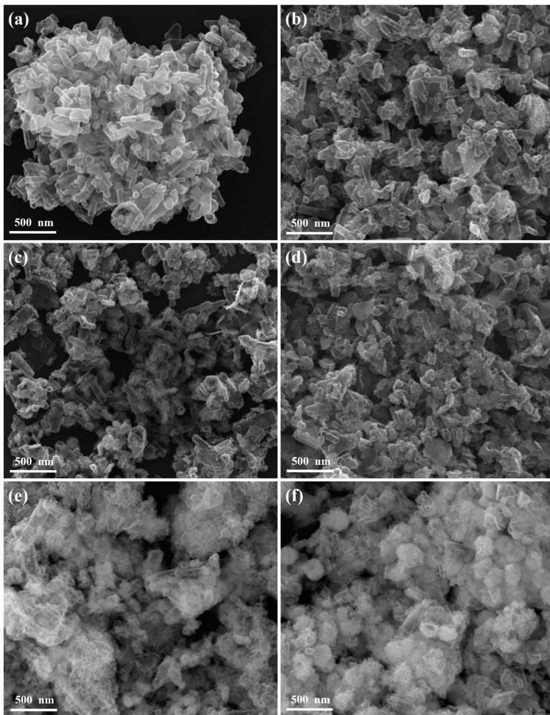
**Fig. S3.** SEM images of CdS (a), CZ<sub>1</sub>S (b), CZ<sub>3</sub>S (c), CZ<sub>5</sub>S (d), CP<sub>1</sub>S (e) and CZ<sub>3</sub>P<sub>1</sub>S (f).
