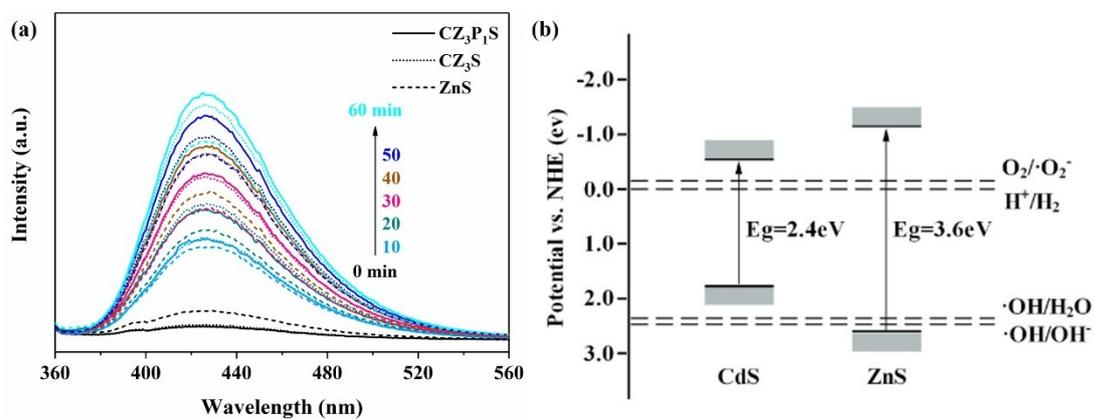
**Fig. S9.** PL spectra (a) of CZ<sub>3</sub>P<sub>1</sub>S, CZ<sub>3</sub>S and ZnS samples in a TA solution irradiated by simulated sunlight at different irradiation time (excitation at the wavelength of 315 nm), and the schematic diagram (b) of the band positions of CdS and ZnS.
