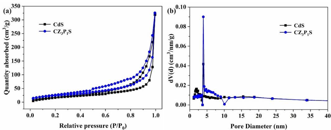
**Fig. S4.** N<sub>2</sub> adsorption-desorption isotherms (a) and pore size distribution curves (b) of CdS NTs and CZ<sub>3</sub>P<sub>1</sub>S catalyst.
