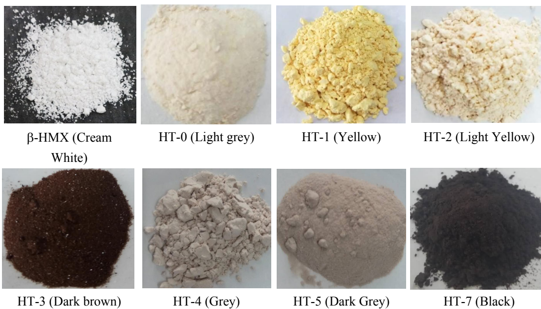
Figure S1. Appearance photographs of the industrial grade \beta -HMX and various HMX crystals doped with 2D TAGP material.
