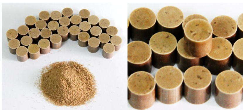
Figure S17. Modeling powder of HT-4 and corresponding cylindrical pressed charges for detonation velocity measurements: the scaled-up HT-4 has an average density of 1.94 \text{ g cm}^{-3} , but the pressed density is only 94% of the theoretical maximum density due to inhomogeneity of the crystals after scaling up.
