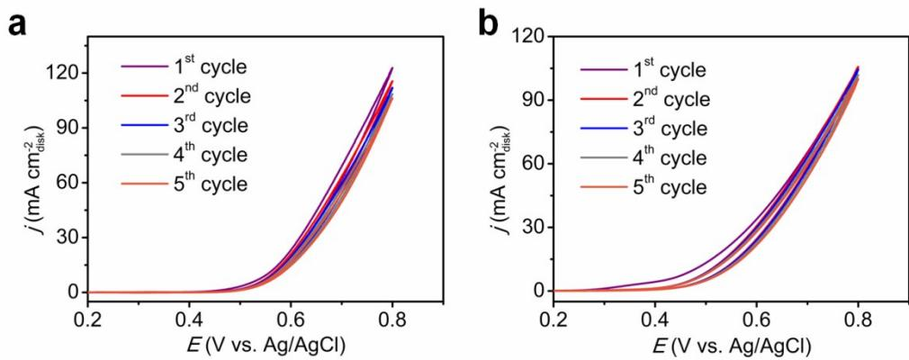
**Fig. S17.** Cyclic voltammograms of (a) RuO<sub>2</sub> and (b) RuS<sub>2</sub>-500 for 5 cycles within OER potential window.
