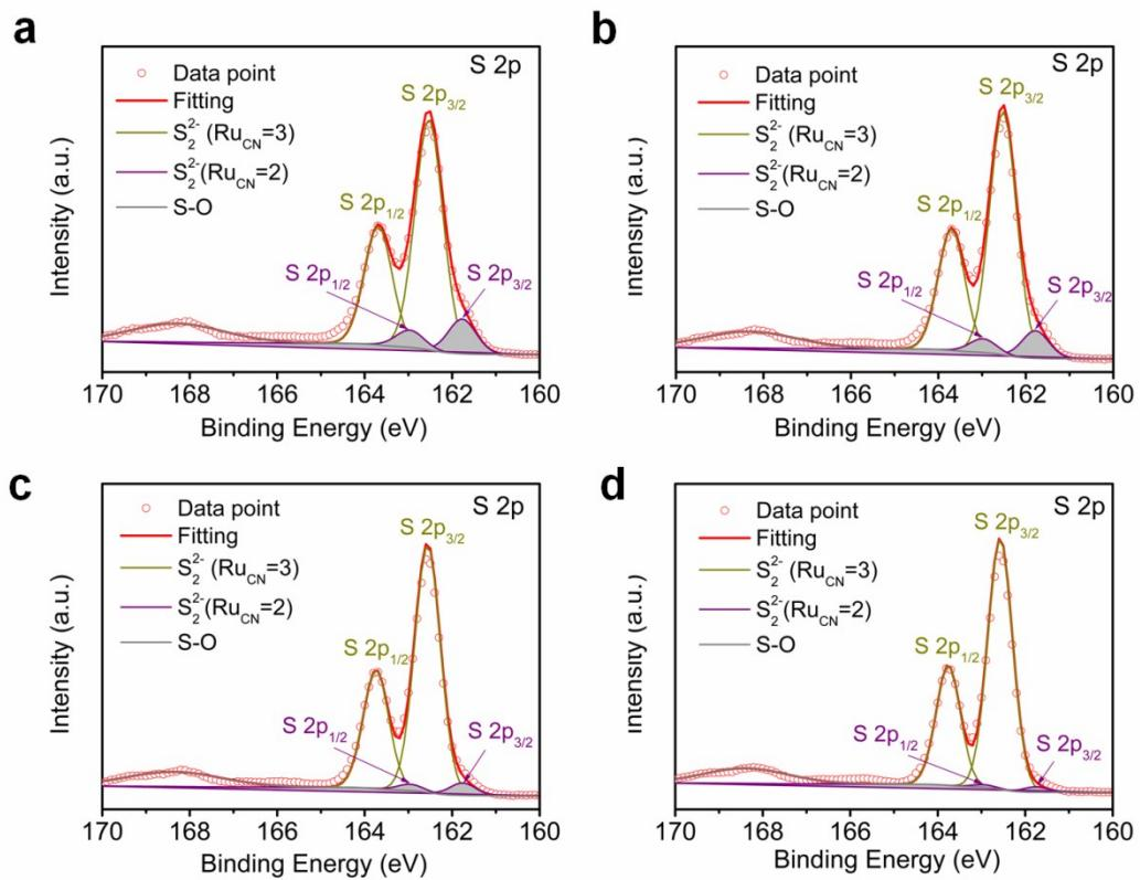
**Fig. S4.** Deconvoluted XPS S 2p spectra of (a) RuS<sub>2</sub>-400, and (b) RuS<sub>2</sub>-500, (c) RuS<sub>2</sub>-600 and (d) RuS<sub>2</sub>-700.
