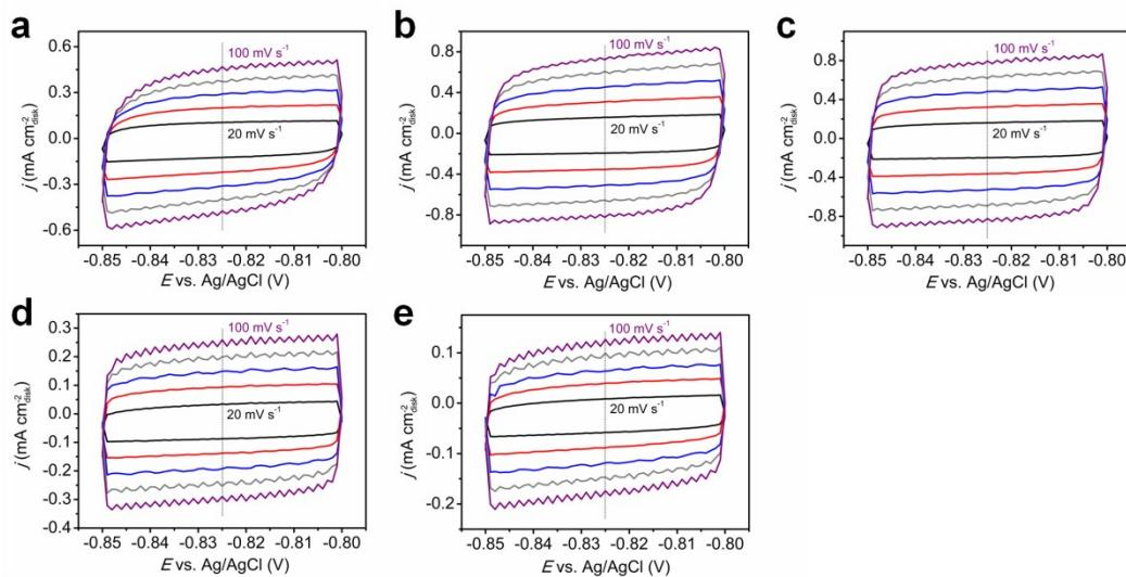
**Fig. S10.** CV measurements in a non-faradic current region (-0.85--0.8 V vs.  $\text{Ag}/\text{AgCl}$ ) at scan rates of 20, 40, 60, 80 and 100 mV s<sup>-1</sup> of (a)  $\text{RuO}_2$ , (b)  $\text{RuS}_2\text{-}400$ , (c)  $\text{RuS}_2\text{-}500$ , (d)  $\text{RuS}_2\text{-}600$  and (e)  $\text{RuS}_2\text{-}700$  catalysts in 1 M KOH solution.
