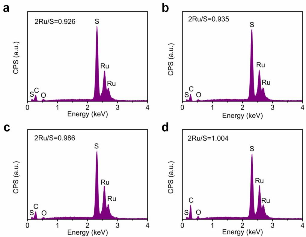
**Fig. S6.** EDX spectra of (a) RuS<sub>2</sub>-400, and (b) RuS<sub>2</sub>-500, (c) RuS<sub>2</sub>-600 and (d) RuS<sub>2</sub>-700.
