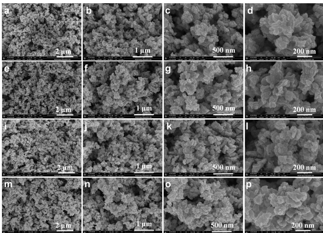
**Fig. S2.** SEM images with different magnifications of (a-d) RuS<sub>2</sub>-400, (e-h) RuS<sub>2</sub>-500, (i-l) RuS<sub>2</sub>-600 and (m-p) RuS<sub>2</sub>-700.
