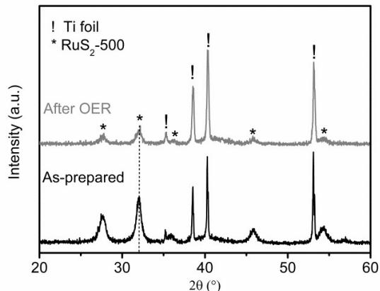
**Fig. S18.** XRD patterns of RuS<sub>2</sub>-500 loaded on the Ti foil substrate before and after OER for 50 cycles.
