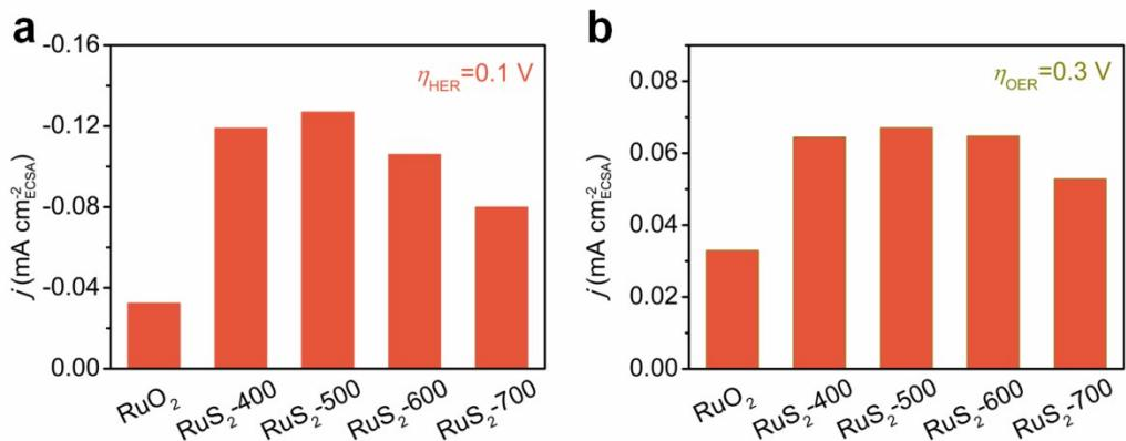
**Fig. S20.** Intrinsic activity of  $\text{RuO}_2$  and  $\text{RuS}_2\text{-T}$  for (a) HER and (b) OER.
