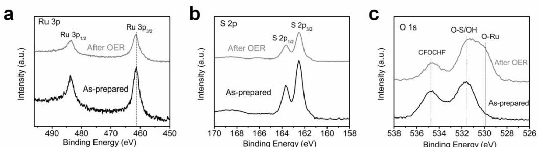
**Fig. S19.** XPS spectra of (a) Ru 3p, (b) S 2p and (c) O 1s for RuS<sub>2</sub>-500 before and after HER for 50 cycles. The peak of Ru 3p<sub>3/2</sub> slightly shifts to higher energy for post-OER samples, indicating partial oxidation on the surface. In O 1s, the peak at ~534.8 eV is originating from the CFOCHF of Nafion solution<sup>[1,2]</sup> which was included in the electrode preparation. The peaks at ~529-530 eV are associated with the lattice oxygen in metal oxides<sup>[3-5]</sup>.
