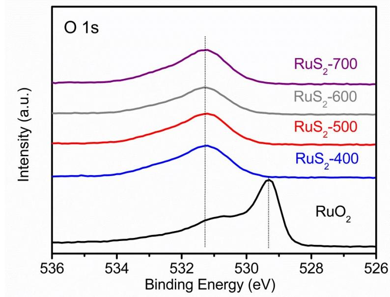
**Fig. S5.** XPS spectra of O1s for RuS<sub>2</sub>-T and RuO<sub>2</sub>.
