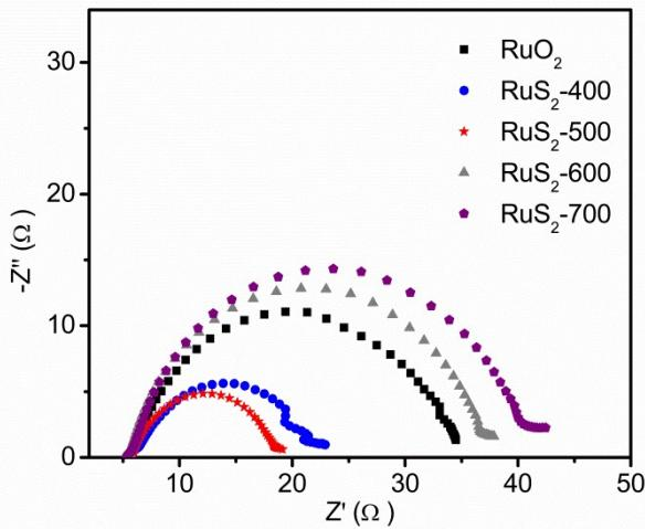
**Fig. S15.** Nyquist plots of  $\text{RuO}_2$ ,  $\text{RuS}_2\text{-}400$ ,  $\text{RuS}_2\text{-}500$ ,  $\text{RuS}_2\text{-}600$  and  $\text{RuS}_2\text{-}700$  catalysts recorded at 0.6 V vs. Ag/AgCl (no iR-corrected) under the influence of an AC voltage of 10 mV.
