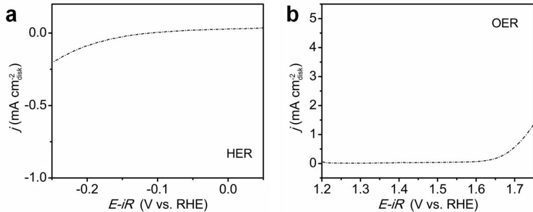
**Fig. S8.** (a) HER and (b) OER polarization curve of conductive carbon in 1 M KOH.
