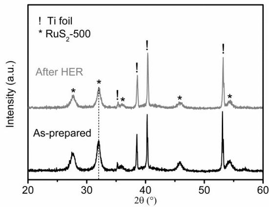
**Fig. S12.** XRD patterns of  $\text{RuS}_2\text{-500}$  loaded on the Ti foil substrate before and after HER for 50 cycles. The XRD patterns show that there is no apparent variation in the peak pattern and position between as-prepared and post-HER  $\text{RuS}_2\text{-500}$ , revealing the unchanged bulk crystal structure of  $\text{RuS}_2\text{-500}$  during HER.
