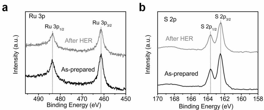
**Fig. S13.** XPS spectra of (a) Ru 3p and (b) S 2p for RuS<sub>2</sub>-500 before and after HER for 50 cycles. XPS spectra of Ru 3p and S 2p show almost no change after HER for 50 cycles.
