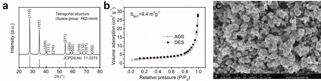
**Fig. S1.** (a) XRD patterns of commercial RuO<sub>2</sub> powder (Sigma-Aldrich). (b) N<sub>2</sub> adsorption-desorption isotherm of RuO<sub>2</sub>. (c) SEM image of RuO<sub>2</sub>.
