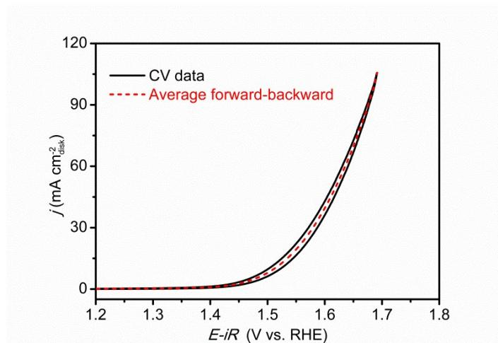
**Fig. S14.** Capacitive correction of the as-measured CV curve ( $10 \text{ mV s}^{-1}$ ) of example catalyst (i.e., RuS<sub>2</sub>-500).
