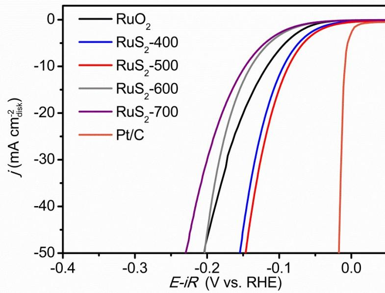
**Fig. S9.** HER polarization curves of  $\text{RuS}_2\text{-T}$ ,  $\text{RuO}_2$  and  $\text{Pt/C}$  catalysts in Ar-saturated 0.5 M  $\text{H}_2\text{SO}_4$  solution. Scan rate, 5 mV s<sup>-1</sup>.
