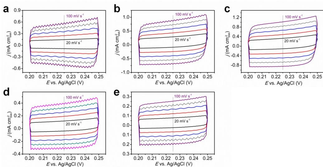
**Fig. S16.** CV measurements in a non-faradic current region (0.2–0.25 V vs. Ag/AgCl) at scan rates of 20, 40, 60, 80 and 100  $\text{mV s}^{-1}$  of (a)  $\text{RuO}_2$ , (b)  $\text{RuS}_2\text{-}400$ , (c)  $\text{RuS}_2\text{-}500$ , (d)  $\text{RuS}_2\text{-}600$  and (e)  $\text{RuS}_2\text{-}700$  catalysts in 1 M KOH solution.
