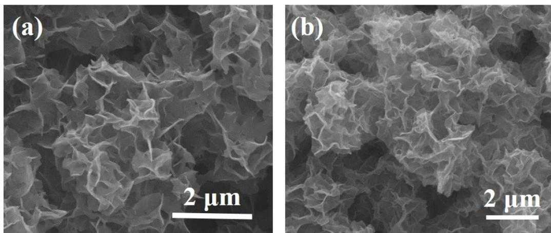
Figure S7 SEM images of the pTTh before (a) and after (b) the aging test.
