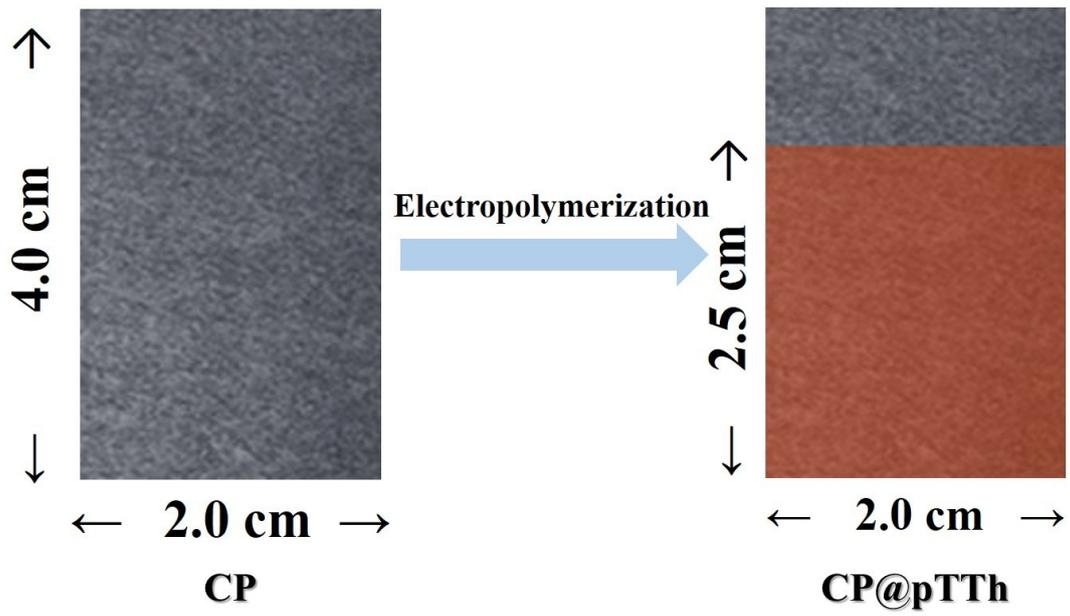
Figure S4 the digital photo of the as-prepared CP@pTTh electrode.
