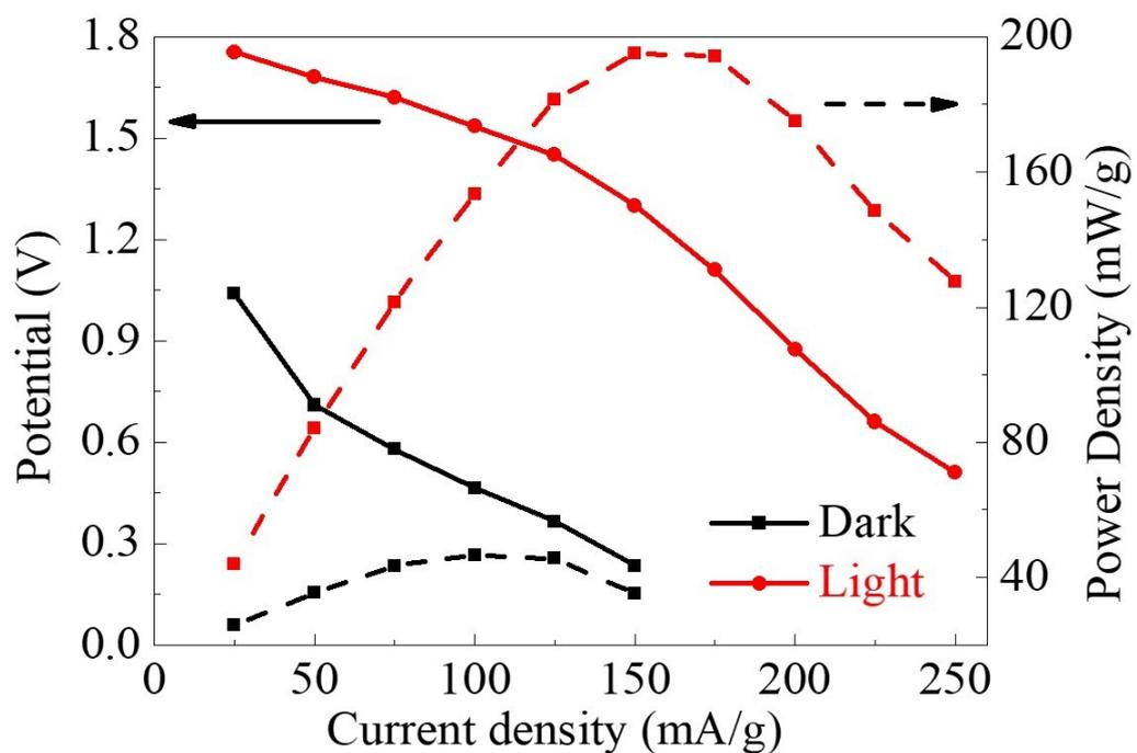
Figure S8 polarization and power density curves of a photo-enhanced Zn-air battery using the CP@pTTh as air electrode (size: 2.0 cm×2.5 cm; mass loading: ~1.3 mg pTTh/cm<sup>2</sup>).
