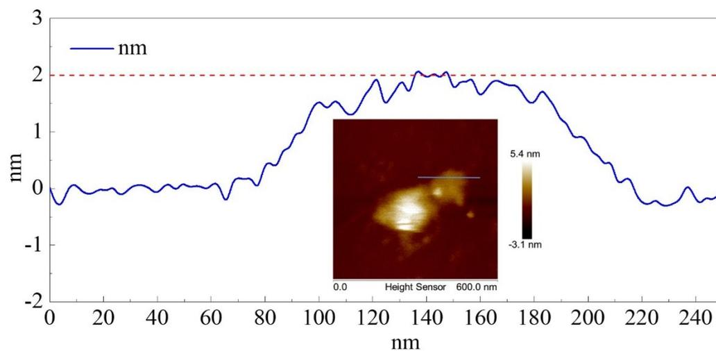
Figure S1 line profiles corresponding to the inset AFM topography image of the pTTh.
