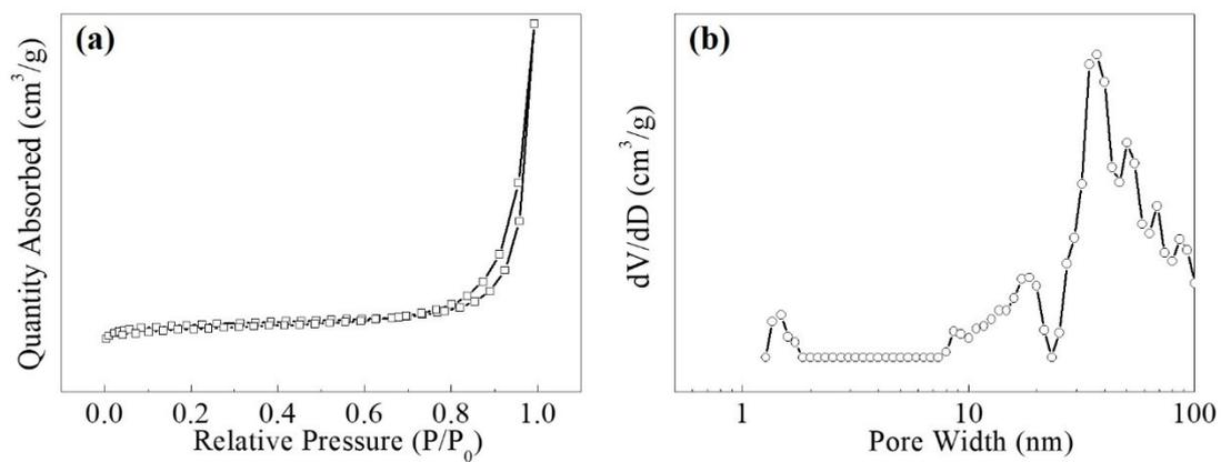
Figure S2 N<sub>2</sub> adsorption-desorption isotherms (a) and the corresponding pore size distribution (b) of the as-prepared pTTh.
