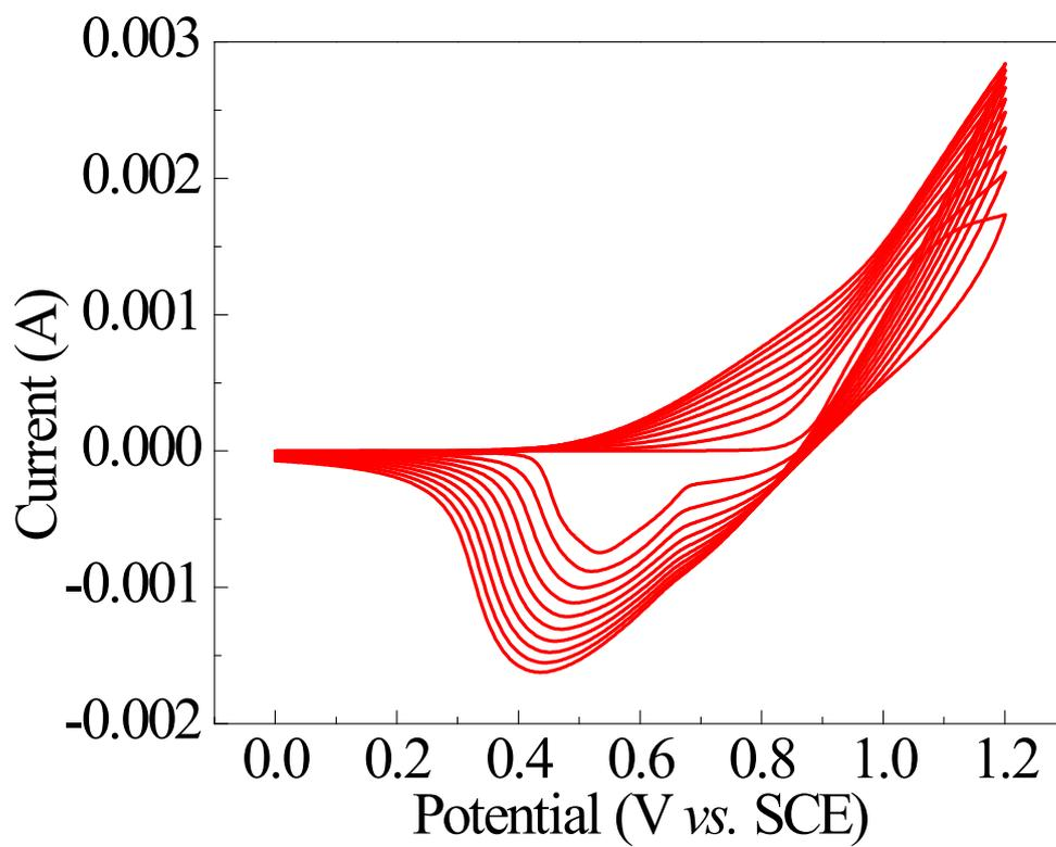
Figure S3 Multicycle cyclic voltammetry electropolymerization of TTh monomer in acetonitrile containing 20 mM monomer and 0.1 M LiClO<sub>4</sub>.
