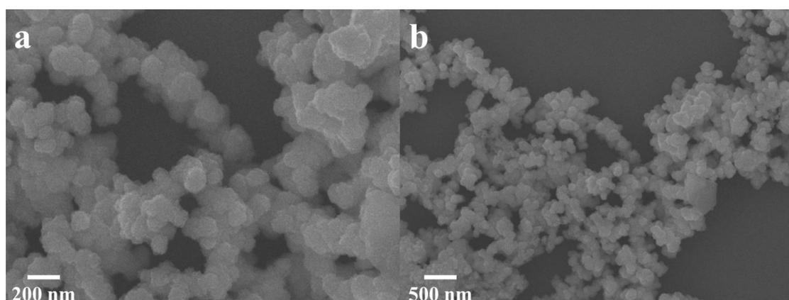
**Figure S5.** SEM images of the O-ReS<sub>2</sub> powder.
