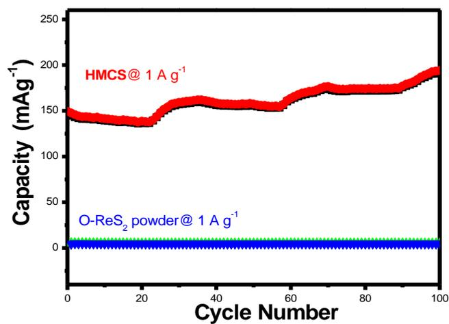
**Figure S13.** Cycling stability of the HMCS and O-ReS<sub>2</sub> powder.
