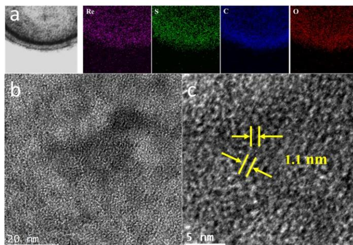
**Figure S14.** (a) EDX mapping and (b, c) HR-TEM images of the cycled O-ReS<sub>2</sub>@HMCS-150 electrode.
