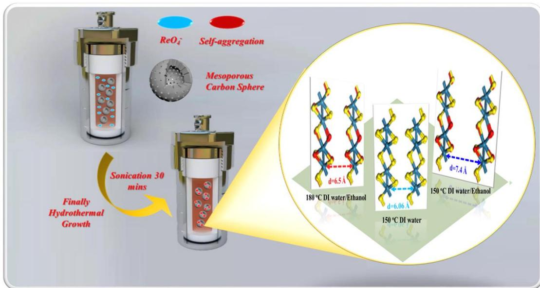
**Figure S2.** Schematic illustration of the synthesis process with expanded interlayer.
