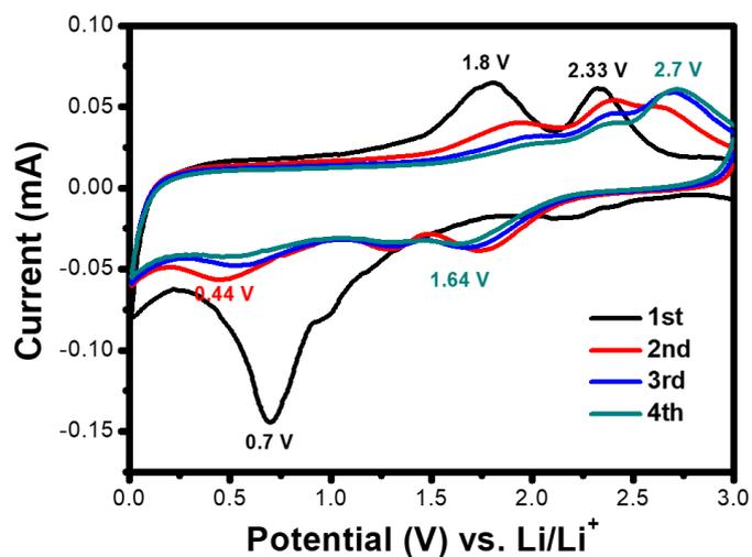
**Figure S12.** CV curves of the O-ReS<sub>2</sub> powder.
