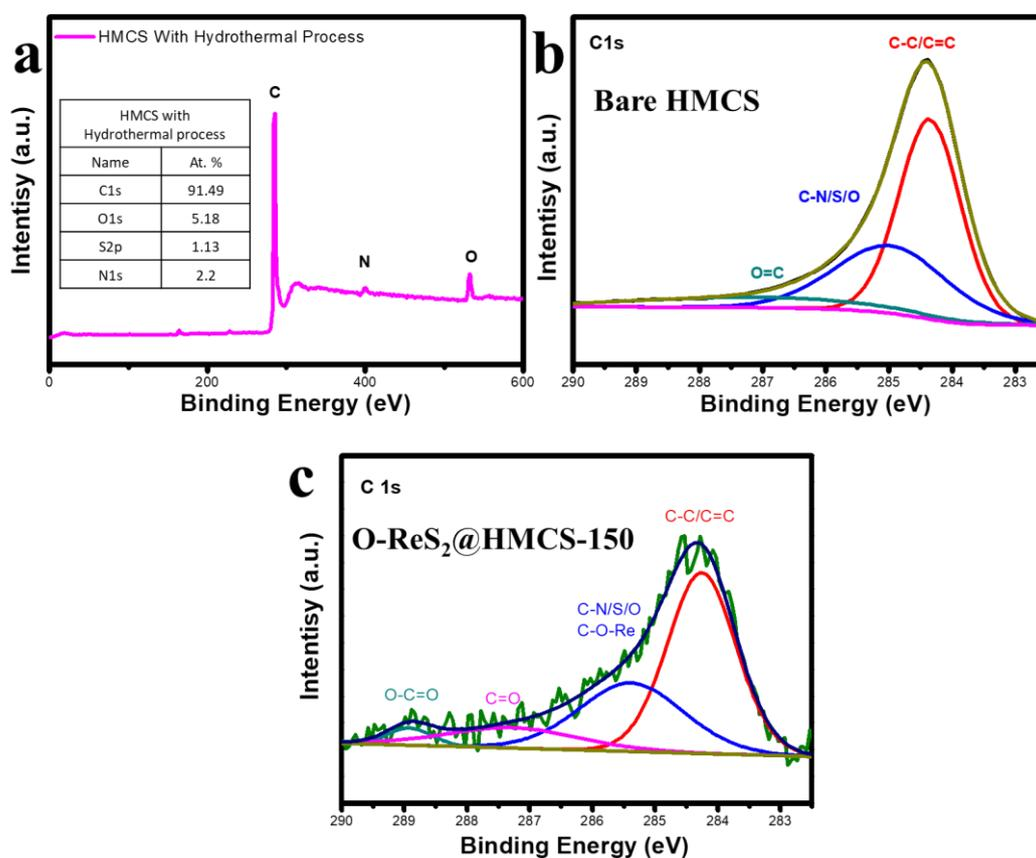
**Figure S9.** (a,b) XPS of the HMCS with same hydrothermal process without the Re-precursors and (c) C1s of the O-ReS<sub>2</sub>@HMCS-150.
