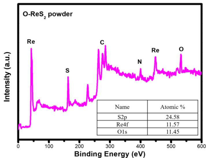
**Figure S10.** XPS of the O-ReS<sub>2</sub> powder with same hydrothermal process without HMCS.
