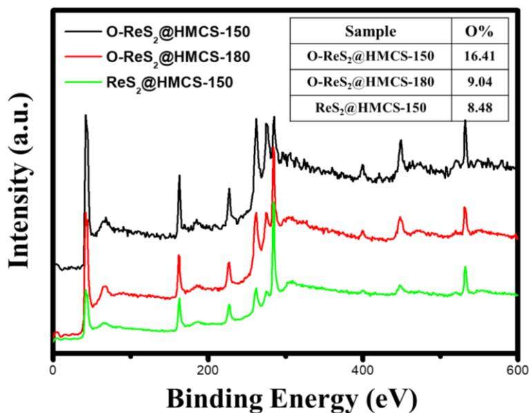
**Figure S8.** XPS data of the composite. Insert table shows the O ratio.
