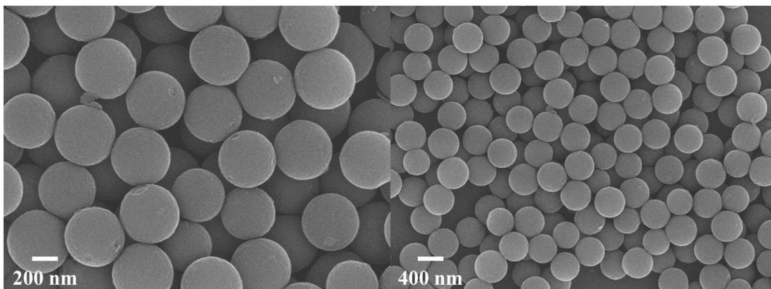
**Figure S1.** SEM images of the SiO<sub>2</sub>@SiO<sub>2</sub>/RF carbon sphere.
