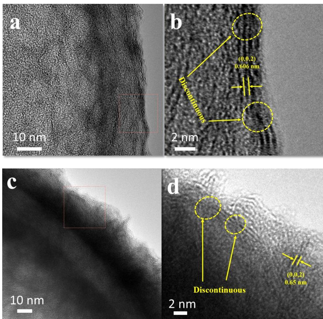
**Figure S7.** (a,b) HR-TEM images of the nanocomposite with only DI water solvent. (c,d) HR-TEM images of the nanocomposite with 180 °C reaction temperature.
