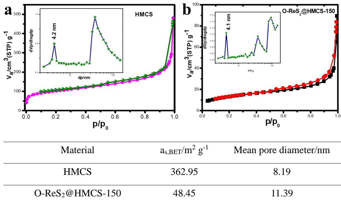
**Figure S11.** N<sub>2</sub> adsorption/desorption isotherms of (a) MHCS and (b) O-ReS<sub>2</sub>@HMCS-150. Insert is the corresponding pore size distribution profile.
