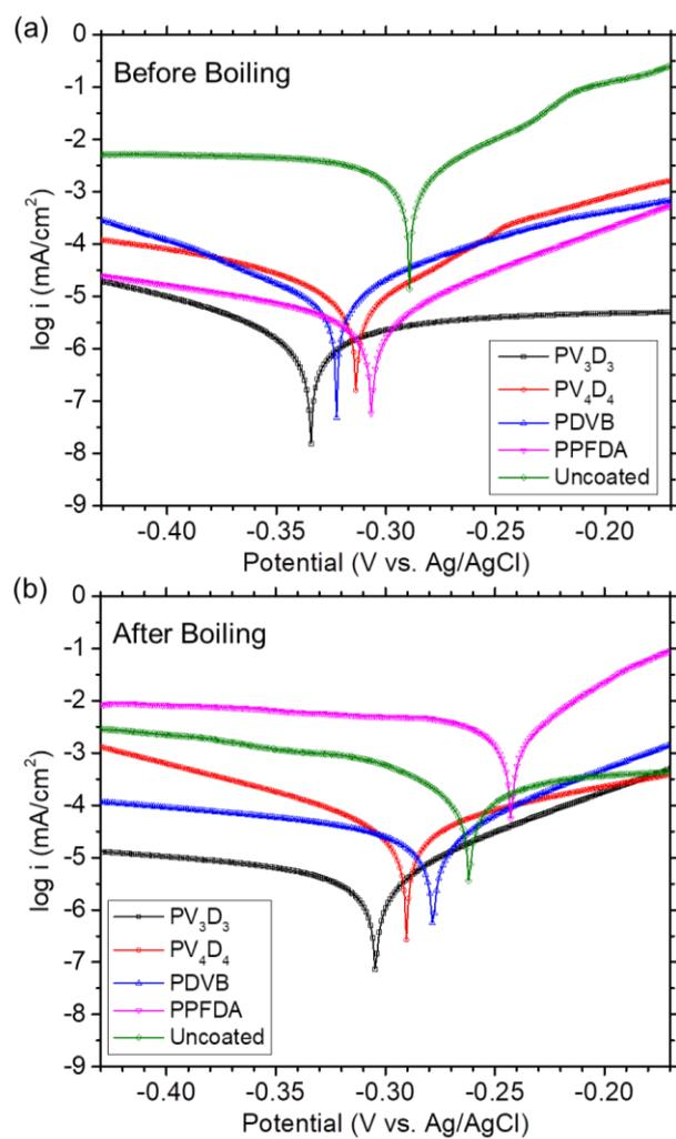
**Figure S6.** Tafel plots for uncoated and iCVD coated Cu/Ni foils before and after exposure to boiling water for 2 h.
