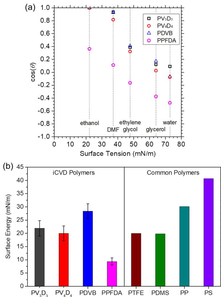
**Figure S4.** (a) Contact angles of liquids with different known surface tension on iCVD polymer surfaces. (b) Calculated surface energy for iCVD polymers and reported surface energy values for common commercial polymers.
