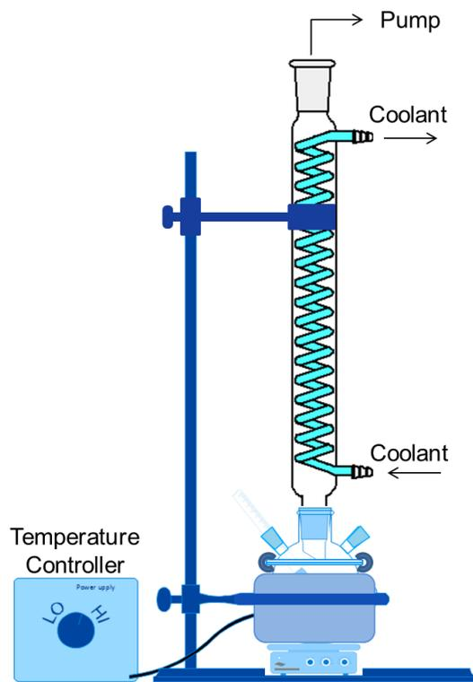
**Scheme S2.** Schematic of the experimental apparatus used for the simulated MSF scaling tests.
