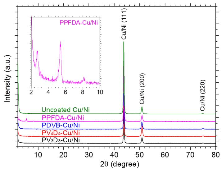
**Figure S1.** Grazing incidence X-ray diffraction (GIXRD) patterns for uncoated Cu/Ni foil and Cu/Ni coated with different iCVD polymers. Inset represents the diffraction peaks for iCVD PPFDA at low  $2\theta$  angles.
