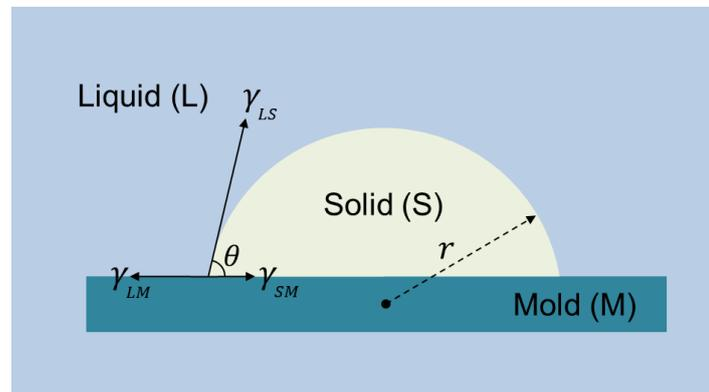
**Scheme S1.** Schematic of heterogeneous nucleation on flat surface
