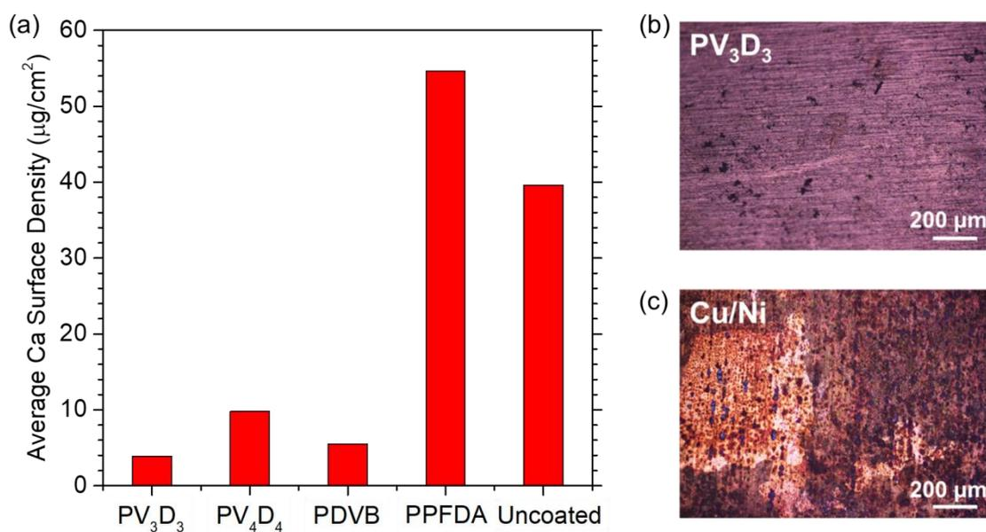
**Figure S7.** (a) Calcium surface density for uncoated and iCVD-coated Cu/Ni after simulated MSF tests for 72 h. (b-c) Optical micrographs for (b) iCVD  $\text{PV}_3\text{D}_3$  coated Cu/Ni after 72 h test, and (c) uncoated Cu/Ni after 72 h tests.
