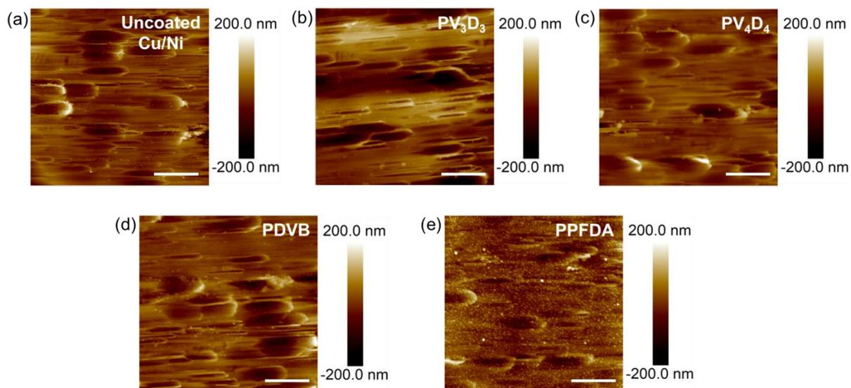
**Figure S2.** Atomic force microscopy (AFM) images for uncoated Cu/Ni foil and Cu/Ni coated with iCVD  $PV_3D_3$ ,  $PV_4D_4$ , PDVB and PPFDA, respectively (Scale bars represent 10  $\mu\text{m}$ ).
