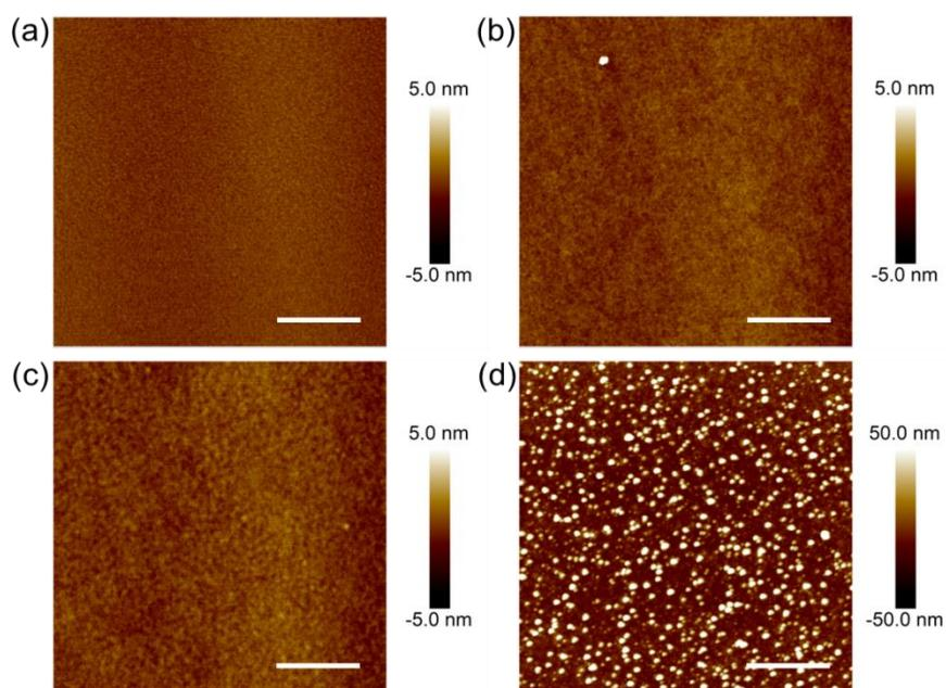
**Figure S3.** AFM images for Si wafers coated with (a) iCVD  $PV_3D_3$ , (b)  $PV_4D_4$ , (c) PDVB and (d) PPFDA, respectively (Scale bars represent 5  $\mu\text{m}$ ).
