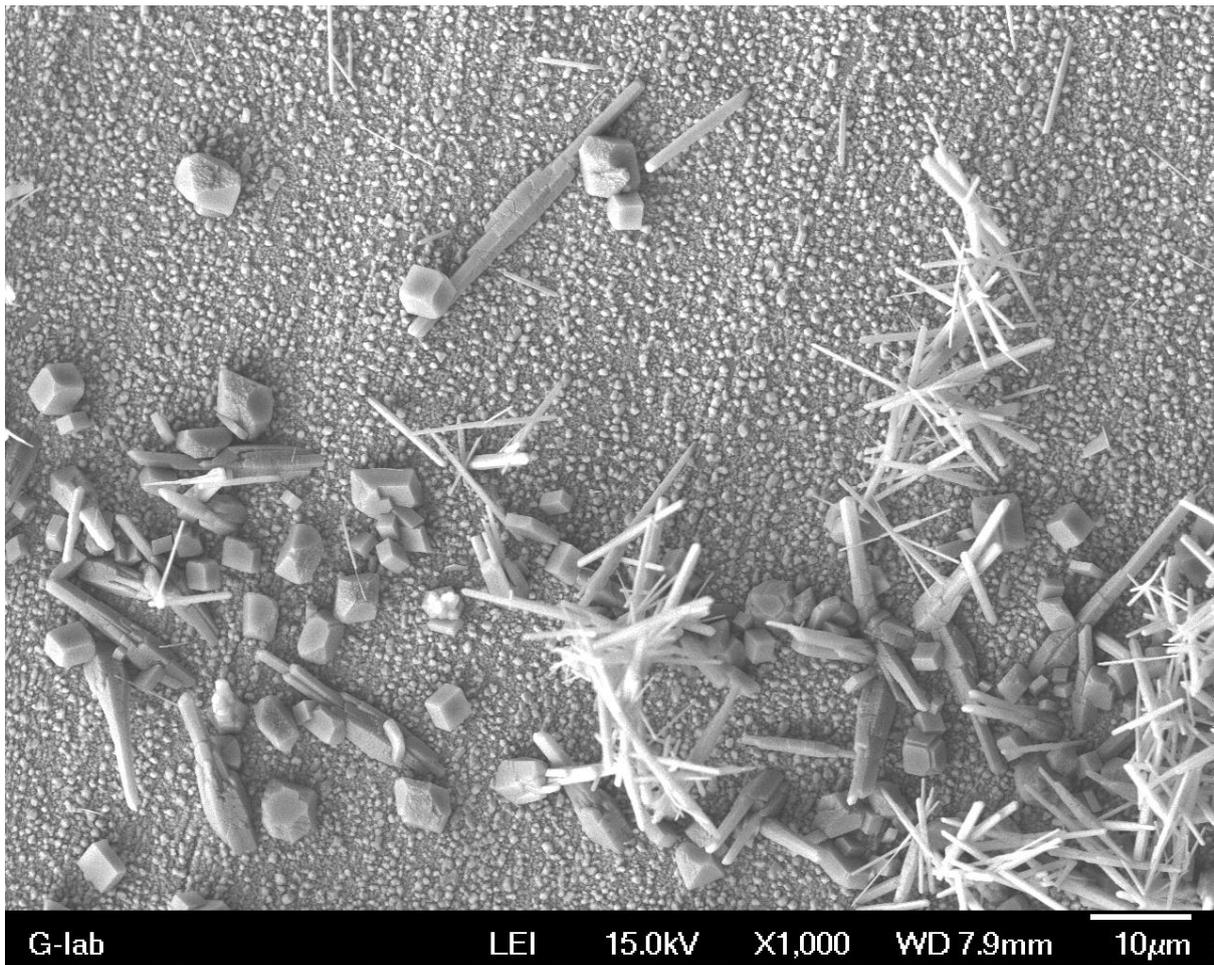
**Figure S5.** SEM image for uncoated and iCVD coated Cu/Ni foil surfaces after CaCO<sub>3</sub> scaling tests at 110 °C.
