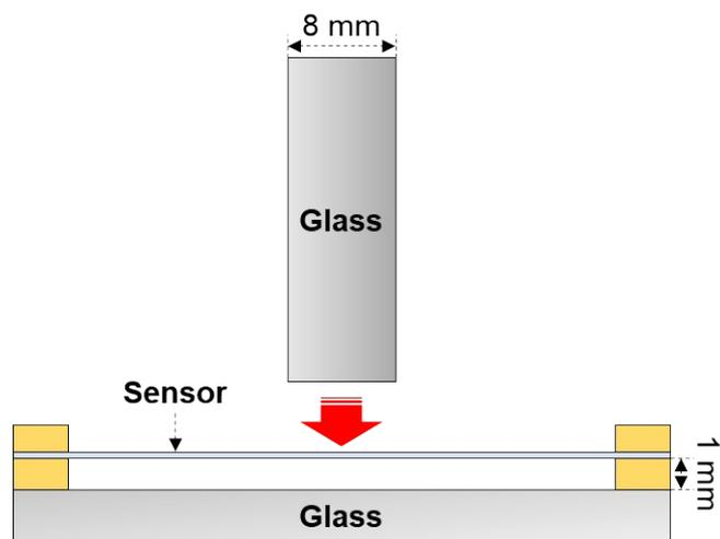
**Fig. S1.** Schematic setup of the pressing test.
