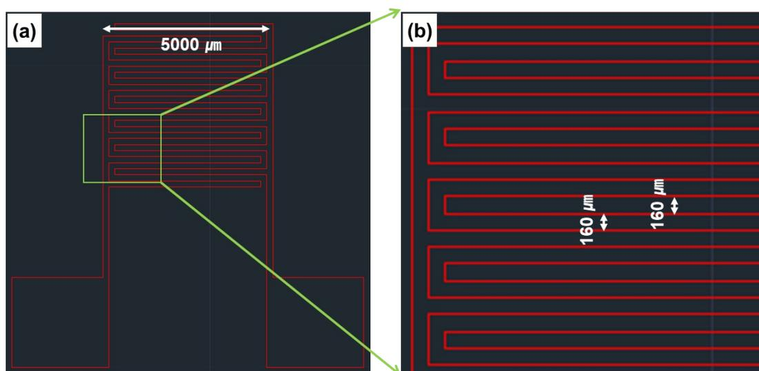
**Fig. S8.** (a) Capacitor design for the pressure sensor and (b) enlarged view of the boxed region in (a).
