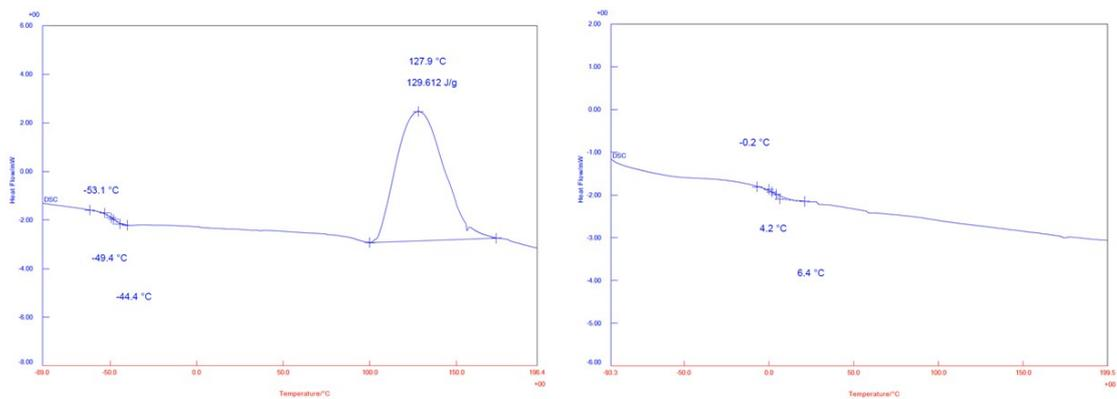
**Fig. S5.** DSC curves for polyurethane acrylate **2** during (left) the first heating cycle and (right) second heating cycle.
