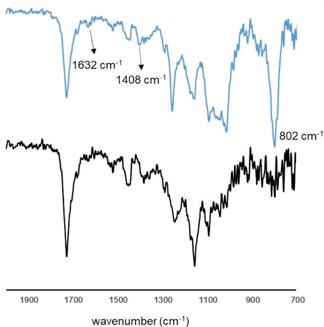
**Fig. S7.** FTIR spectra of the UVC-PSA tape (top) before and (bottom) after UV treatment.
