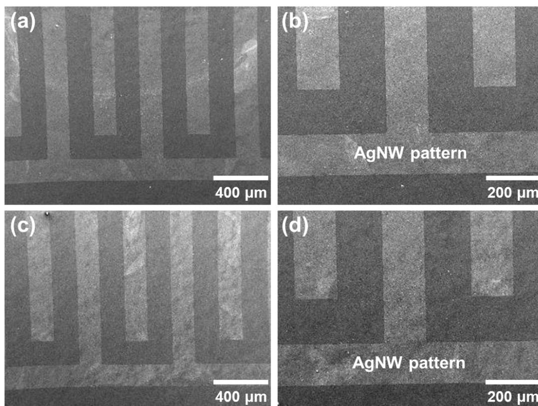
**Fig. S9.** (a), (b) AgNW circuits patterned according to a tandem compound electrode on a 1.4- $\mu\text{m}$ -thick PET before peeling from a carrier substrate. (c), (d) Those after peeling from the carrier with UV irradiation.
