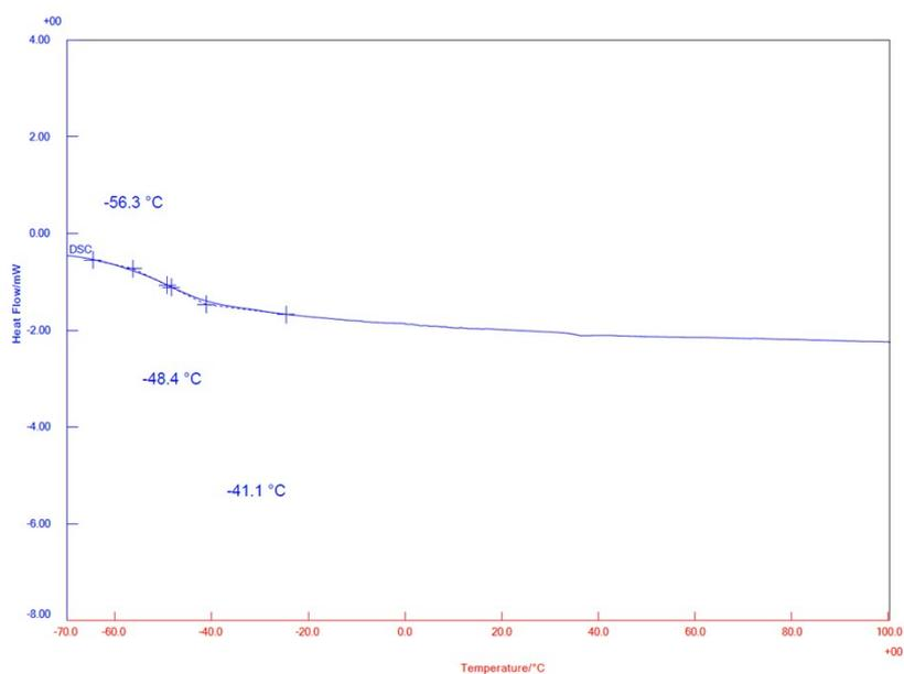
**Fig. S3.** DSC curve for acrylic polymer **1** measured in the range -70 °C to 100 °C.
