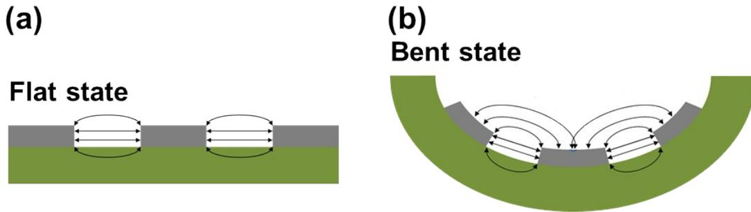
**Fig. S10.** Description of electromagnetic coupling between AgNW-based lines at (a) flat state and (b) bent state.
