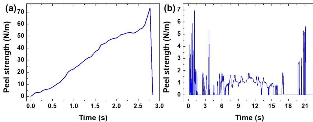
**Fig. S6.** Strength-time curves of UVC-PSA tapes obtained with loop tack test (left) before and (right) after UV irradiation.
