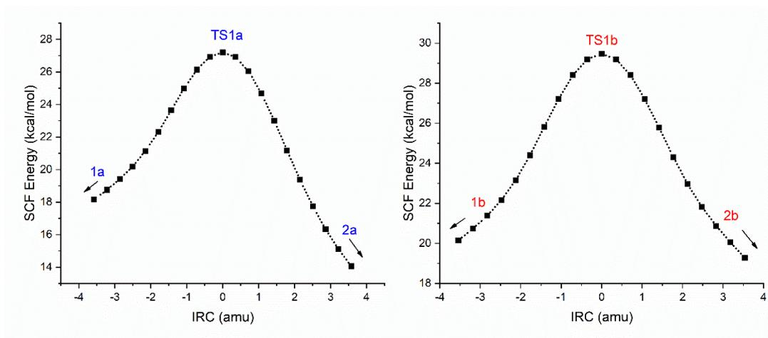
Figure S7.3. IRC from **TS1a** (left) and **TS1b** (right) connecting reactants and products.
