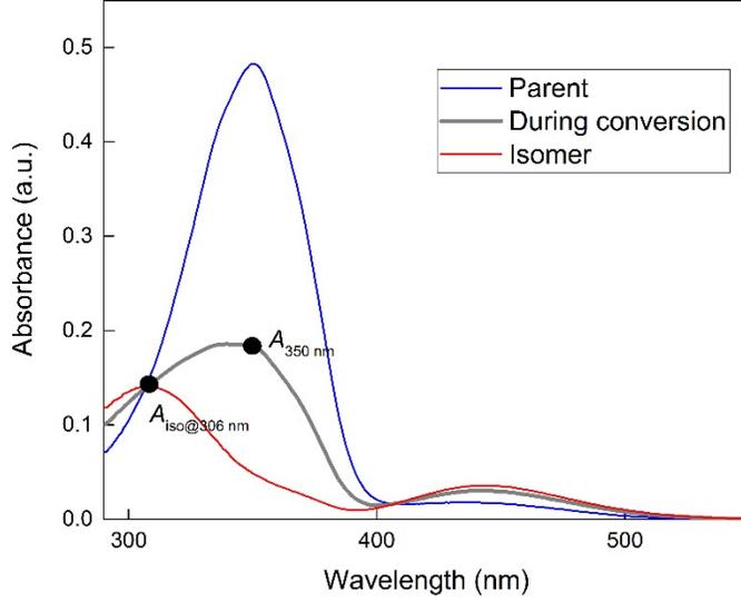
Figure S4.1. **AZO1** spectrum changes over conversion process. Blue curve shows the pure *trans* state, red curve shows the converted *cis* form. Grey curve represents a spectra taken during conversion.  $A_{350\text{ nm}}$  is the absorbance at 350 nm during conversion.  $A_{\text{iso}@306\text{ nm}}$  corresponds to the absorbance at the isosbestic point at 306 nm.
