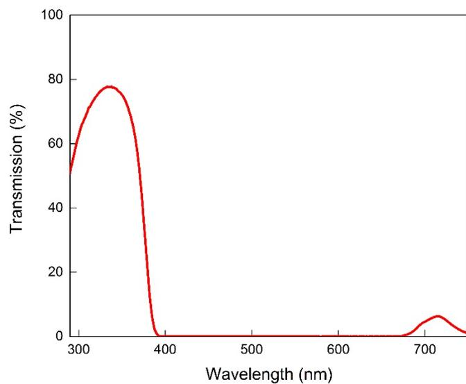
Figure S1.2. Transmission spectrum of UG11 band pass filter with a thickness of 1 mm from SCHOTT
