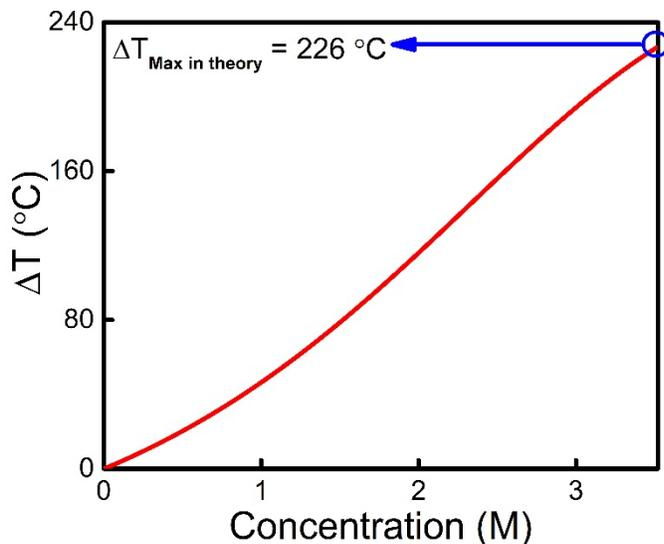
Figure S7.1. Theoretical heat release simulation in function of concentration of **AZO1**, a maximum  $\Delta T$  of 226 °C can be achieved with neat **AZO1-cis** sample.
