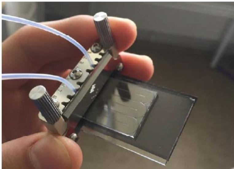
Figure S1.2. Actual photo of the microfluidic chip.
