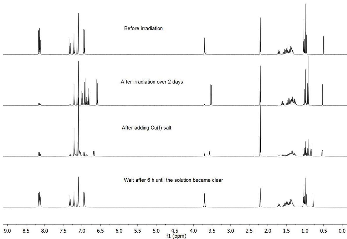
Figure S7.4.  $^1\text{H}$  NMR studies of **AZO-cis** in  $\text{toluene-d}_8$  solution with  $[\text{Cu}(\text{CH}_3\text{CN})_4]\text{PF}_6$ .
