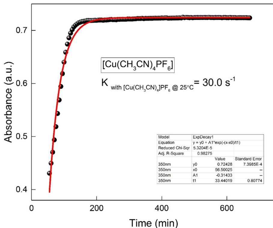
Figure S7.3. Catalytic back conversion of **AZO-cis** in toluene solution with  $[\text{Cu}(\text{CH}_3\text{CN})_4]\text{PF}_6$ .
