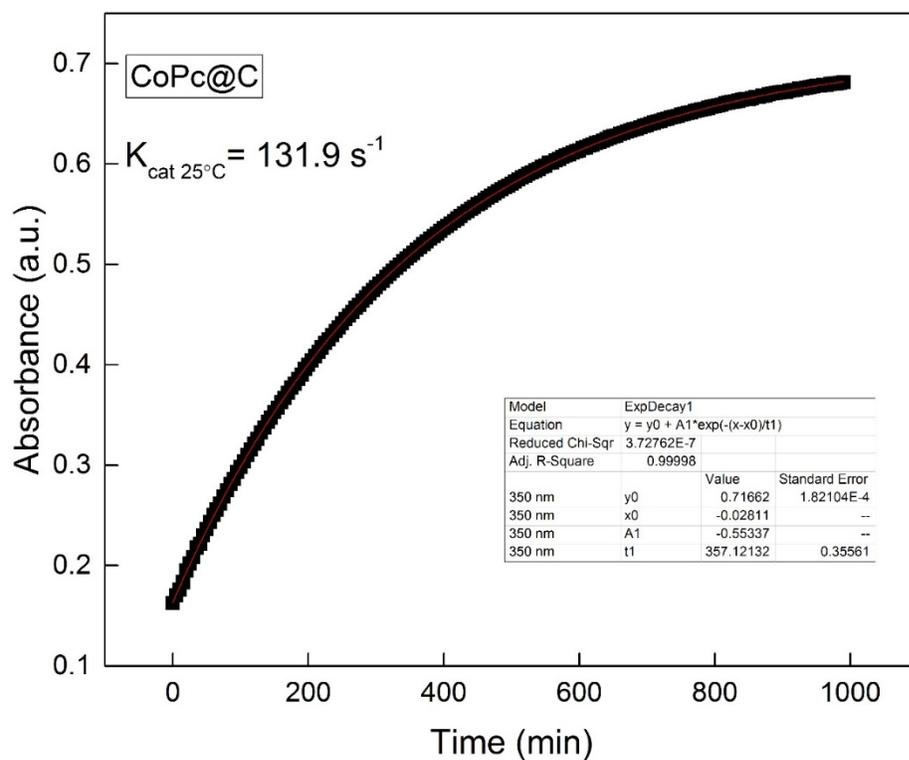
Figure S7.2. Catalytic back conversion of **AZO-cis** in toluene solution with CoPc@C.
