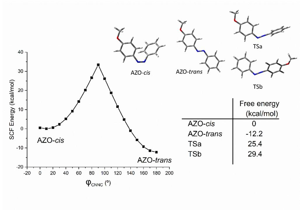
Figure S7.1. Scan along the CNNC dihedral torsion. Free energies for *free-AZO* critical points.
