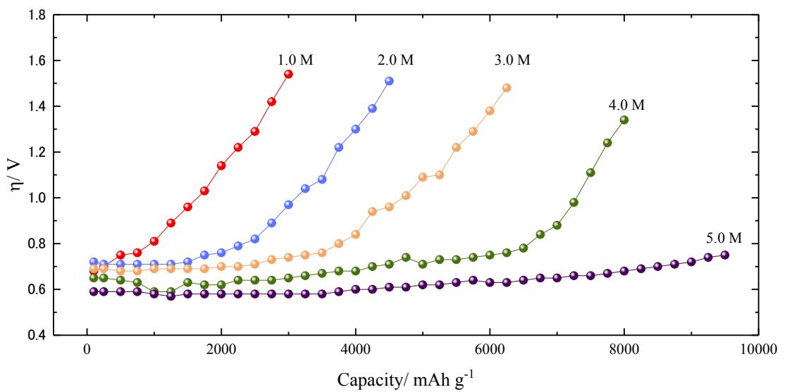
**Fig. S2.** Charge overpotential as a function of capacities for different concentration  $\text{LiNO}_3$  in  $\text{Li-O}_2$  batteries
