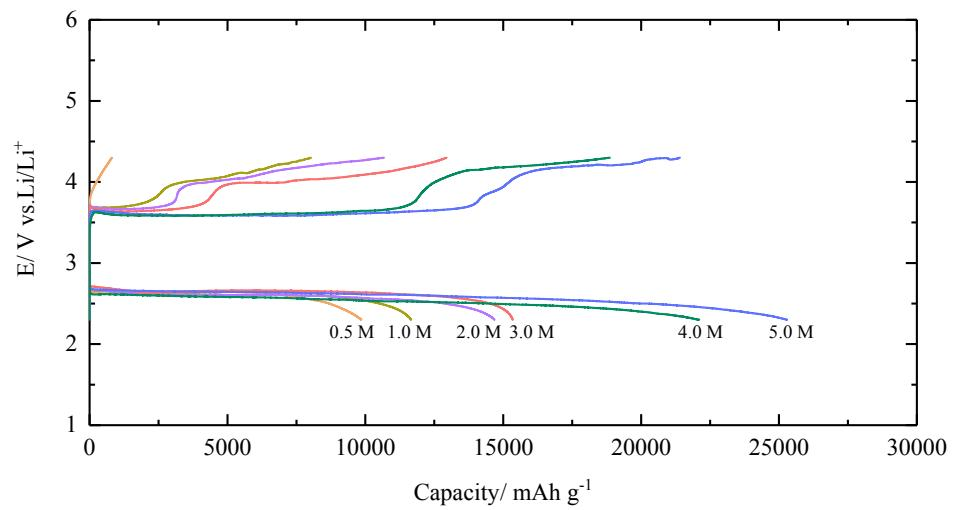
**Fig. S1.** Full discharge-charge profile as a function of different concentration LiNO<sub>3</sub> in Li-O<sub>2</sub> batteries at a current density of 500 mA g<sup>-1</sup> and a cut-off voltage window from 2.3 to 4.5 V vs.Li/Li<sup>+</sup>
