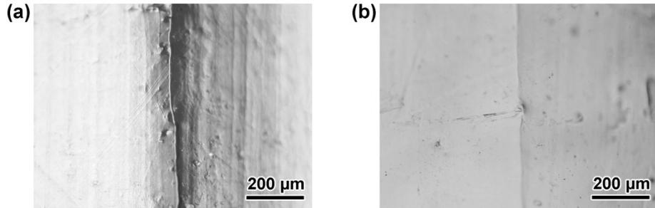
**Fig. S9** Microscope images of the cut Zn<sup>2+</sup>/POA-His films after healing for (a) 10 s and (b) 1 h.
