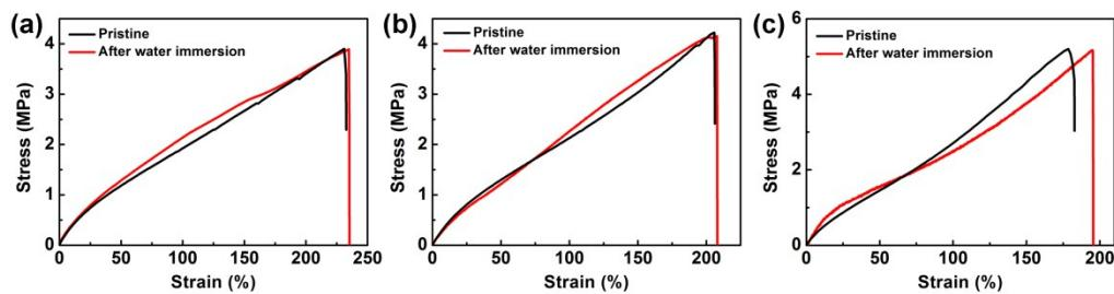
**Fig. S8** Stress-strain curves of (a)  $Zn^{2+}$ /POA-His, (b)  $Cu^{2+}$ /POA-His and (c)  $Fe^{3+}$ /POA-His films before and after immersion in water.
