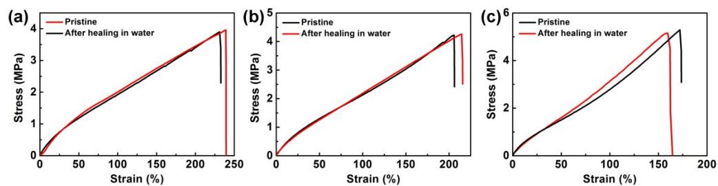
**Fig. S10** Stress-strain curves of (a) Zn<sup>2+</sup>/POA-His, (b) Cu<sup>2+</sup>/POA-His and (c) Fe<sup>3+</sup>/POA-His films and the cut films after healing in water.
