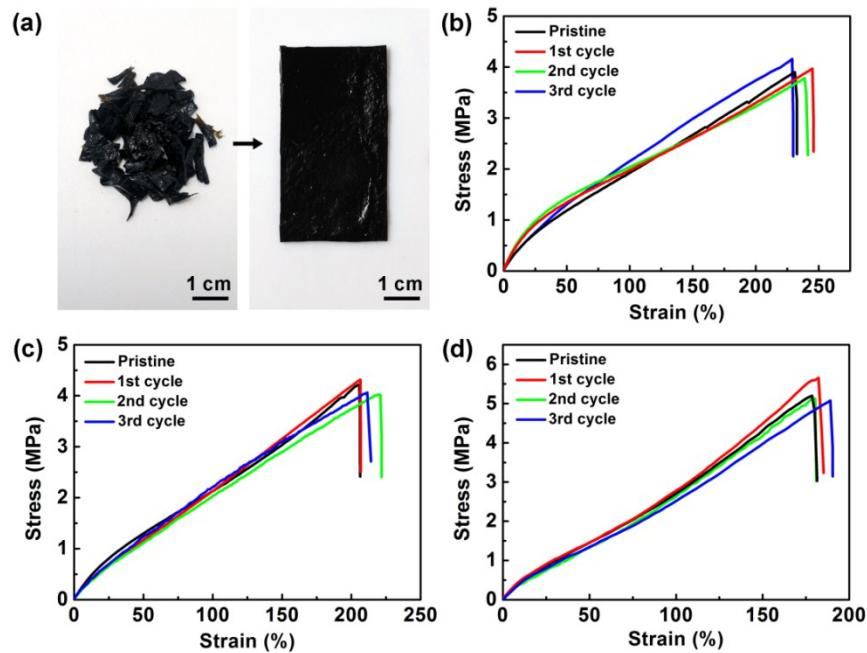
**Fig. S11** (a) Recycling test of  $\text{Fe}^{3+}$ /POA-His film. (b-d) Stress-strain curves of (b)  $\text{Zn}^{2+}$ /POA-His, (c)  $\text{Cu}^{2+}$ /POA-His and (d)  $\text{Fe}^{3+}$ /POA-His films after different cycles of recycling process.
