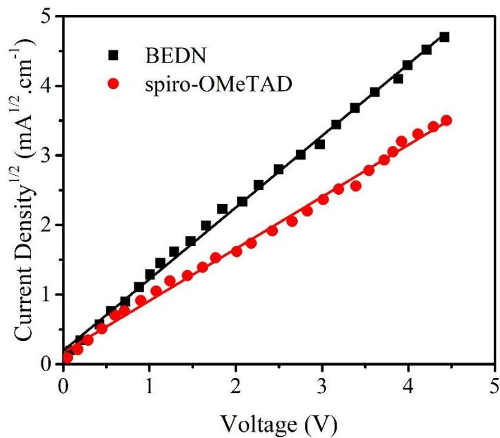
**Figure S7.**  $J^{1/2}$ -V curves of dopant-free BEDN and spiro-OMeTAD based devices with a architecture of ITO/PEDOT:PSS/HTMs/Au.
