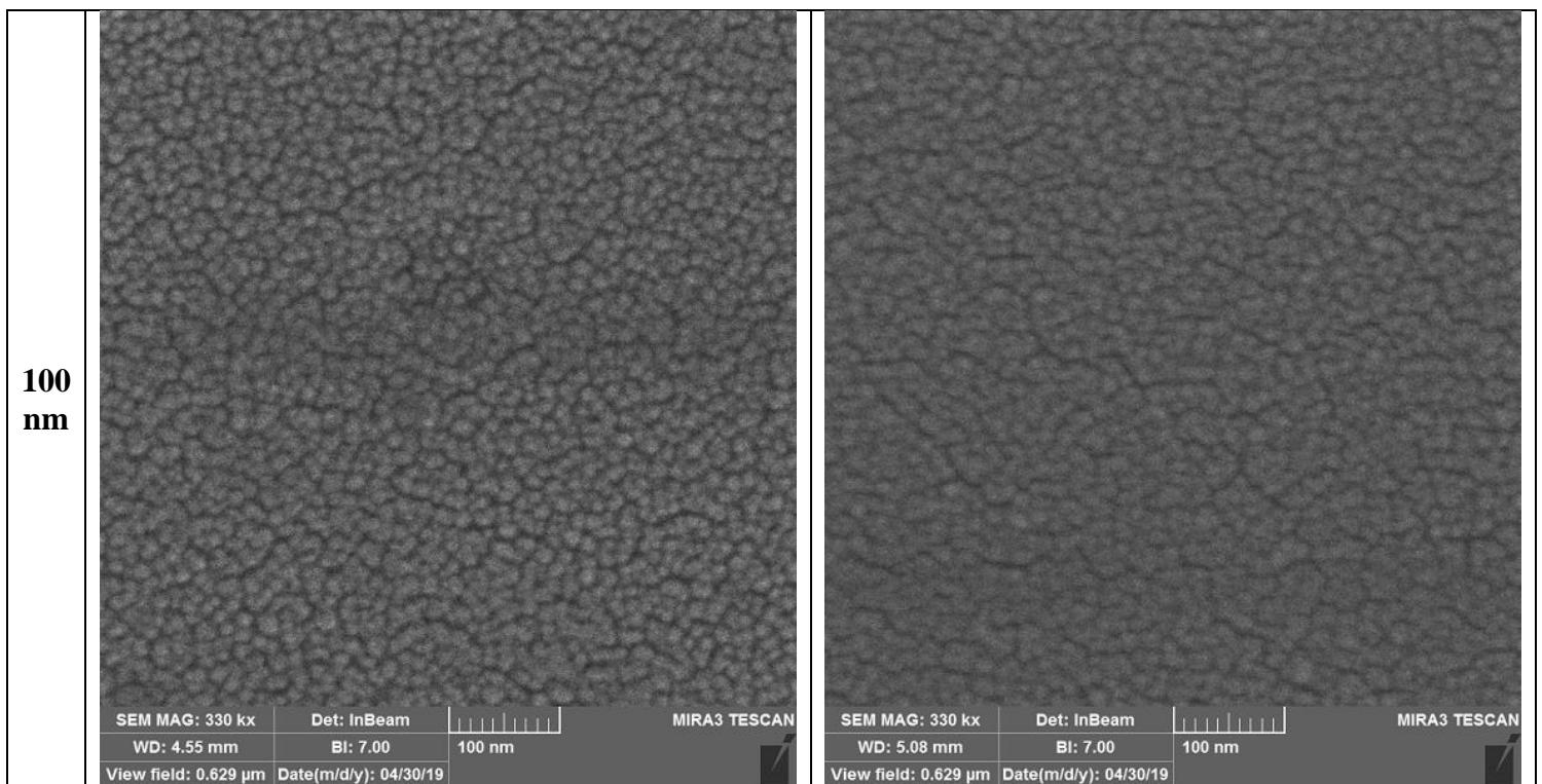
**Figure S3.** FE-SEM images of the top view of the cells with structures Glass/spiro-OMeTAD (left) and Glass/ BEDN (right).
