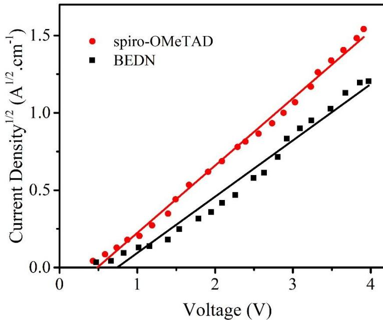
**Figure S8.**  $J^{1/2}$ -V curves of BEDN and spiro-OMeTAD based devices with a architecture of ITO/PEDOT:PSS/HTMs:Dopants/Au.
