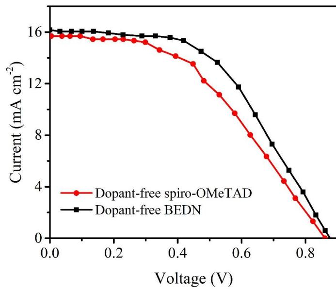
**Figure S6.** J-V curves of PSCs based on dopant-free BEDN and dopant-free spiro-OMeTAD HTMs.
