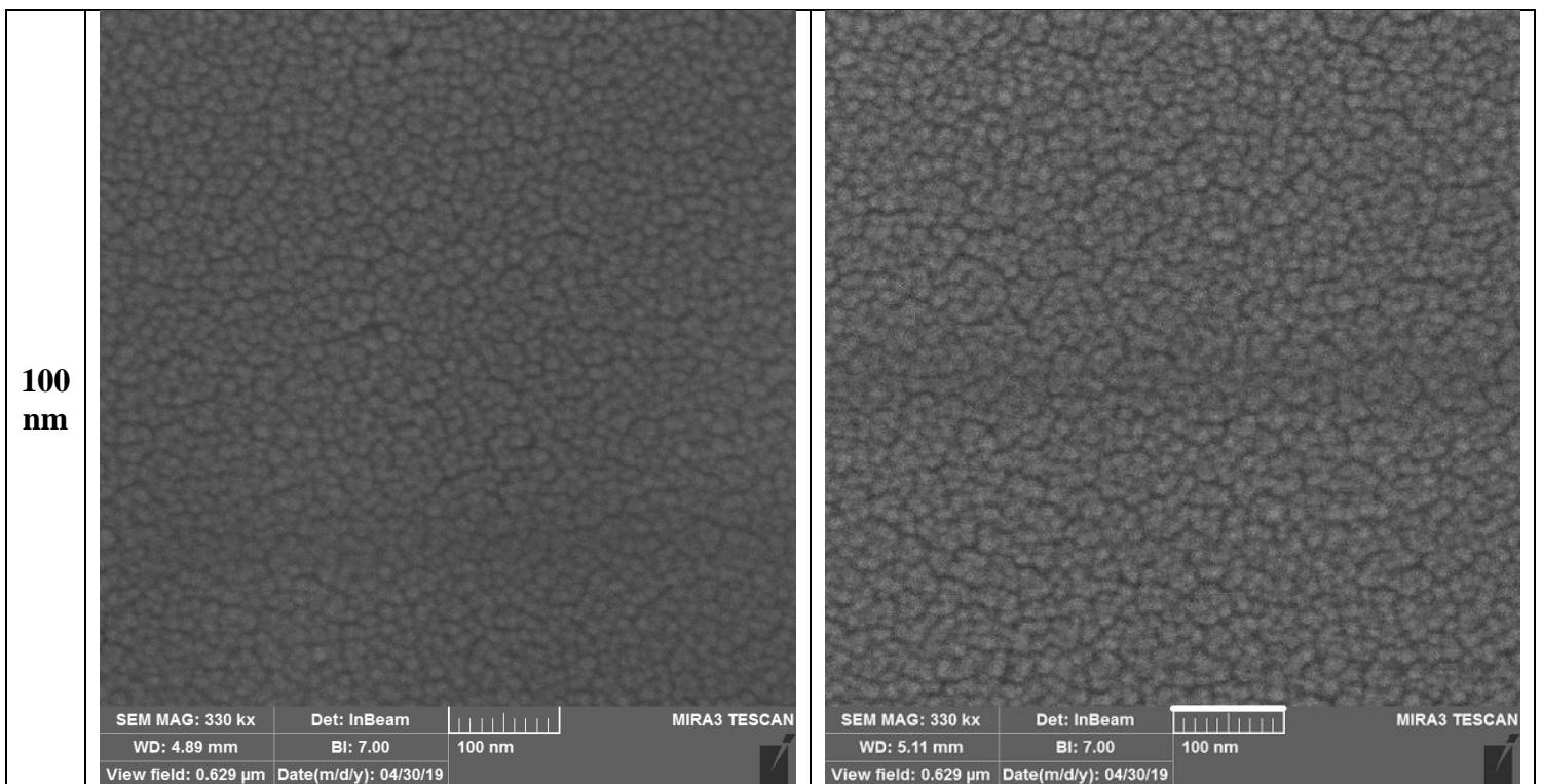
**Figure S4.** FE-SEM images of the top view of the cells with structure Glass/meso-TiO<sub>2</sub>/spiro-OMeTAD (left) and Glass/meso-TiO<sub>2</sub>/BEDN (right) .
