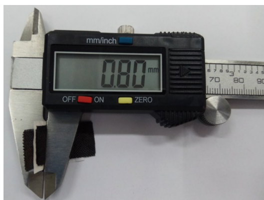
Figure S10: The digital photograph of thickness measurements for ZCS-NC//MPC-ASC (including gelectrodes, ausi-solid-state gel electrolyte and separator).
