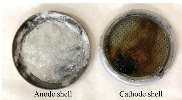
**Figure S3.** Photographs of coin shells after 1000 cycles, showing heavy corrosion in the positive electrode shell.
