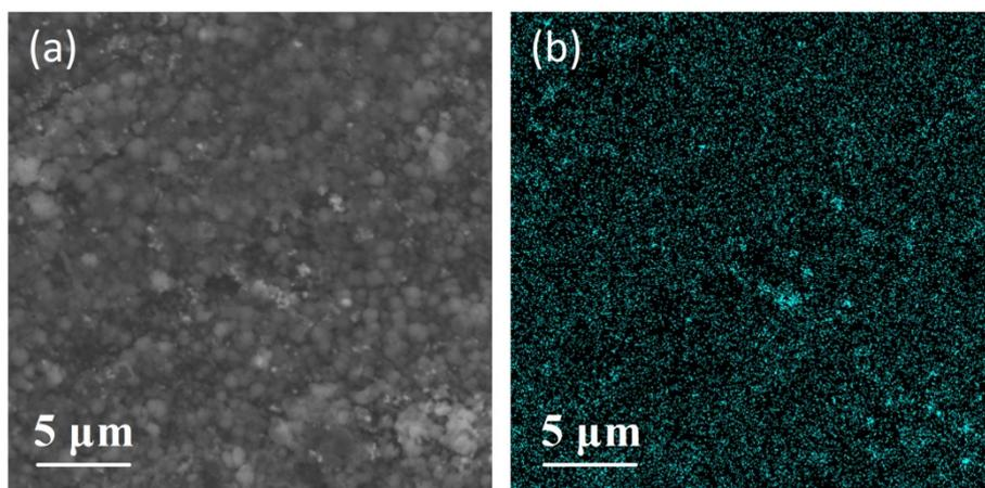
**Figure S7.** a) SEM image of Ag/Li anodes after 500 cycles ( $5\text{mA cm}^{-2}$ , completely stripping). b) Corresponding EDS mapping of Ag.
