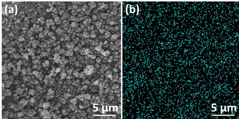
**Figure S1.** a) SEM image of SSNs before cycling, b) Corresponding EDS mapping of Ag.
