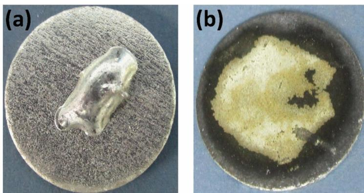
**Figure S5.** Lithiophilicity experiments of a) bare Li anode and b) Ag/Li anodes with molten Li.
