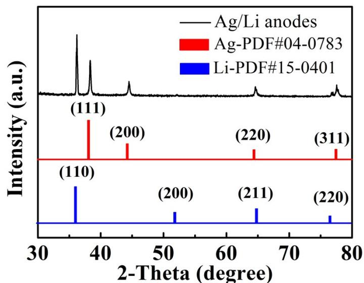
**Figure S2.** XRD patterns of Ag modified Li anodes before cycling.
