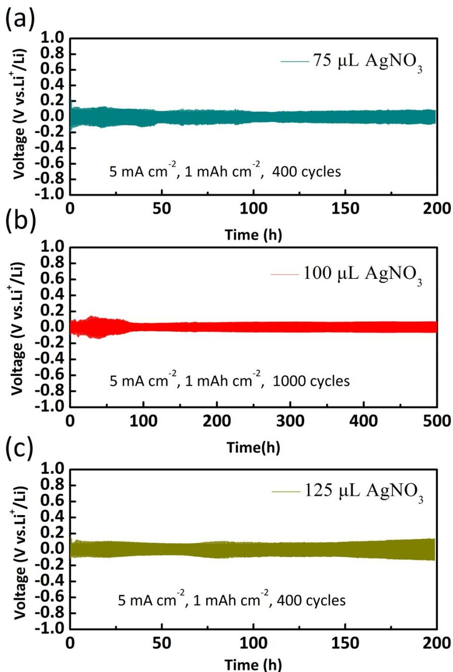
**Figure S4.** Voltage profiles of Ag/Li symmetric cells dropped with various volumes of silver nitrate solution at  $5 \text{ mA cm}^{-2}$  with  $1 \text{ mAh cm}^{-2}$ .
