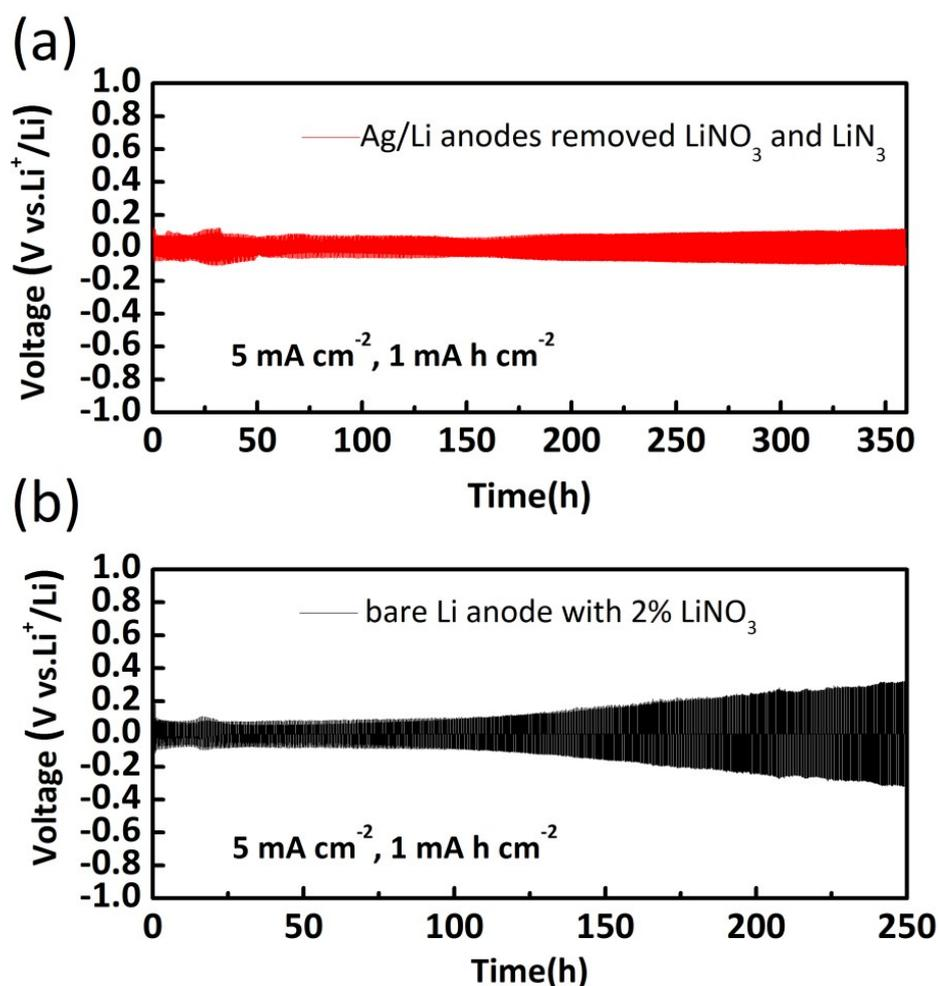
**Figure S8.** a) Voltage profile of Ag/Li symmetric cells removed the generated LiNO<sub>3</sub> and LiN<sub>3</sub>. b) Voltage profile of bare Li symmetric cells with 2 % LiNO<sub>3</sub>.
