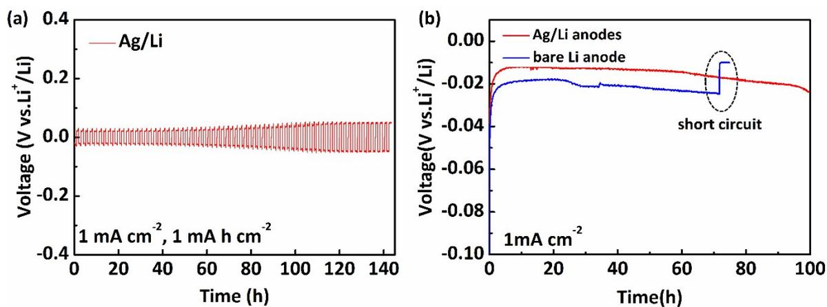
**Figure S6.** a) Voltage profile of reassembled Ag/Li symmetric cell after 1000 cycles. b) Galvanostatic discharge tests of Ag/Li symmetric cell (red) and bare Li symmetric cell (blue) at 1 mA cm<sup>-2</sup>.
