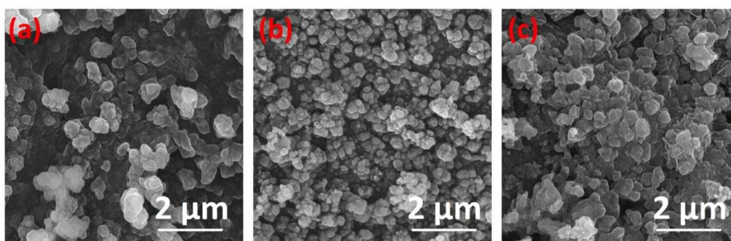
**Figure S3.** SEM images of SSNs with a) 75  $\mu\text{L}$ , b) 100  $\mu\text{L}$  and c) 125  $\mu\text{L}$  silver nitrate solution.
