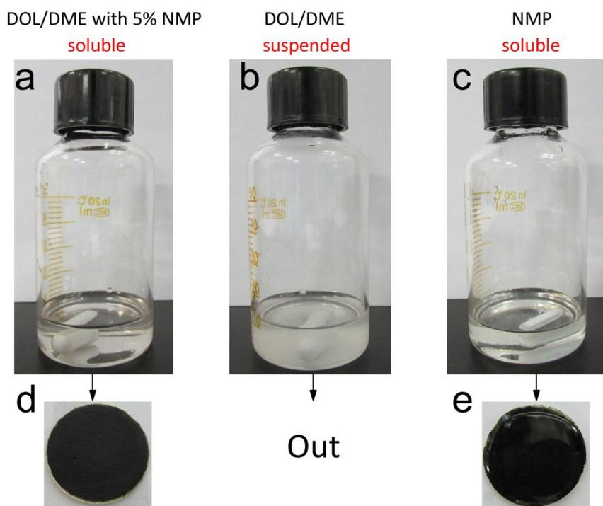
**Figure S9.** a-c: the camera images of silver nitrate in various solvents. d-e: Li foils with 100  $\mu$ L of silver nitrate solution (0.05 mol L<sup>-1</sup>) after 1 hour. The Li foil dripped with DOL/DME With 5% NMP has dried out, but the Li foils with pure NMP are still wet. These images indicate DOL/DME With 5% NMP is most suitable. Since in this solvent system, the silver nitrate can be soluble and rapidly evaporated.
