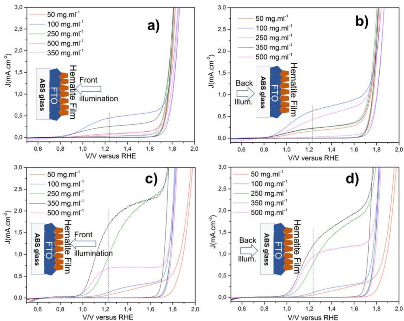
**Figure S6** - Current density,  $J$ , against Voltage,  $V_{RHE}$ , curves for (a and b) unmodified, and (c and d) Sb-hematite films with different thickness measured under dark and simulated sunlight irradiation at front side and back side, respectively.
