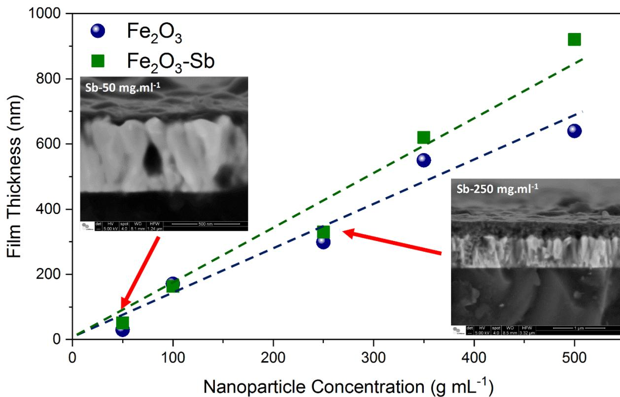
**Figure S5** - Variation of the pure and Sb-hematite film thickness as a function of the magnetite nanoparticle concentration in the colloidal solution. The insets show SEM images of Sb-hematite films.
