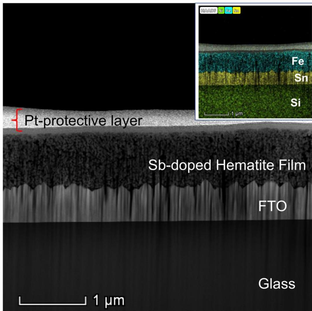
**Figure S3.** HAADF-STEM image of the cross-section analysis of the Sb-hematite film sintered at 850°C. The inset shows the EDS maps of the same region.
