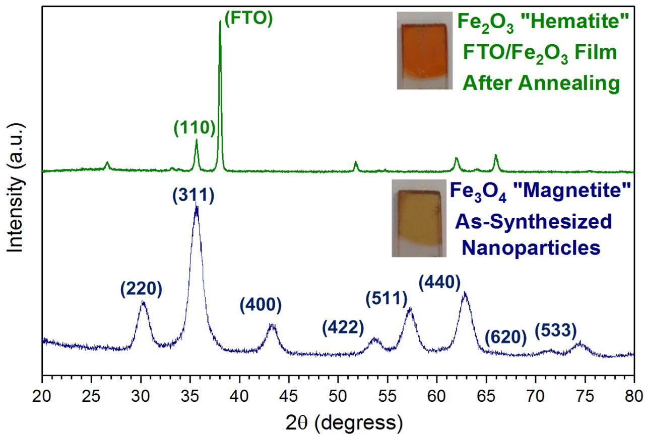
**Figure S2.** X-ray diffraction pattern of the hematite (Fe<sub>2</sub>O<sub>3</sub>) thin films deposited over FTO substrate along with the pattern of the as-synthesized magnetite (Fe<sub>3</sub>O<sub>4</sub>) nanoparticles. The inset photographs show the FTO films before and after phase transformation from magnetite to hematite at 850°C.
