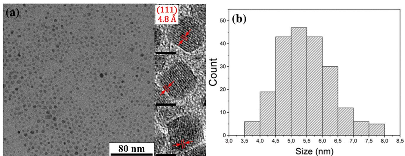
**Figure S4.** Magnetite nanoparticle characterization: (a) Low magnification TEM image of the magnetite nanoparticles used in this work along with HRTEM images showing the (111) lattice fringes with  $d_{hkl}$  equal 4.8 Å, the scale bars have 5 nm; b) Particle size distributions obtained from the TEM analysis.
