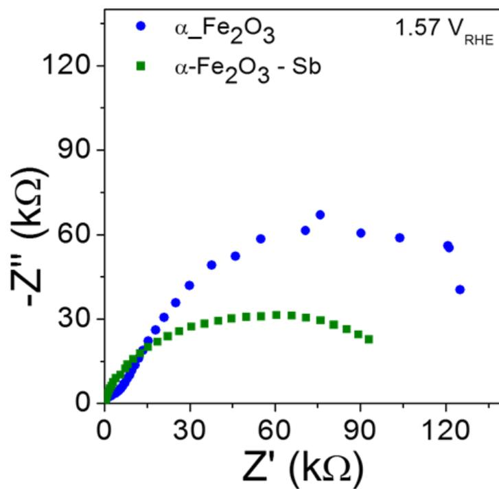
**Figure S9.** Electrochemical impedance spectra (EIS) obtained for unmodified (blue) and Sb-Hematite (green) films electrode in a 1.0 mol L<sup>-1</sup> NaOH solution.
