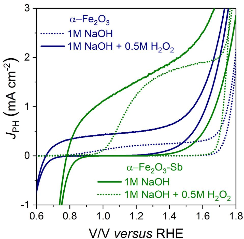
**Figure S8.**  $J_{PH} \times V$  curves in darkness and under illumination for the unmodified hematite and Sb-hematite film in 1M NaOH electrolyte with and without 0.5M  $\text{H}_2\text{O}_2$ .
