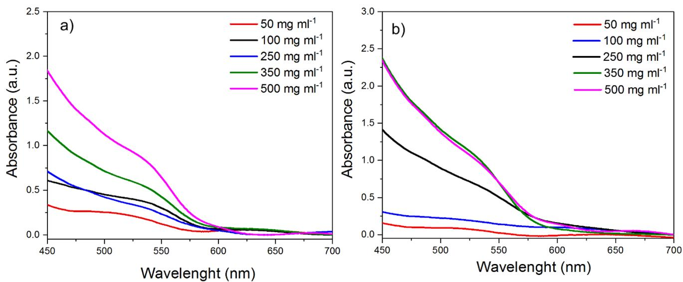
**Figure S7.** UV-Vis spectra of hematite films deposited with different nanoparticle concentration in colloidal solution (from 50 to 500 mg ml<sup>-1</sup>): a) hematite and b) Sb- hematite film.
