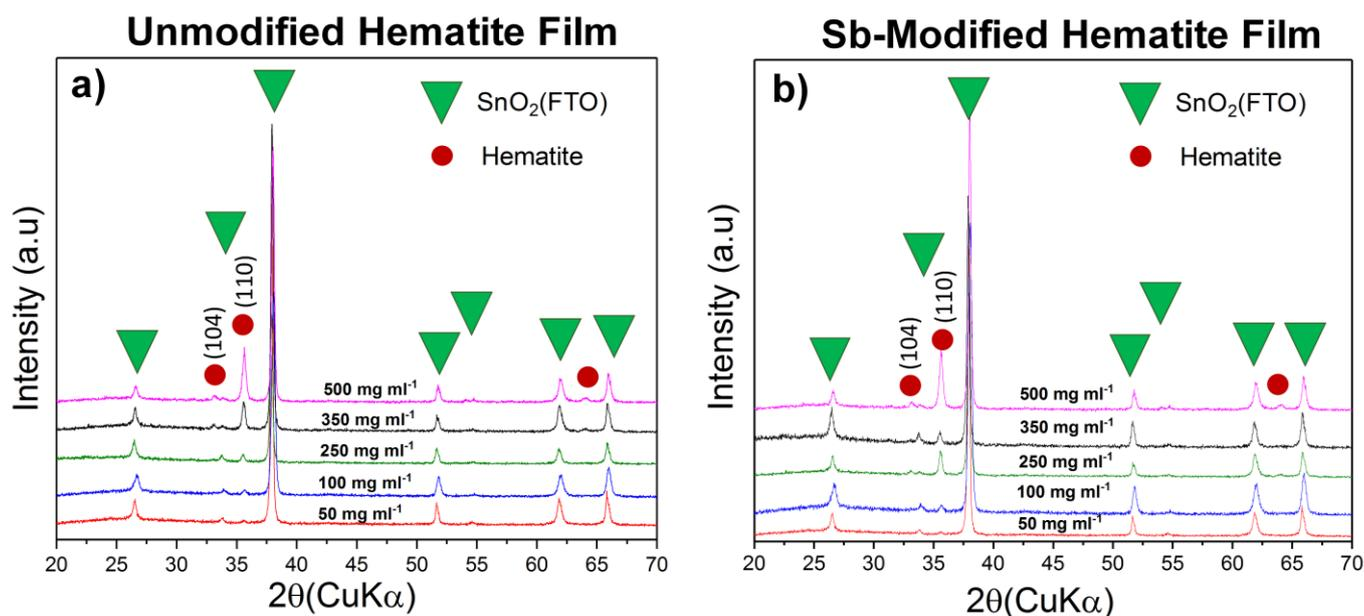
**Figure S1.** X-ray diffraction patterns of the hematite thin films deposited with different concentrations of the colloidal solution (50 to 500 mg.ml<sup>-1</sup>): a) unmodified Hematite film; b) Sb-modified hematite film.
