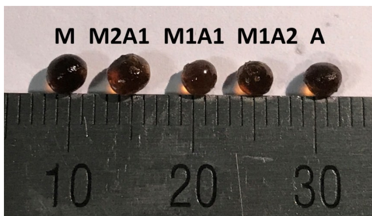
Figure S3. The digital photos of the five kinds of hydrogel spheres with different molar ratios of monomers fabricated by this strategy. The wet hydrogel spheres maintained good sphericity after cross-linking reaction and the average diameter of them were 3.06, 3.04, 2.81, 2.72 and 2.69 mm, respectively.
