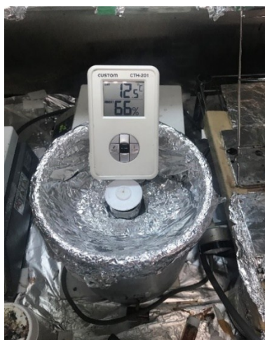
Figure S2. Photo of ambient air with 65% RH when all-inorganic perovskite film was prepared.
