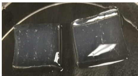
Figure S2. The healed EW hydrogel could be separated into two parts quickly in urea solution.
