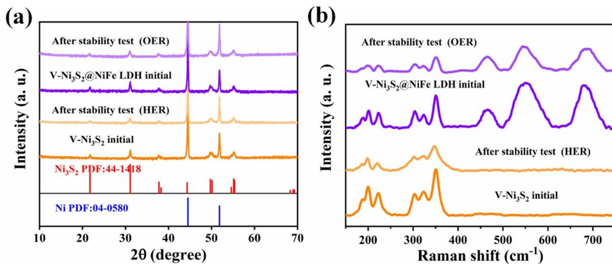
**Fig. S18** (a) XRD patterns, and (b) Raman spectra of V-Ni<sub>3</sub>S<sub>2</sub> and V-Ni<sub>3</sub>S<sub>2</sub>@NiFe LDH before and after overall water splitting stability test.
