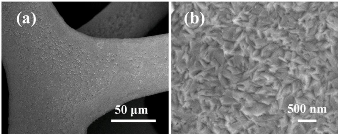
**Fig. S7** SEM images of pure Ni<sub>3</sub>S<sub>2</sub> at low and high magnifications.
