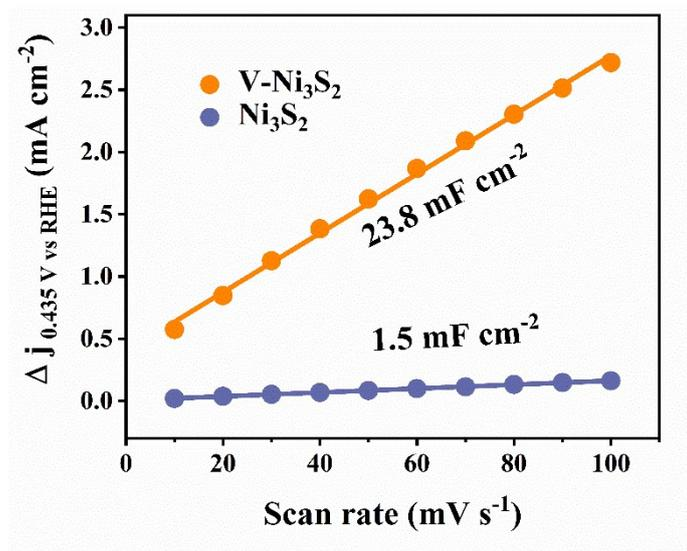
**Fig. S12** Capacitive current density as a function of scan rate for Ni<sub>3</sub>S<sub>2</sub> and V-Ni<sub>3</sub>S<sub>2</sub>.
