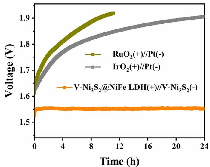
**Fig. S16** Stability tests of overall water splitting at a current density of 10 mA cm<sup>-2</sup> over different electrode pairs.
