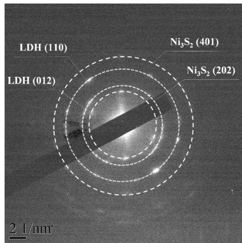
**Fig. S3** Selected area electron diffraction (SAED) of V-Ni<sub>3</sub>S<sub>2</sub>@NiFe LDH.
