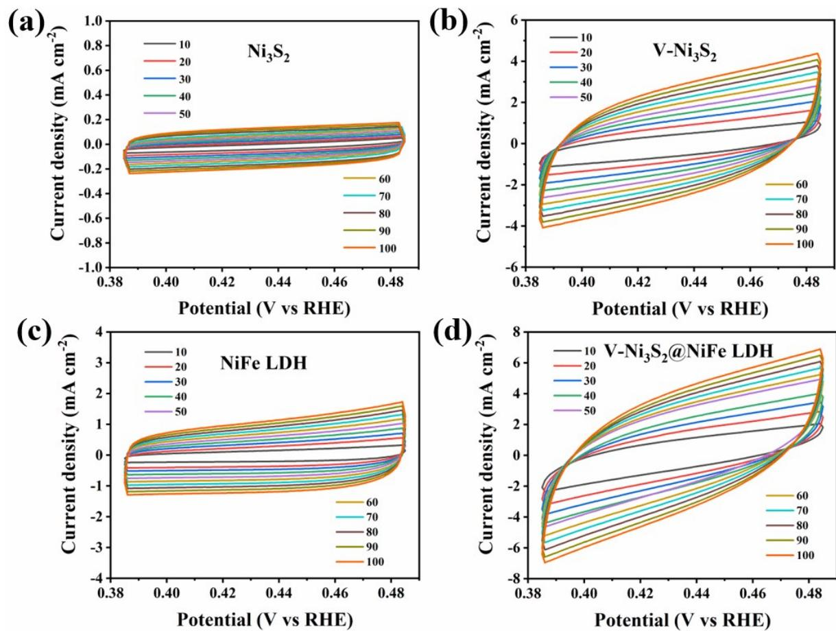
**Fig. S10** Cyclic voltammograms at different scan rates (from 10 mV/s to 100 mV/s with an interval rate of 10 mV/s). (a) Ni<sub>3</sub>S<sub>2</sub>, (b) V-Ni<sub>3</sub>S<sub>2</sub>, and (c) NiFe LDH, and (d) V-Ni<sub>3</sub>S<sub>2</sub>@NiFe LDH.
