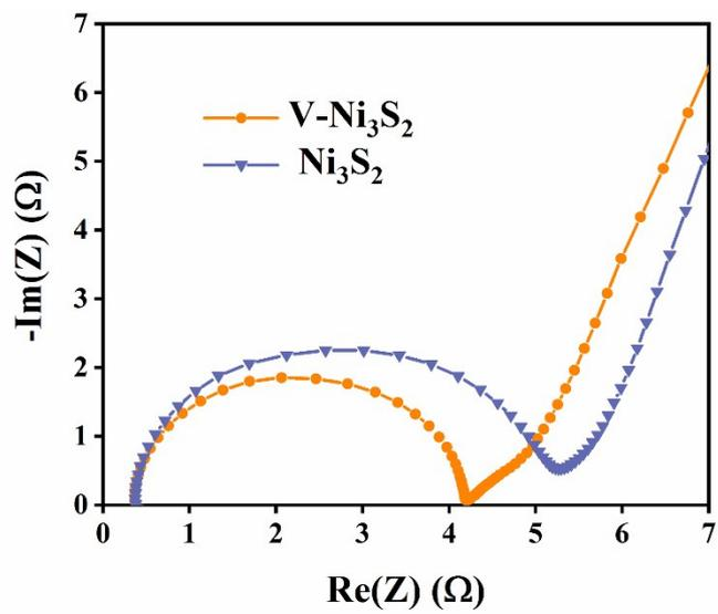
Fig. S13 Nyquist plots of  $\text{Ni}_3\text{S}_2$  and  $\text{V-Ni}_3\text{S}_2$ .
