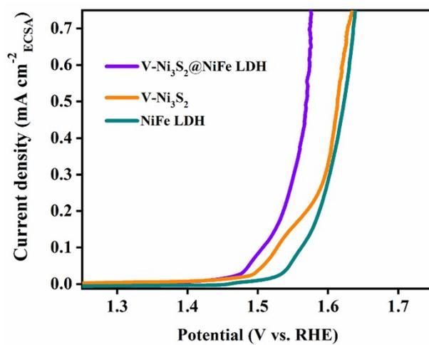
**Fig. S11** Polarization curves with current density normalized by the calculated ECSA for the different catalysts.
