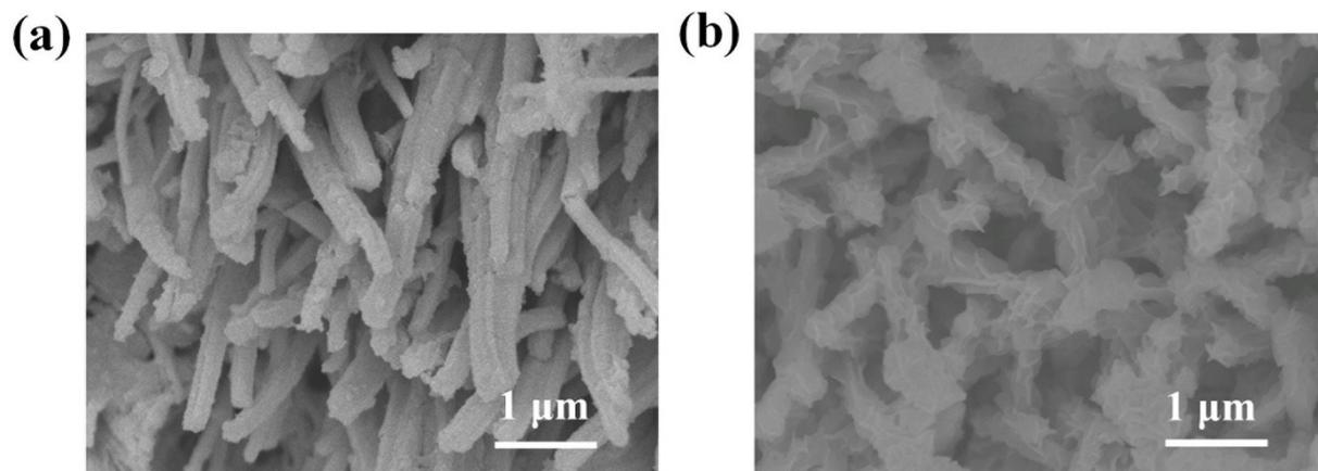
**Fig. S17** SEM images of (a) V-Ni<sub>3</sub>S<sub>2</sub> (cathode for HER) and (b) V-Ni<sub>3</sub>S<sub>2</sub>@NiFe LDH (anode for OER) after overall water splitting stability test.
