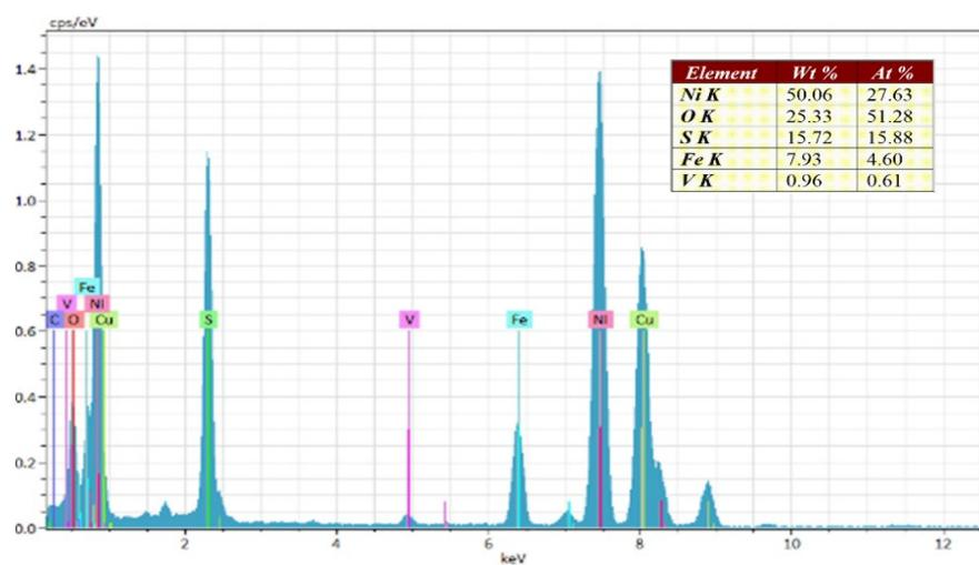
**Fig. S5** Energy dispersive X-ray (EDX) spectrum of V-Ni<sub>3</sub>S<sub>2</sub>@NiFe LDH.
