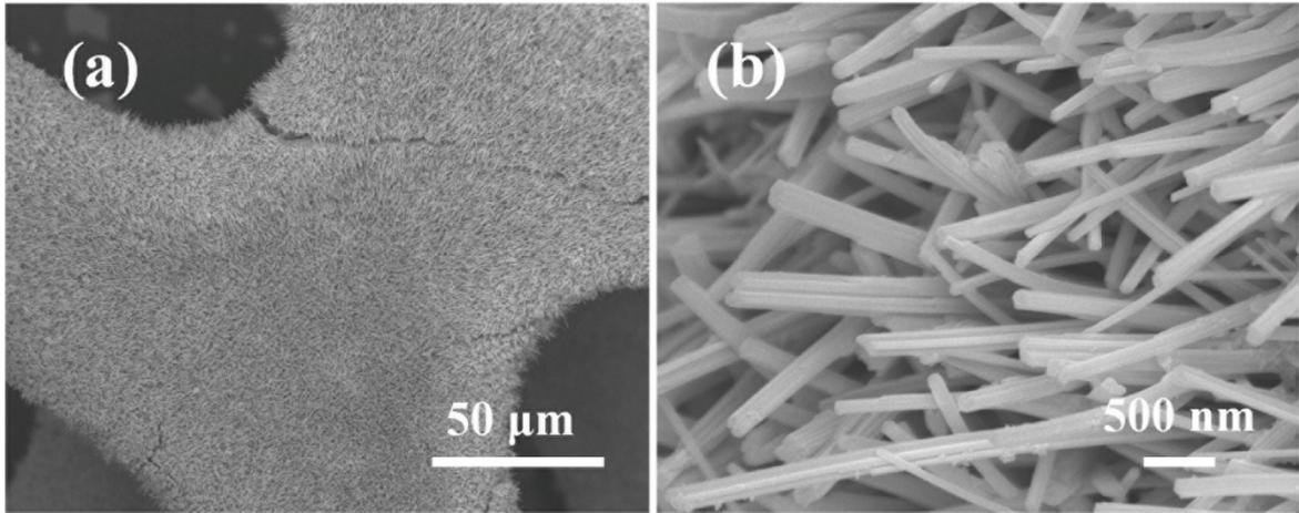
**Fig. S2** SEM images of V-Ni<sub>3</sub>S<sub>2</sub> nanorod arrays at low and high magnifications.
