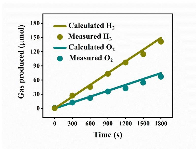
**Fig. S14** Experimental and theoretical calculated amounts of H<sub>2</sub> and O<sub>2</sub> by the overall water splitting of V-Ni<sub>3</sub>S<sub>2</sub>@NiFe LDH(+)//V-Ni<sub>3</sub>S<sub>2</sub>(-) at a current density of 50 mA cm<sup>-2</sup>.
