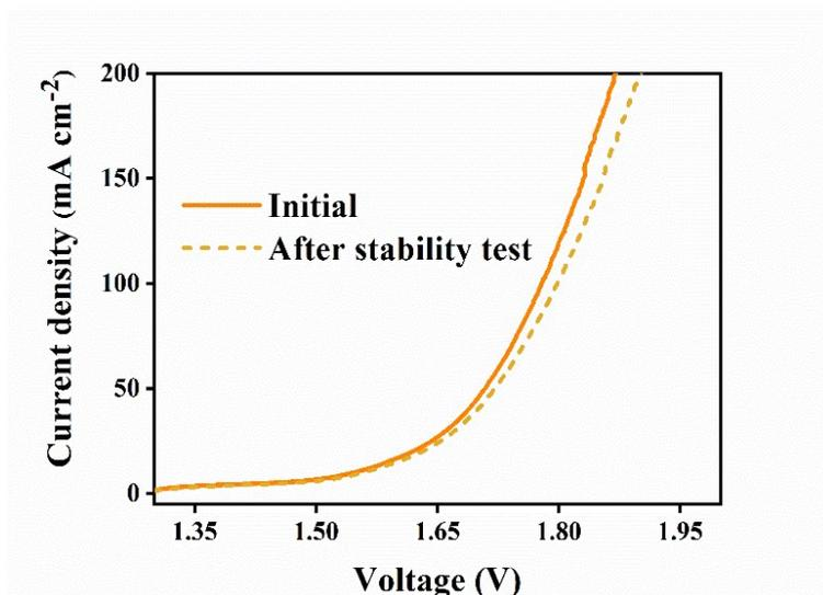
**Fig. S15** Overall water splitting polarization curves before and after overall water splitting stability test.
