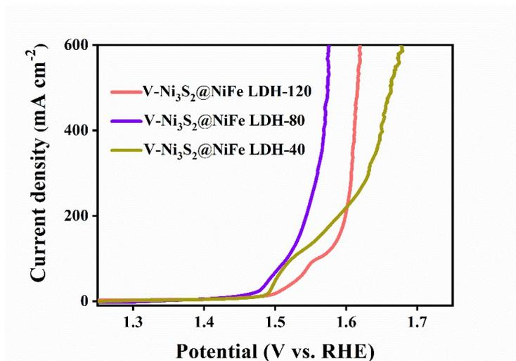
**Fig. S9** OER polarization curves of V-Ni<sub>3</sub>S<sub>2</sub>@NiFe LDH-40, V-Ni<sub>3</sub>S<sub>2</sub>@NiFe LDH-80, and V-Ni<sub>3</sub>S<sub>2</sub>@NiFe LDH-120.
