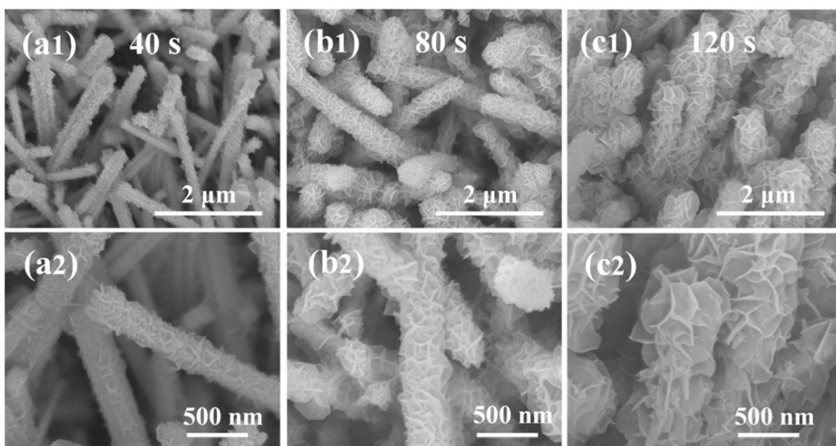
**Fig. S8** SEM images of (a1 and a2) V-Ni<sub>3</sub>S<sub>2</sub>@NiFe LDH-40, (b1 and b2) V-Ni<sub>3</sub>S<sub>2</sub>@NiFe LDH-80, and (c1 and c2) V-Ni<sub>3</sub>S<sub>2</sub>@NiFe LDH-120 at low and high magnifications.
