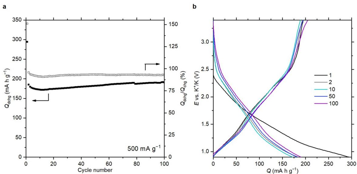
**Figure S13.** Cycling performance of **P1** in PIBs at 500 mA g<sup>-1</sup>: (a) the dependence of the discharge capacity and the coulombic efficiency on the cycle number; (b) charge-discharge curves for different cycle numbers.
