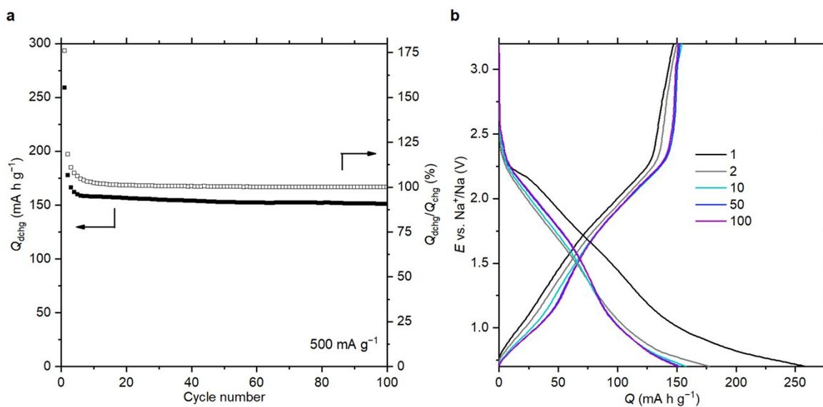
**Figure S12.** Cycling performance of **P1** in SIBs at 500 mA g<sup>-1</sup>: (a) the dependence of the discharge capacity and the coulombic efficiency on the cycle number; (b) charge-discharge curves for different cycle numbers.
