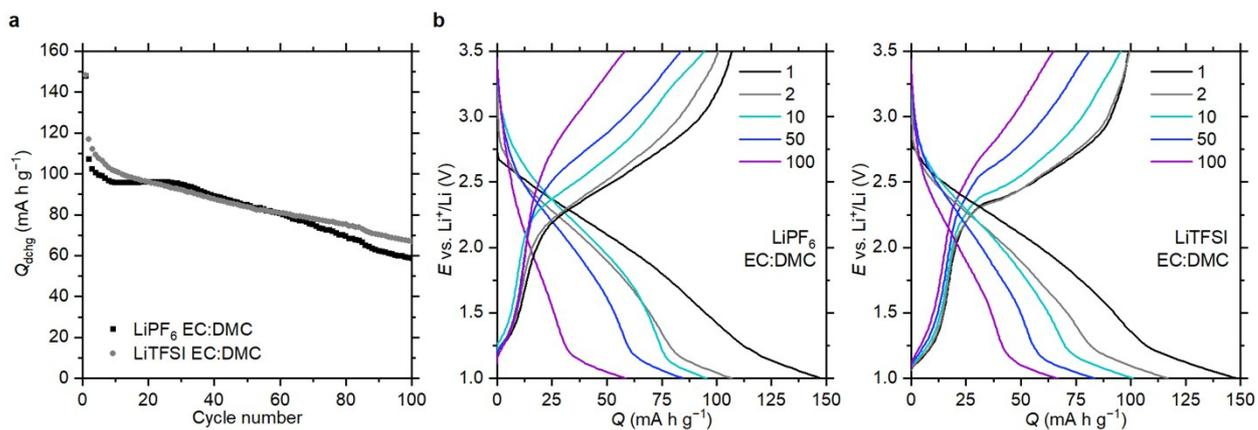
**Figure S7.** Cycle performance of **P1** in LIBs with 1M  $\text{LiPF}_6$  or 1M  $\text{LiTFSI}$  in EC:DMC: (a) cycling stability at  $500 \text{ mA g}^{-1}$ ; (b) charge-discharge curves at  $500 \text{ mA g}^{-1}$  for different cycle numbers.
