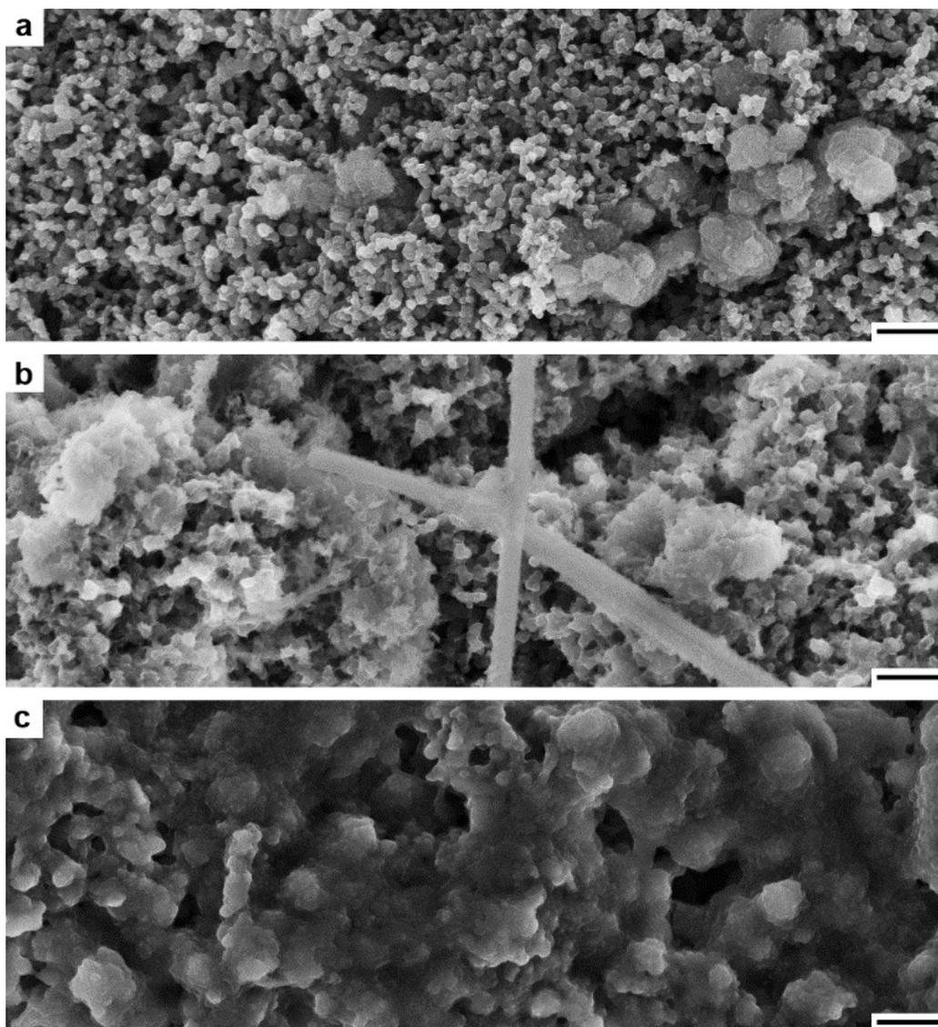
**Figure S8.** SEM images of the electrodes (a) before cell assembling and after 100 cycles at  $500 \text{ mA g}^{-1}$  in (b) 1M LiTFSI DME, (c) 1M LiTFSI EC:DMC. Scale bars: 400 nm. Two filaments observed in (b) are fibers from the separator.
