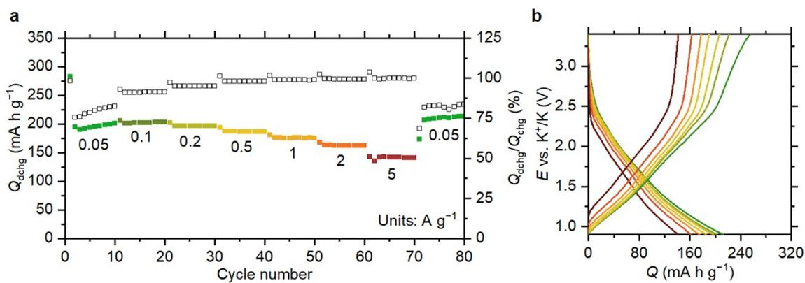
**Figure S20.** Electrochemical behavior of P1 in potassium-ion batteries for an electrode with the mass ratio of P1:Super P:PVdF = 6:3:1. (a) discharge capacities and charge/discharge capacity ratios at different current rates; (b) charge-discharge curves for each 10th cycle represented in (a) except for the cycle 10.
