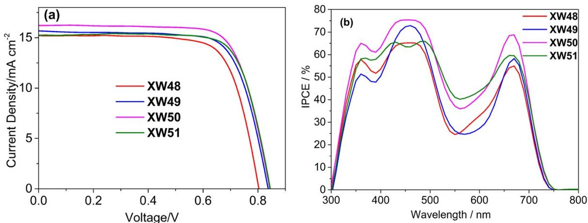
**Figure S5.** (a) J-V curves and (b) IPCE action spectra of DSSCs based on **XW48~XW51** using a  $\text{Co}^{3+}/\text{Co}^{2+}$  electrolyte.
