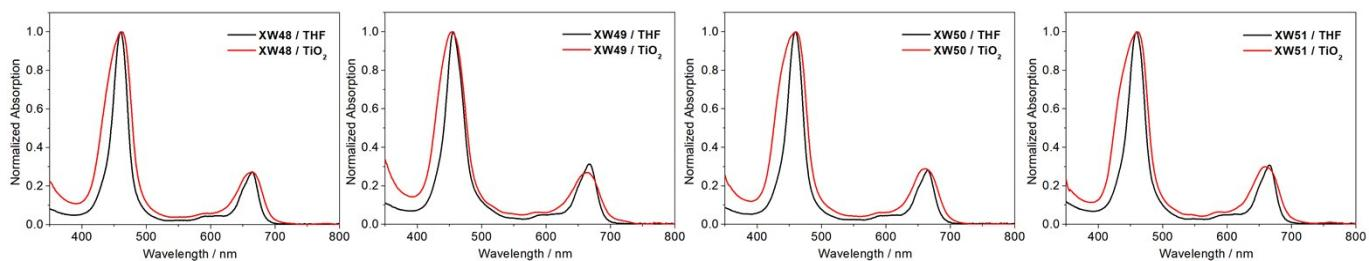
**Figure S2.** Normalized UV-visible spectra of porphyrins **XW48~XW51** in THF and on the TiO<sub>2</sub> films (3 μm).
