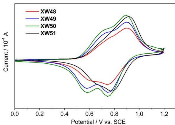
**Figure S3.** Cyclic voltammetry curves of the **XW48~XW51** adsorbed to a nanocrystalline TiO<sub>2</sub> film deposited on the conducting FTO glass.
