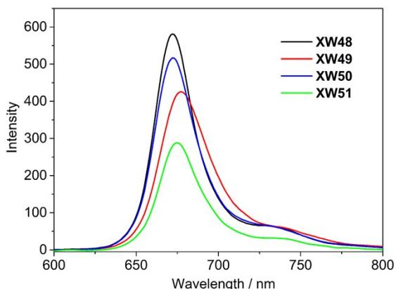
**Figure S1.** Emission spectra of **XW48~XW51** in THF. The spectra were used to calculate the wavelength at the intersection ( $\lambda_{\text{inter}}$ ) of normalized absorption and emission spectra, and the corresponding  $E_{0-0}$  values. Excitation wavelengths: 460 nm (**XW48**), 456 nm (**XW49**), and 455 nm (**XW50**) and 460 nm (**XW51**).
