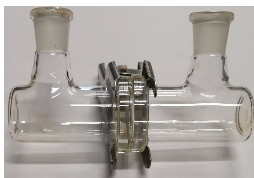
Fig. S3. Homemade diffusion cell used for the preparation of COF-JLU2 membranes.
