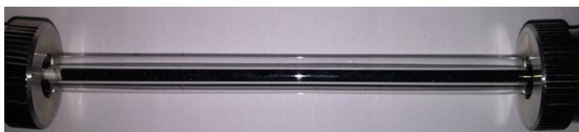
**Fig. S24.** The photograph of the packing column used for the breakthrough experiments.
