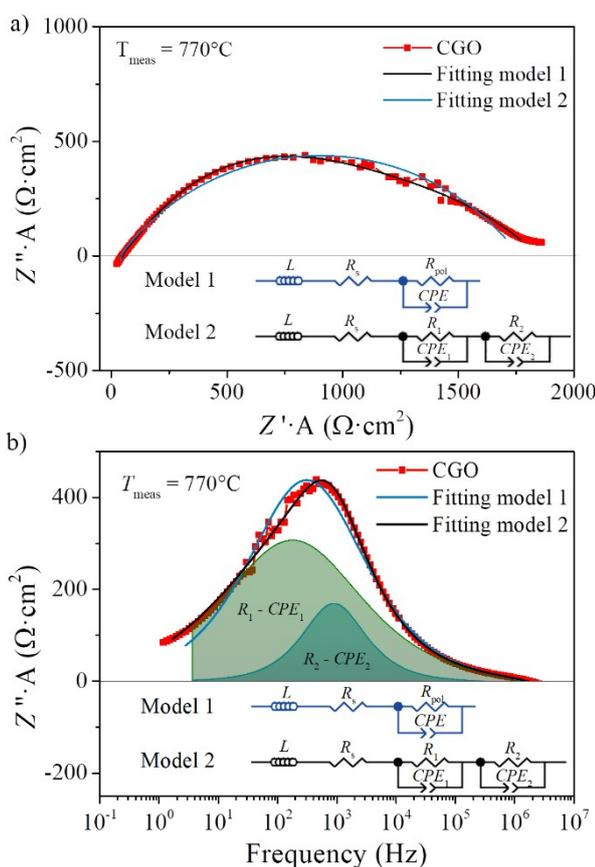
**Figure S1.** S1a) Nyquist plot ( $T = 770^\circ\text{C}$ ) of a YSZ/mesoporous CGO test cell is shown with the equivalent circuits used for the fitting. S1b) Bode plot with the two different fitting models. The single  $R_i - CPE_i$  are highlighted.
