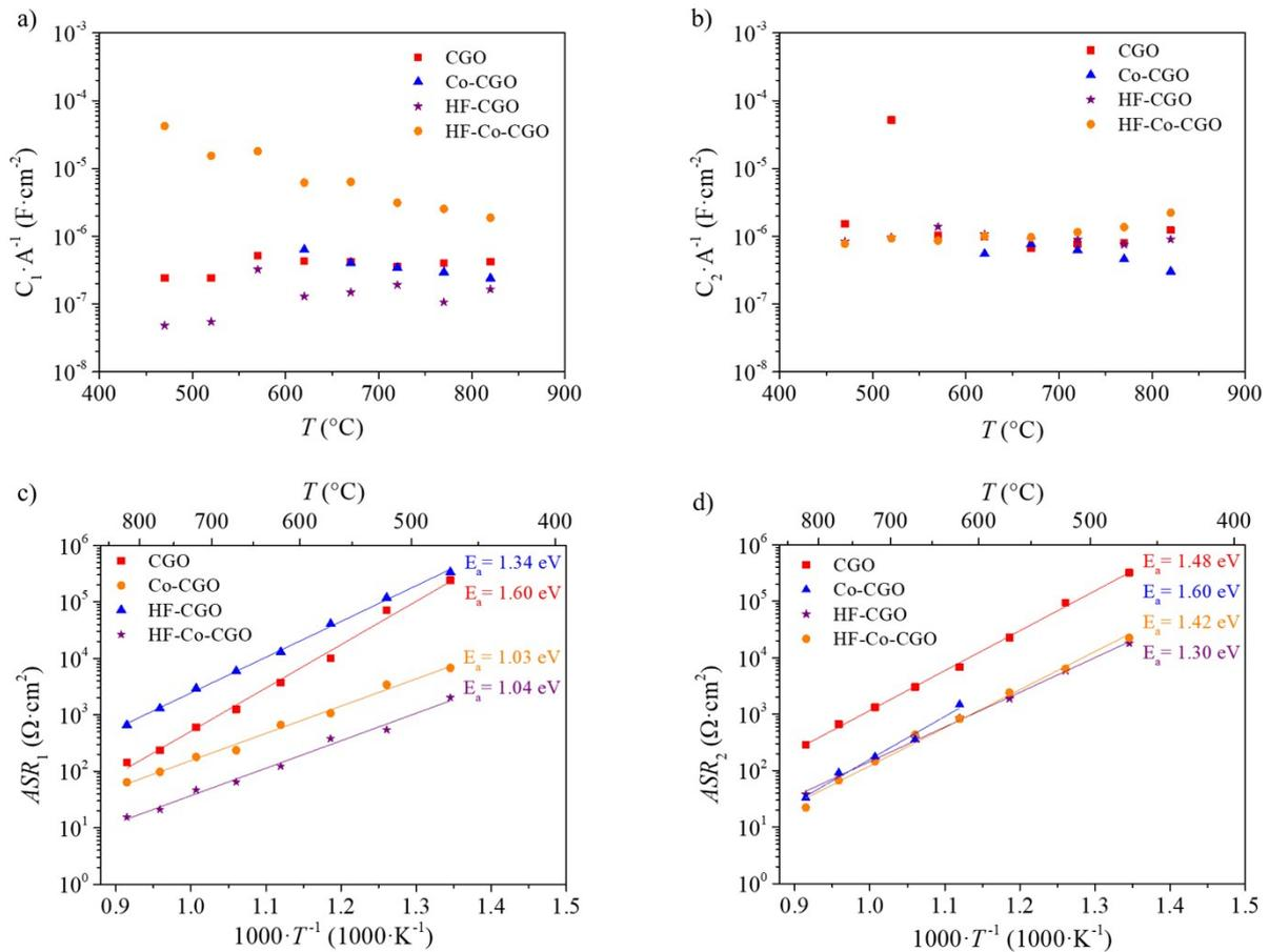
**Figure S2.** Resulting EIS fitting parameters for symmetric CGO/YSZ cells as a function of temperature. The high (low) frequency arc true capacitance and area specific resistance are reported in panels a (b) and c (d), respectively.
